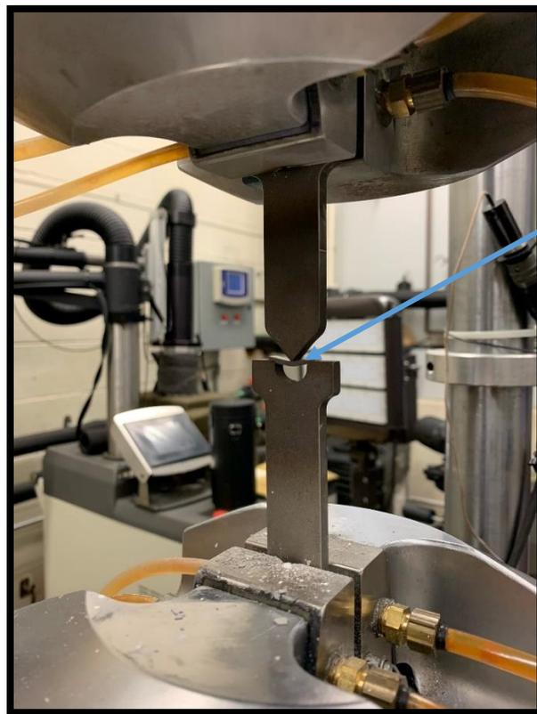
Three Point Bend Test Specimen
