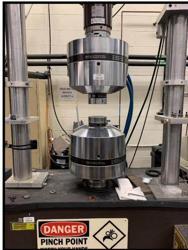
**Figure 14. MTS 110 kip Load Frame used for Compression Tests**
