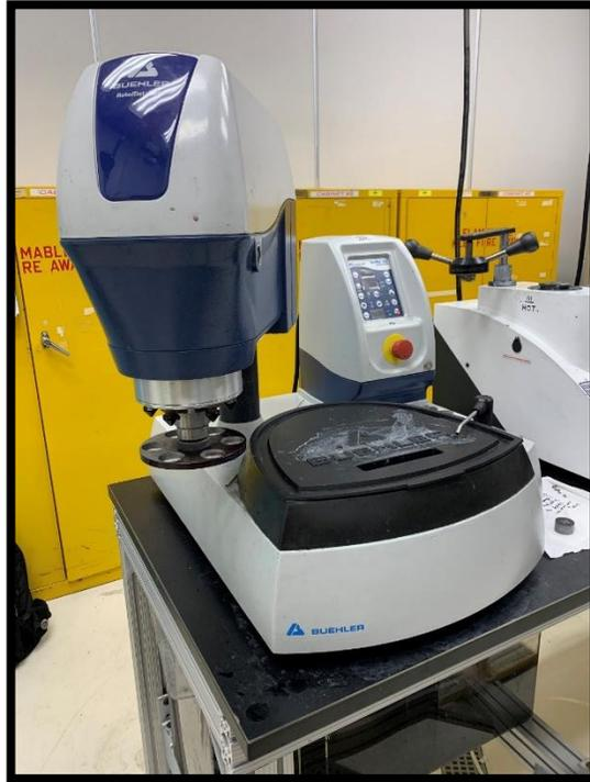
**Figure 9. Buehler Ecomet 300 Grinding and Polishing Machine**
