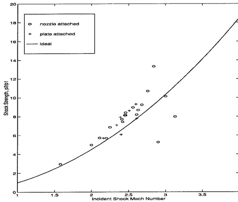
Figure 9. Incident Shock Strength Versus Mach Number
