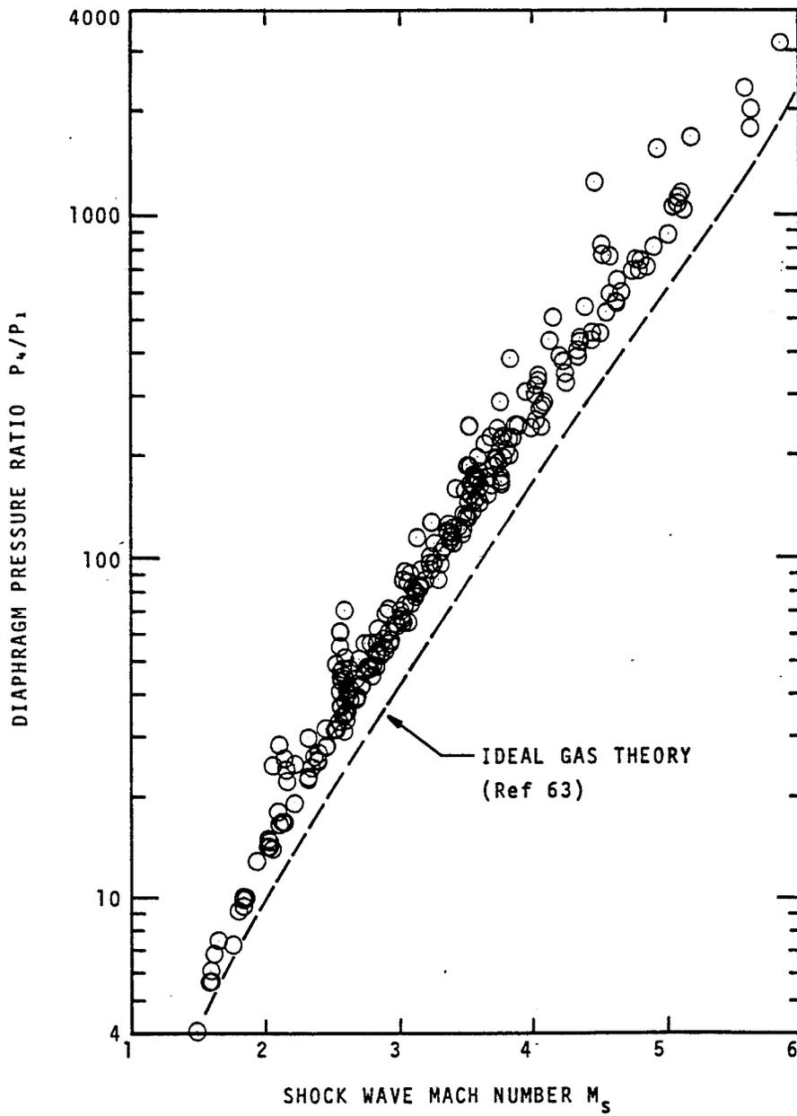
Figure 14. Uda's Figure 22, Diaphragm Pressure Ratio Experimental Data Points Compared to Ideal Gas Theory Curve for the He/Air System
