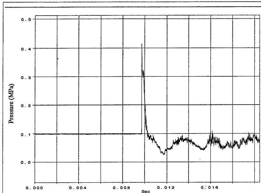
Figure 6. Pressure History at the Nozzle Exit for an Unstarted Nozzle
