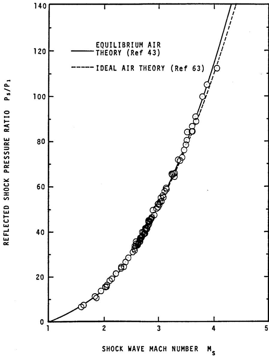
Figure 15. Uda's Figure 23, Reflected Shock Pressure Ratio Experimental Data Points Compared to Equilibrium and Ideal Air Theory Curves
