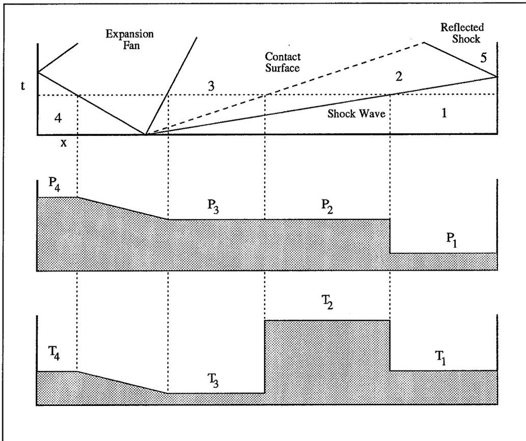
Figure 1.  $x$ - $t$  Diagram and Pressure and Temperature Plots for the Shock Tube Prior to Shock Wave Reflection
