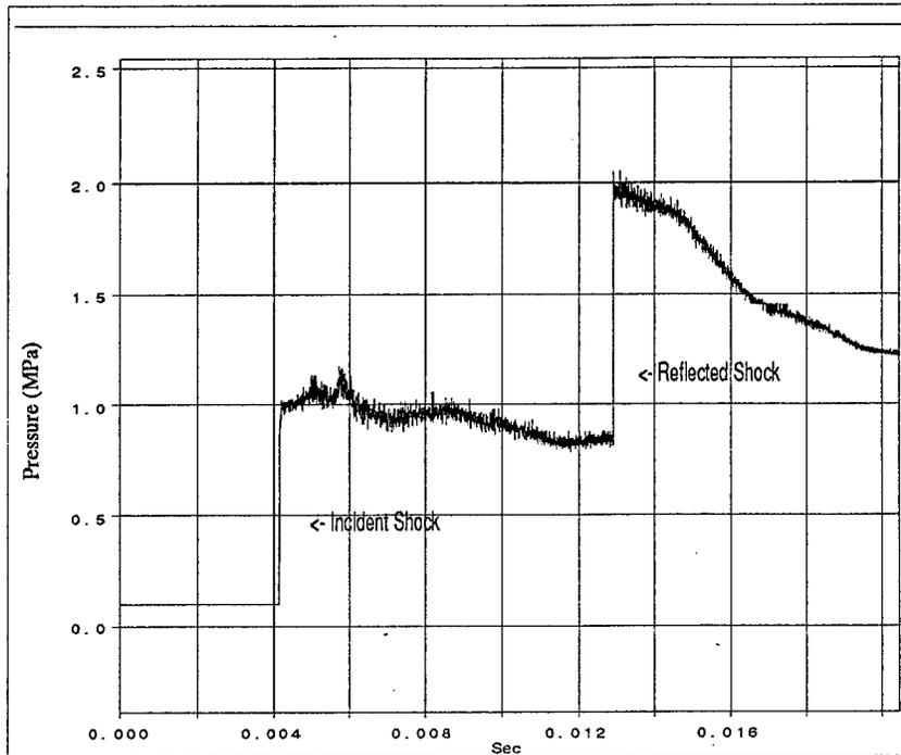
Figure 17. Pressure History at the Location of Pressure Transducer B Upstream of the Nozzle
