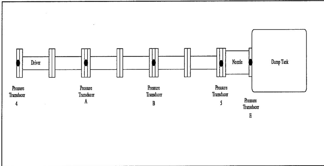
Figure 3. Pressure Transducer Locations
