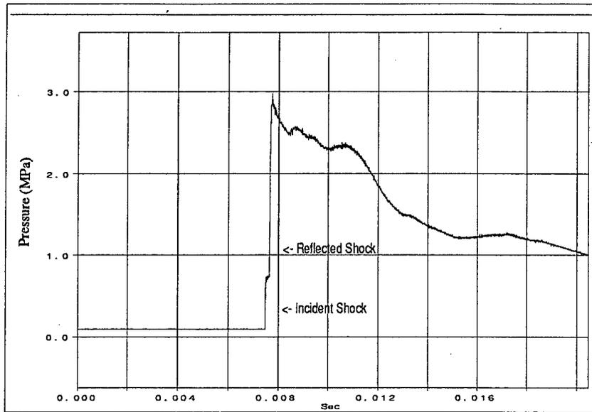
Figure 4. Pressure History at the Nozzle Entrance (Pressure Transducer 5)
