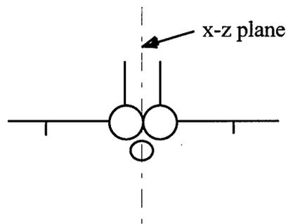
Figure 2-3.  $x$ - $z$  plane of symmetry.
