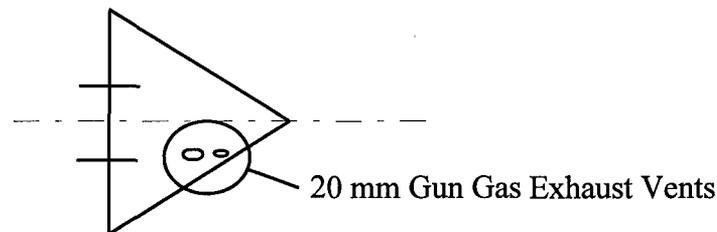
Figure 2-4. 20 mm gun gas exhaust vent location.
