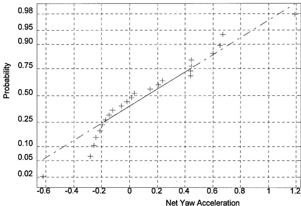
Figure 4.2. Normal probability plot of net yaw acceleration data for example F-15B.
