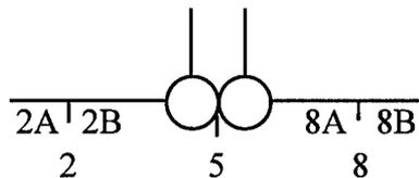
Figure 2-1. F-15 external Station locations, aft view.
