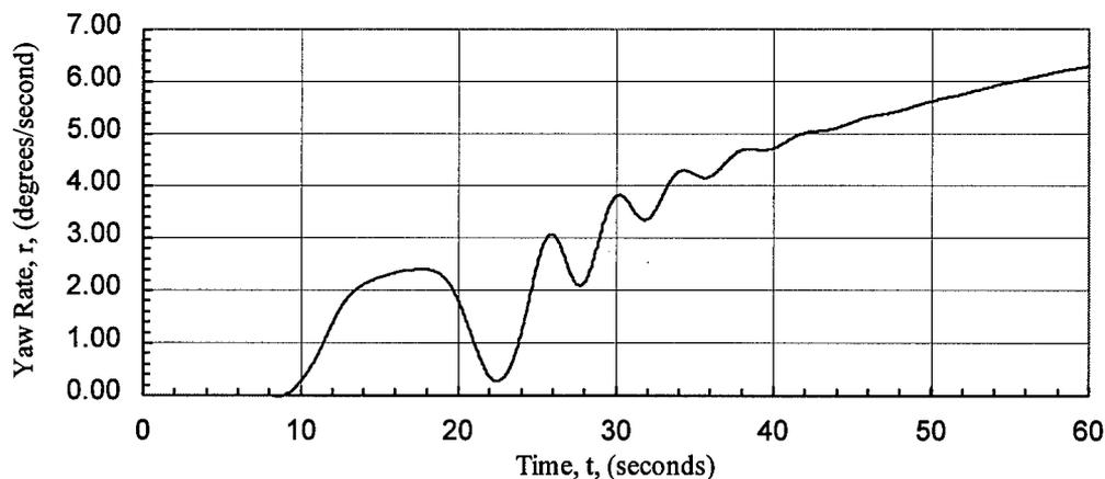
Figure 3-2. Baseline F-15A simulator yaw rate prediction at 15,000 feet (4,572 meters) PA, with symmetric stabilators.
