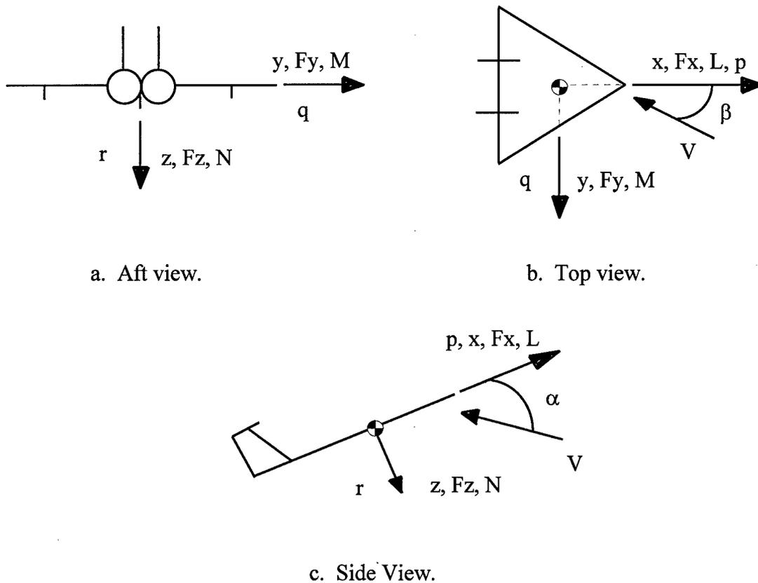
Figure 2-2. Right-handed coordinate System.
