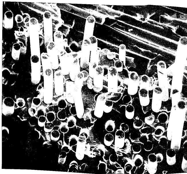
Figure 96. Isothermal Fatigue 566°C: 133 MPa, Fiber Pull-Out, 550x
