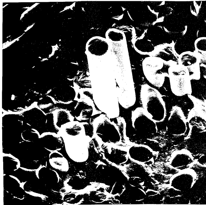
Figure 90. Out-of-Phase TMF: 145 MPa, Fiber Condition, 600x
