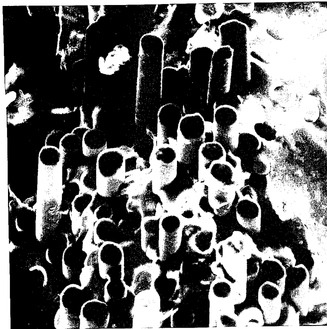
Figure 104. 1093°C Isothermal Fatigue: 100 MPa, Fiber Condition, 550x
