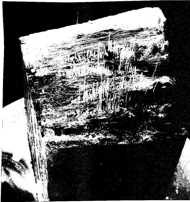
Figure 95. Isothermal Fatigue 566°C: 160 MPa, Fracture Surface, 11x
