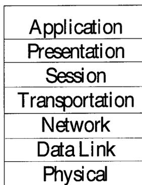
Figure C.1 Open Systems Interconnection Reference Model Architecture(34)
