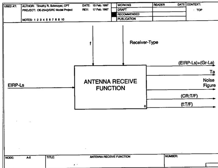
Figure 3.6 IDEF0 OE-254/GRC (A-0) Diagram with Constraint
