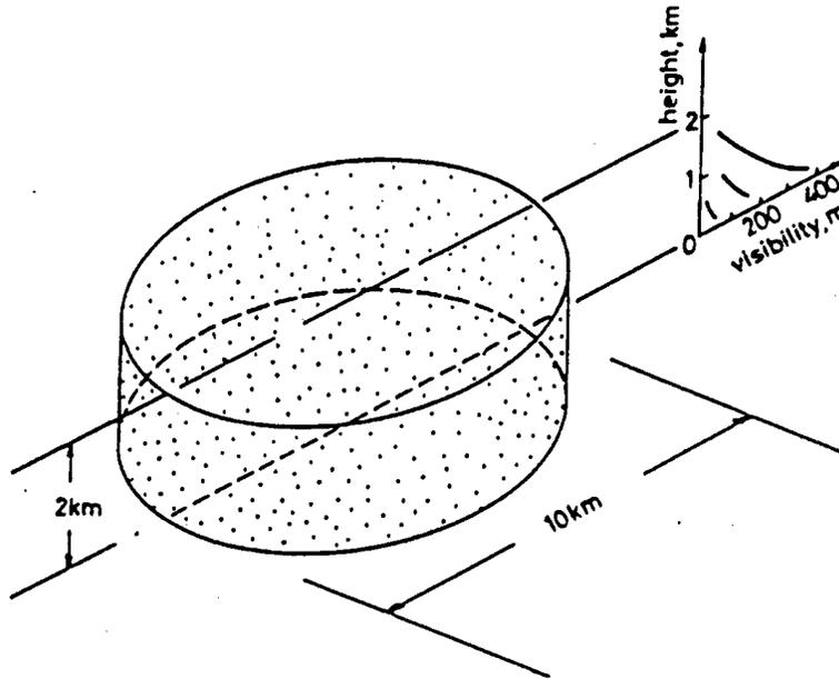
Figure C.8 Schematic of the Dust Cell Model(14)
