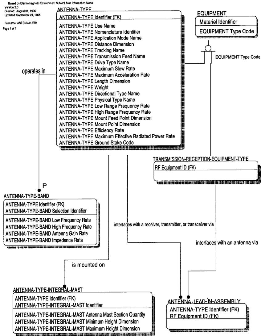
Figure 3.2 IDEF1X Antenna ER Diagram
