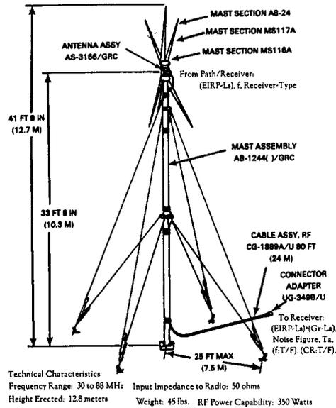
Figure 3.8 System Architecture of OE-254()/GRC Antenna System
