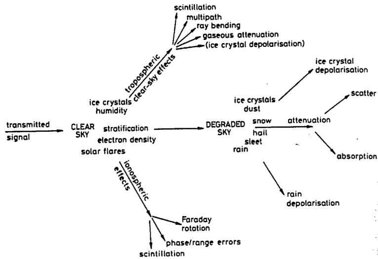
Figure C.3 Schematic Presentation of Propagation Impairment Mechanisms(14)
