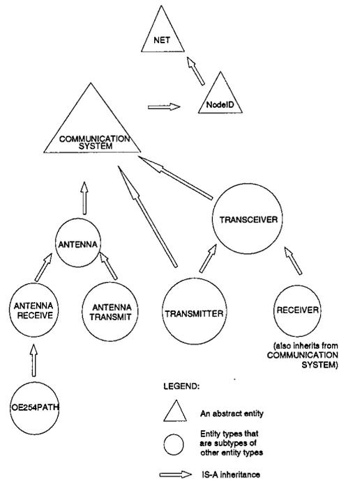
Figure 3.9 Semantic Model for a Communication Net.
