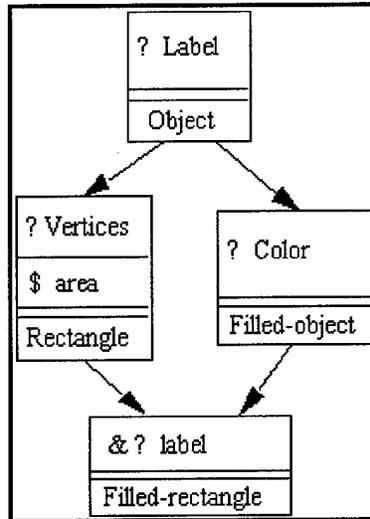
Figure 2. Inheritance Diagram
