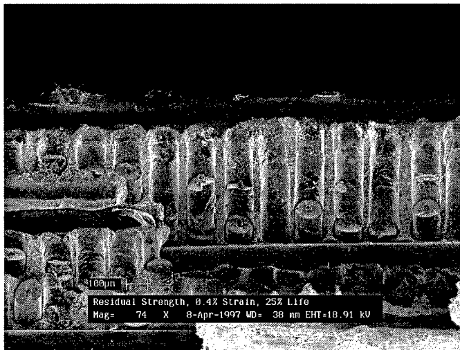
Figure 40. Fiber Failure, 0.4% Maximum Strain, 25% Expected Life
