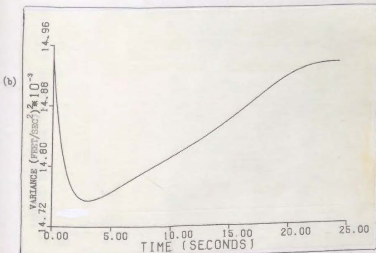
Fig. 5.12(a),(b) Smoother estimate and variance of accelerometer error after two iterations.
