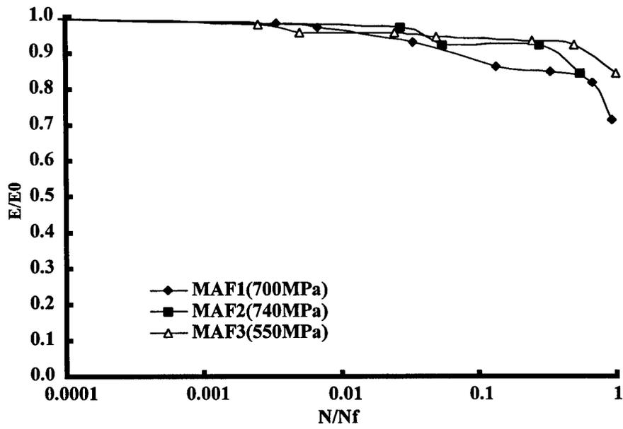
Figure 57. Normalized Modulus vs Normalized Cycles - MAF Specimens
