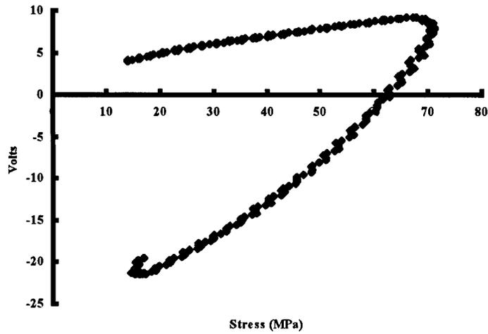
Figure 69. Stress vs Voltage Loop - Cycle 1,  $\sigma = 75\text{MPa}$  (Before Repoling)
