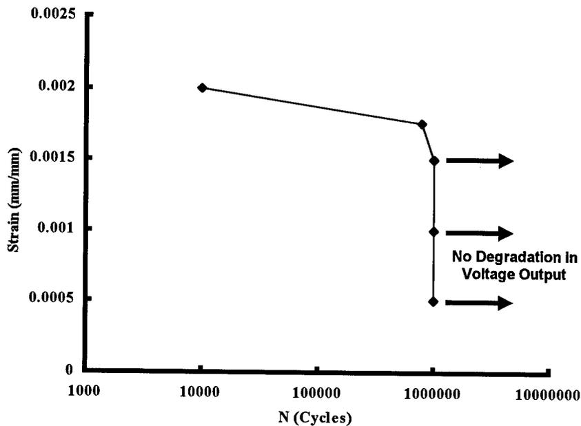
Figure 19. Strain vs Cycles to Failure - Out-of-Phase Condition
