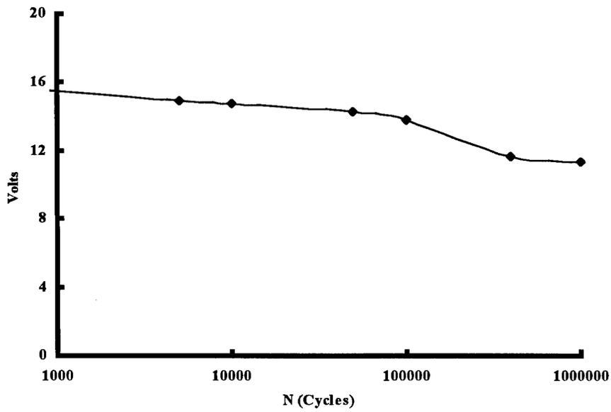
Figure 29. Voltage Output vs Cycles Curve,  $\sigma = 75 MPa$
