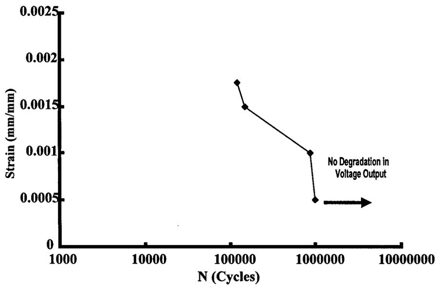
Figure 27. Strain vs Cycles to Failure - In-Phase Condition
