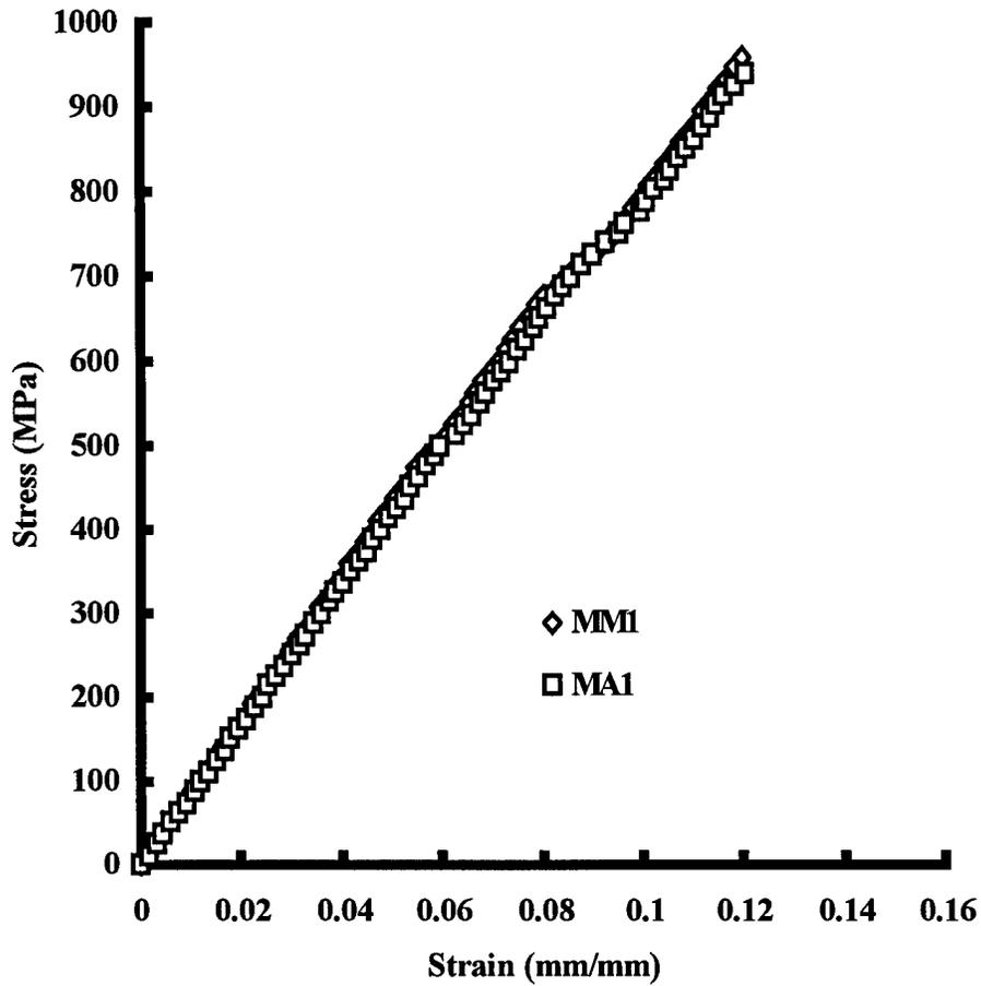
Figure 44. Stress-Strain Curves for Specimens MM1 and MA1
