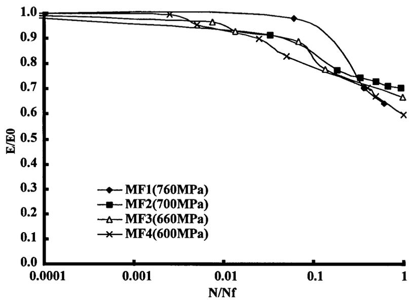
Figure 55. Normalized Modulus vs Normalized Cycles - MF Specimens
