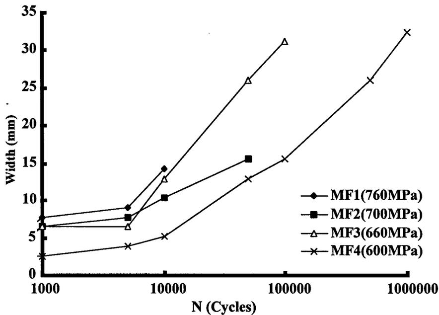
Figure 62. Width of Delamination vs Cycles - MF Specimens
