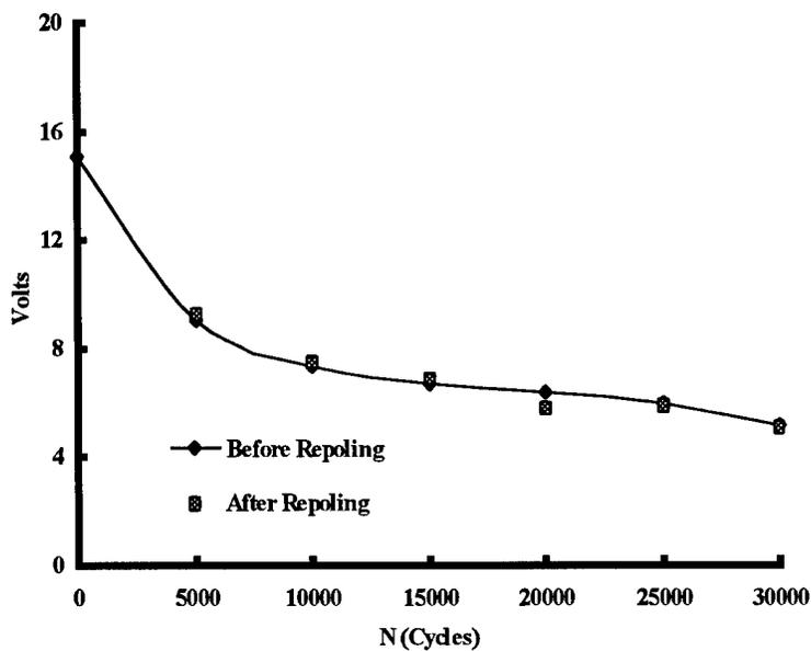
Figure 17. Voltage Output vs Cycles Curve,  $\sigma = 100 MPa$  and  $E = 10V$  to  $100V$
