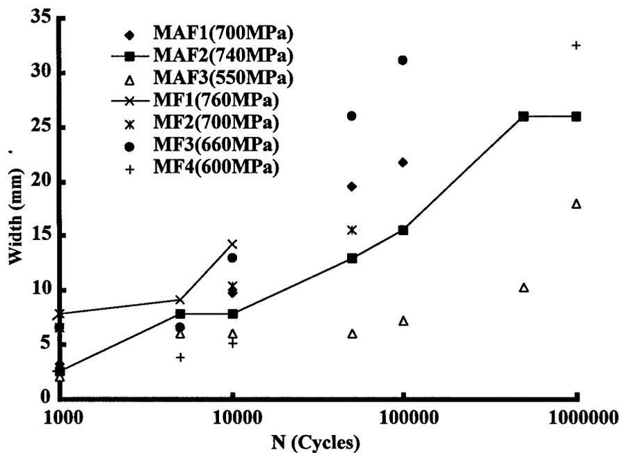
Figure 64. Width of Delamination vs Cycles - All Specimens
