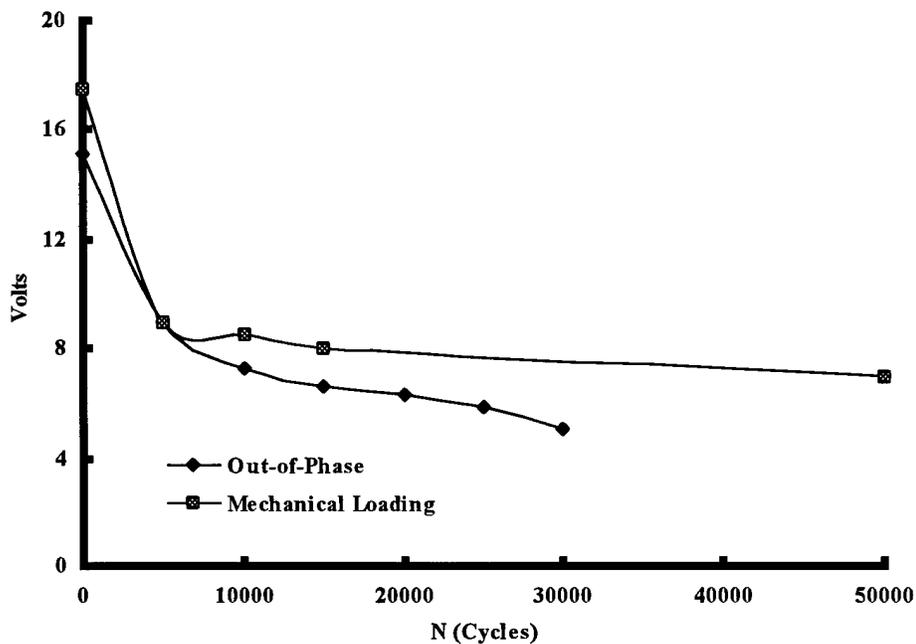
Figure 38. Voltage Output vs Cycles Curves - Out-of-Phase and Low Stress Conditions,  $\sigma = 100MPa$
