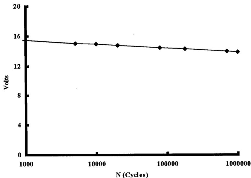
Figure 20. Voltage Output vs Cycles Curve,  $\sigma = 25MPa$  and  $E = -10V$  to  $-100V$
