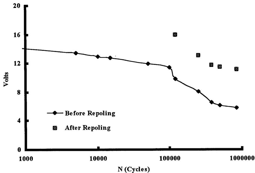
Figure 21. Voltage Output vs Cycles Curve,  $\sigma = 50 MPa$  and  $E = -10V$  to  $-100V$
