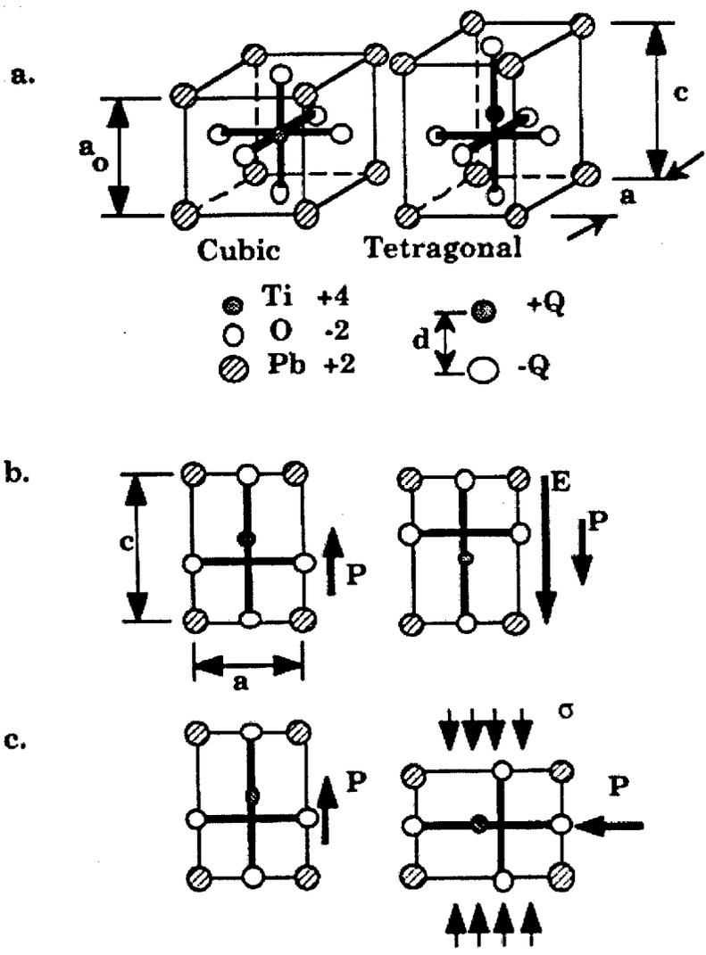
Figure 3. Crystal Structure of Piezoelectric Material
