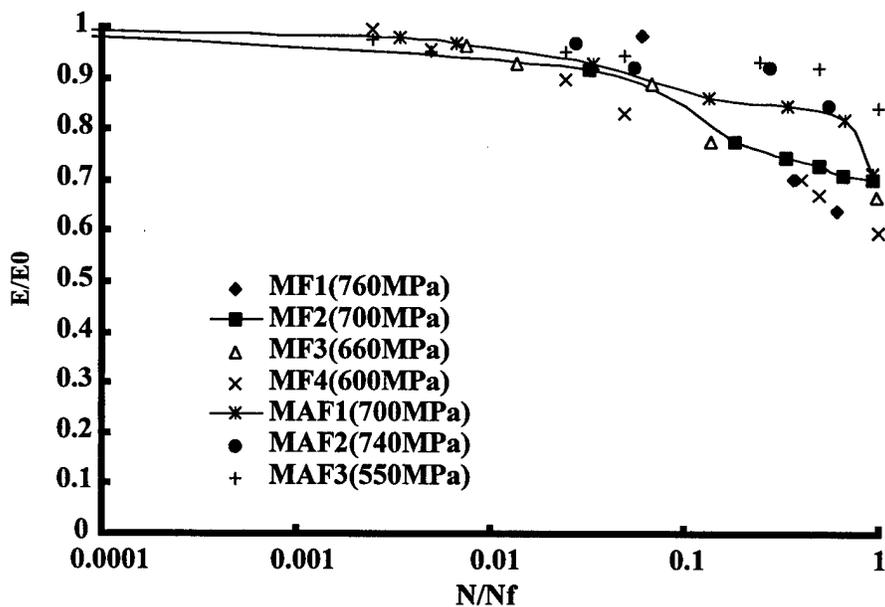
Figure 58. Normalized Modulus vs Normalized Cycles - All Specimens
