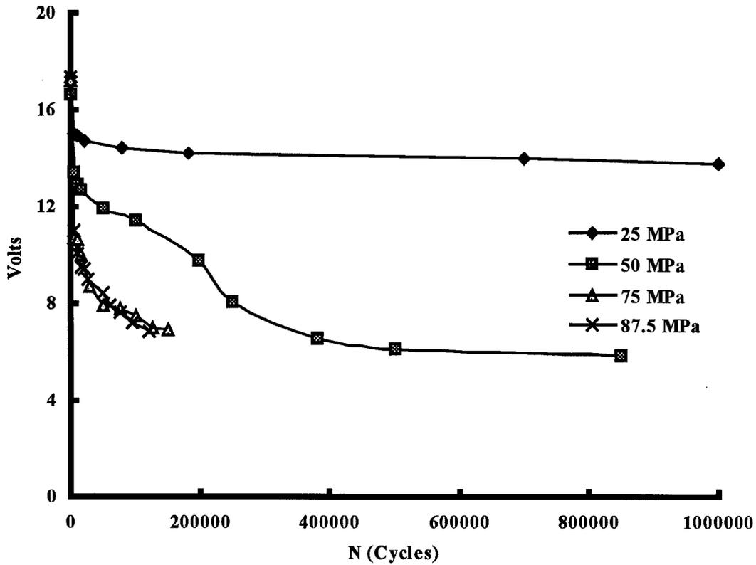
Figure 26. Voltage Output vs Cycles Curves - In-Phase Condition
