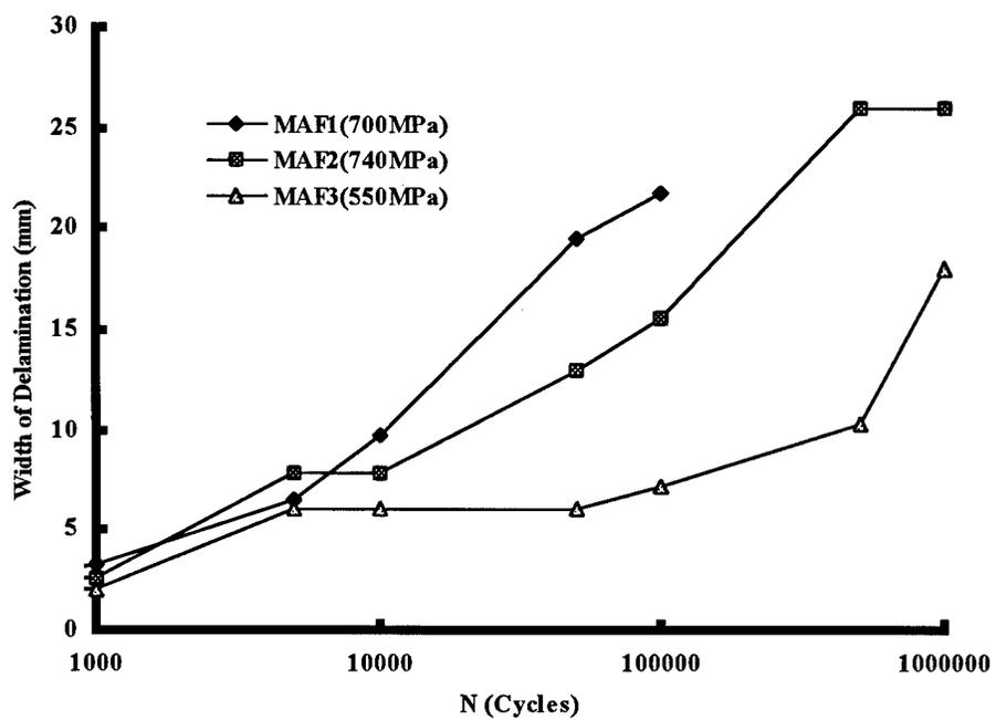
Figure 63. Width of Delamination vs Cycles - MAF Specimens
