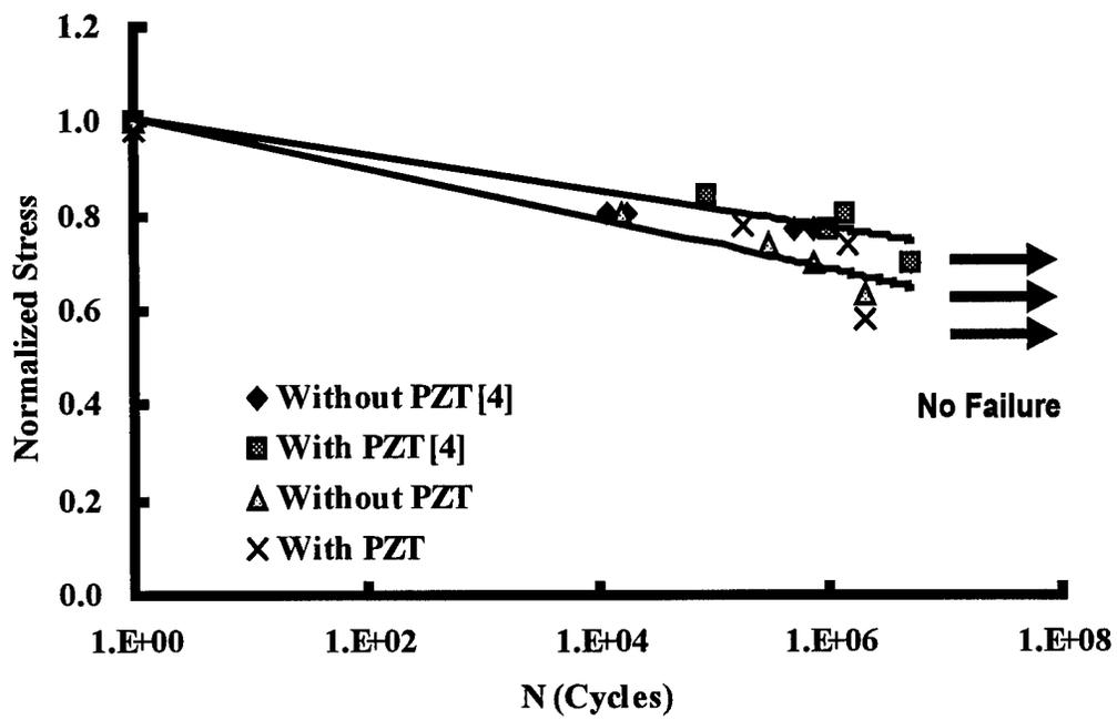
Figure 68. Normalized Stress vs Cycles - Current Work and Coleman [4]
