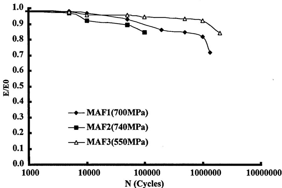
Figure 56. Normalized Modulus vs Cycles - MAF Specimens
