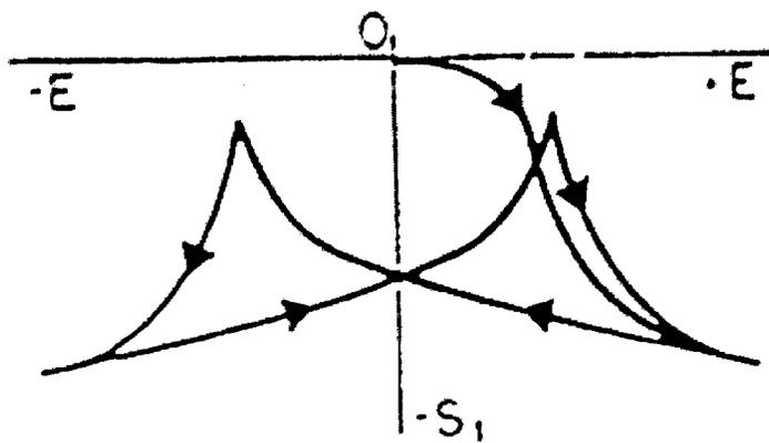
Figure 4. Polarization vs Electric Field Hysteresis Loop
