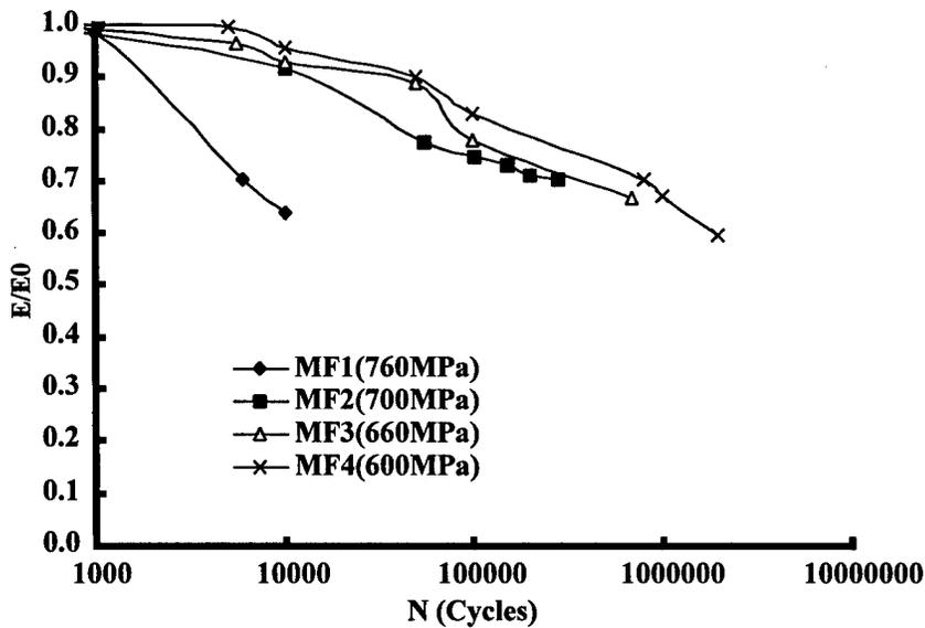
Figure 54. Normalized Modulus vs Cycles - MF Specimens
