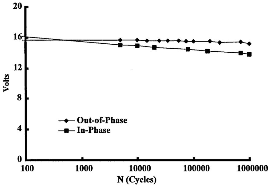
Figure 34. Voltage Output vs Cycles Curves - Out-of-Phase and In-Phase Conditions,  $\sigma = 25MPa$
