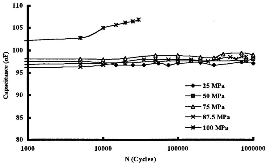
Figure 40. Capacitance vs Cycles Curves - Out-of-Phase Condition
