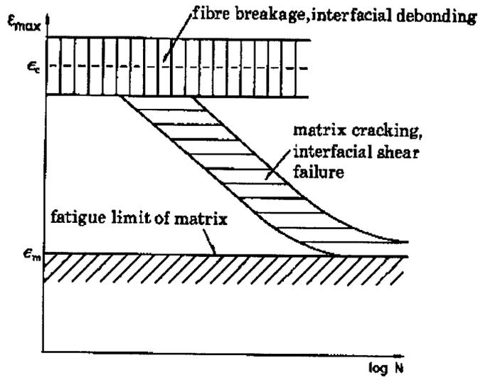
Figure 1. Fatigue-life diagram for Unidirectional Composites [20]
