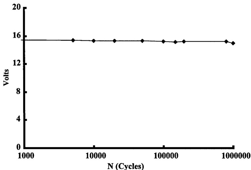
Figure 13. Voltage Output vs Cycles Curve,  $\sigma = 50\text{ MPa}$  and  $E = 10\text{ V}$  to  $100\text{ V}$
