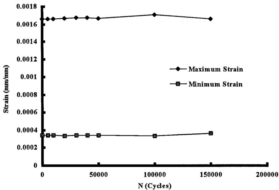
Figure 43. Strain vs Cycles Curve - Specimen EAF3
