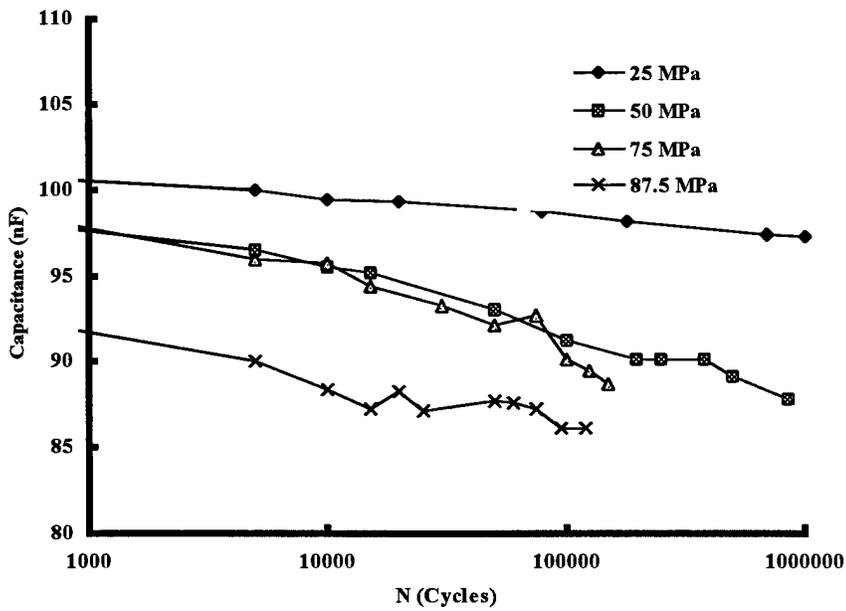
Figure 41. Capacitance vs Cycles Curves - In-Phase Condition
