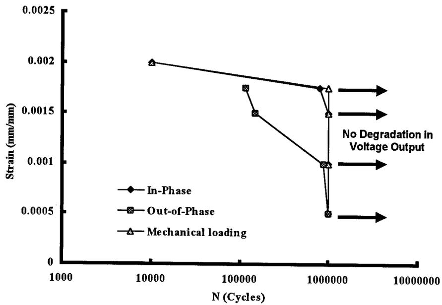
Figure 39. Strain vs Cycles to Failure - All Conditions
