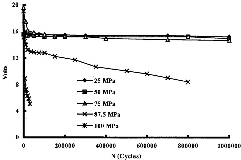
Figure 18. Voltage Output vs Cycles Curves - Out-of-Phase Condition
