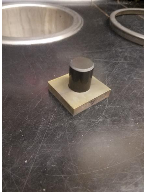
Figure 6 Sample blank with metallographic mount handle for grinding
