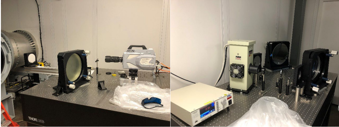
Figure 21: Physical Schlieren set-up for experiments
