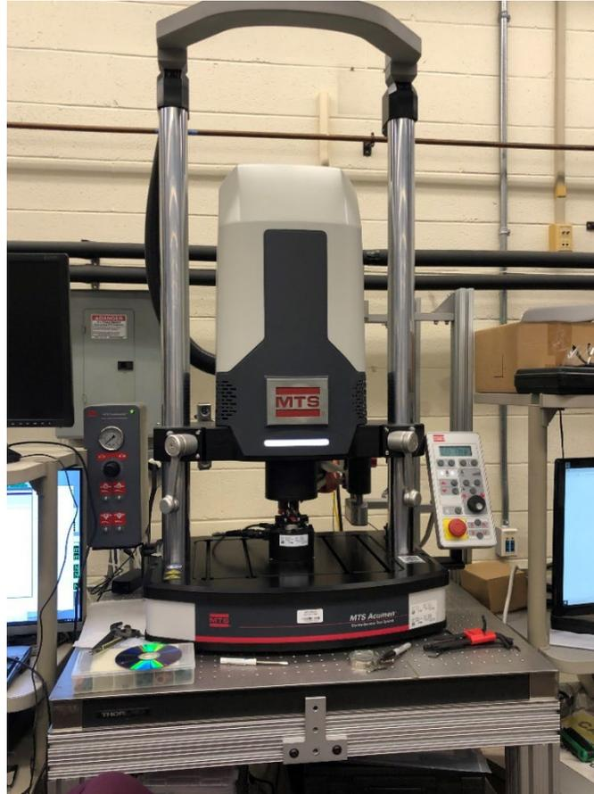
**Figure 3.6 MTS Acumen Electromechanical Test System [36]**
