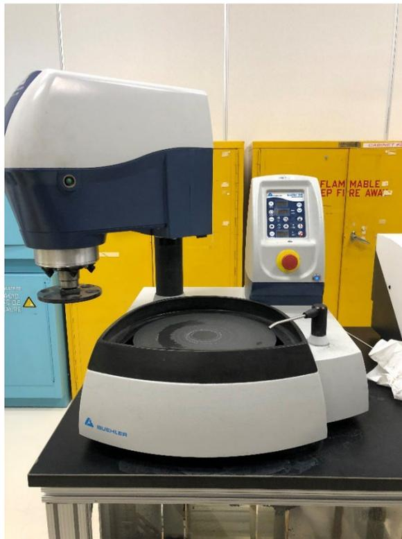
**Figure 3.3 Buehler Ecomet 300 Grinder and Polisher [34]**
