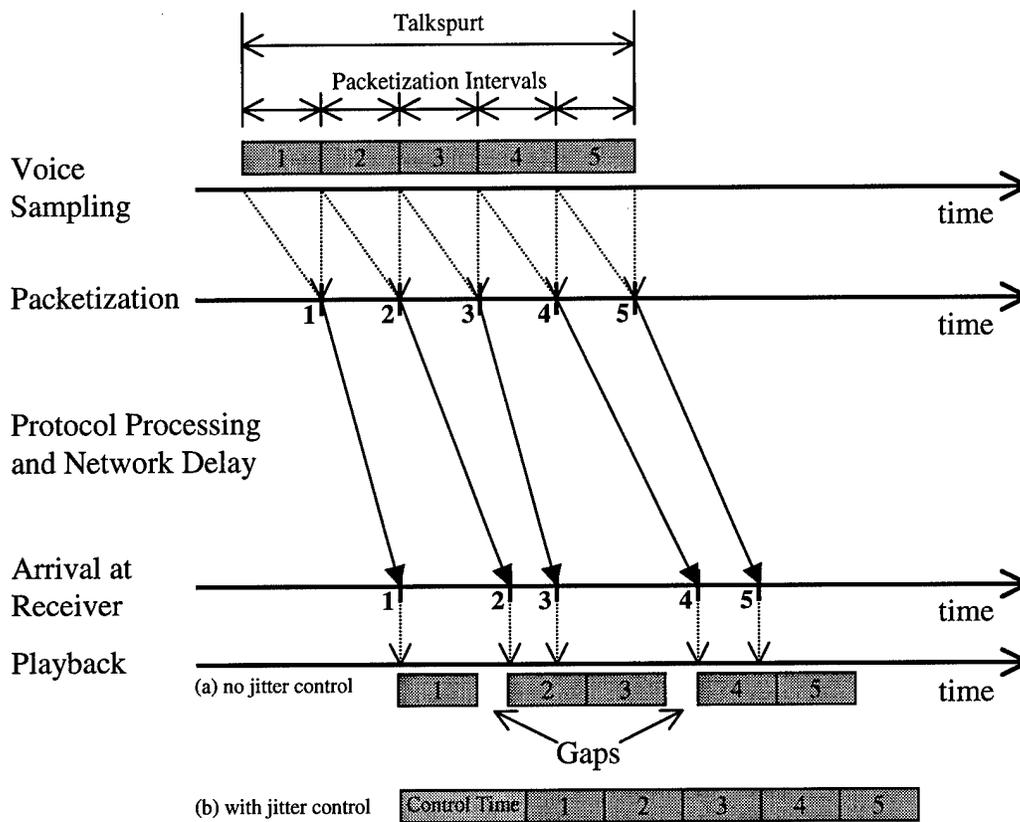
Figure 1.3 Transmission and Playback of a Talkspurt
