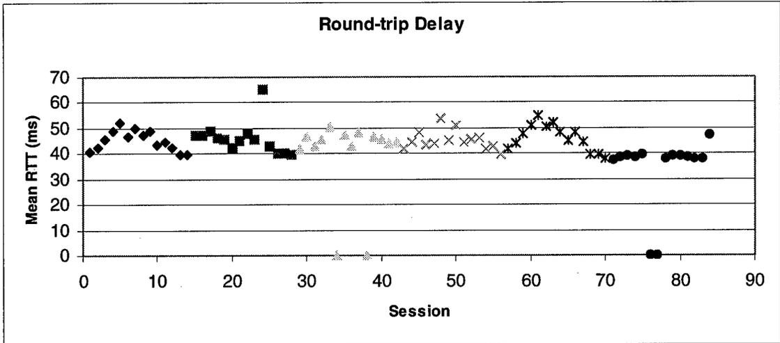
Figure C- 16 Mean Delays for AFIT-Hanscom AFB. Path
