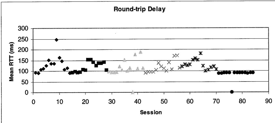
Figure C- 13 Mean Delays for AFIT-Travis AFB. Path
