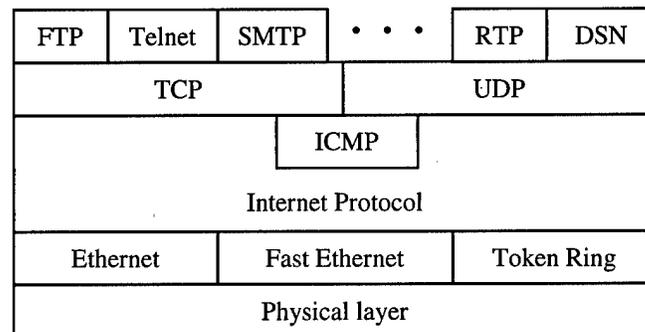
*Figure 2.1 Partition of the TCP/IP Protocol Family*
