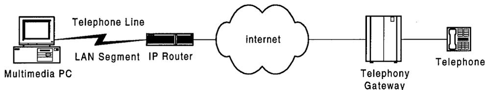
*Figure 2.6 PC-to-Phone/Phone-to-PC configuration*
