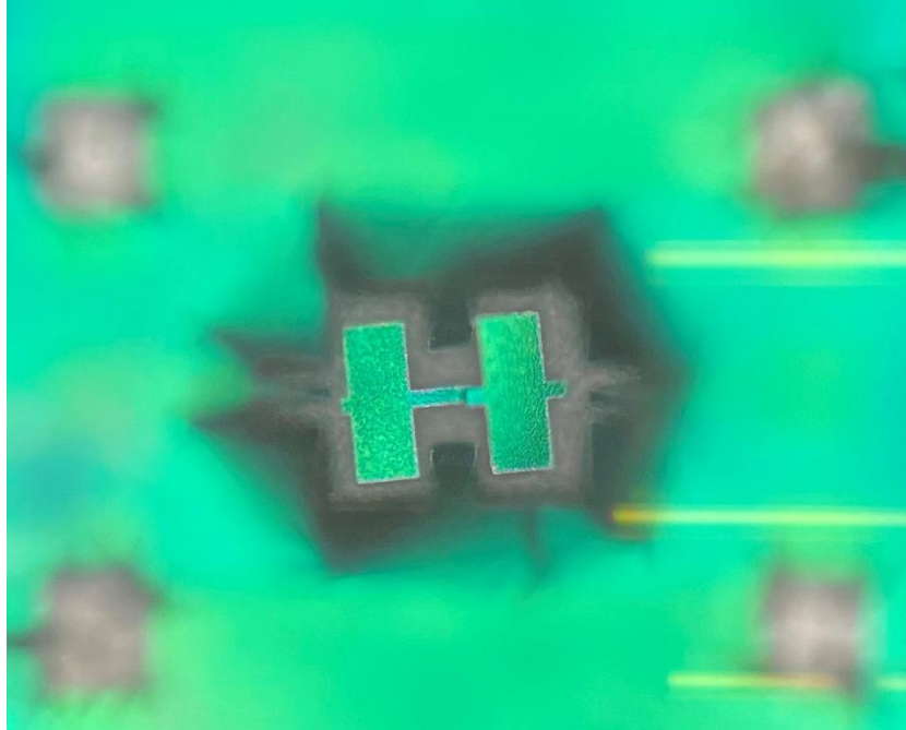
Figure 36: Fully released BST resonators using XeF 2 . The BST film began to crack and the resonators broke at the anchor points
