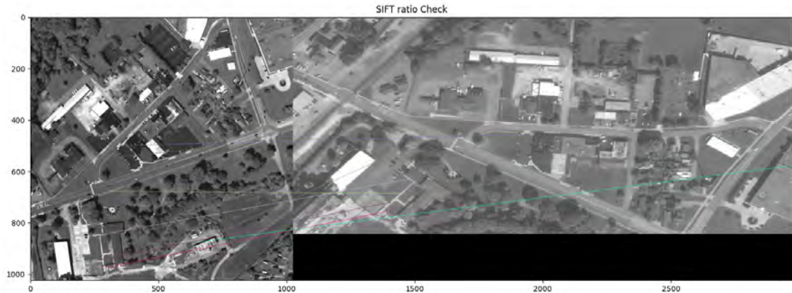
Figure 44: SIFT matches between the aerial and satellite imagery after being processed through the Ratio test
