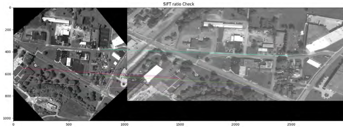
Figure 46: SIFT feature matching with the Ratio Test. Left image is a north aligned aerial photo and the right is a satellite image of the same local area
