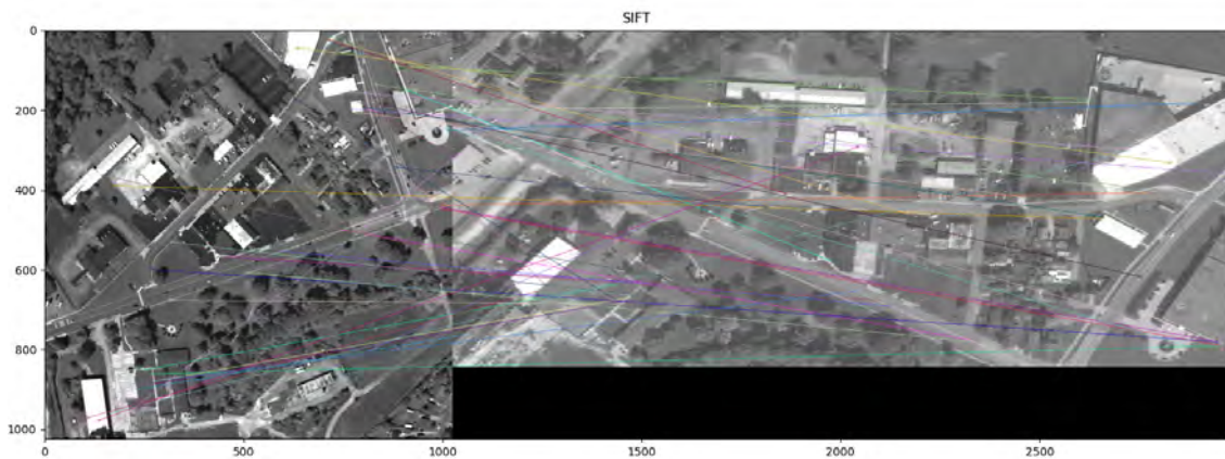
Figure 43: This figure depicts the SIFT matches between the aerial image, left, and the satellite image, right, collected from Digital Globe.
