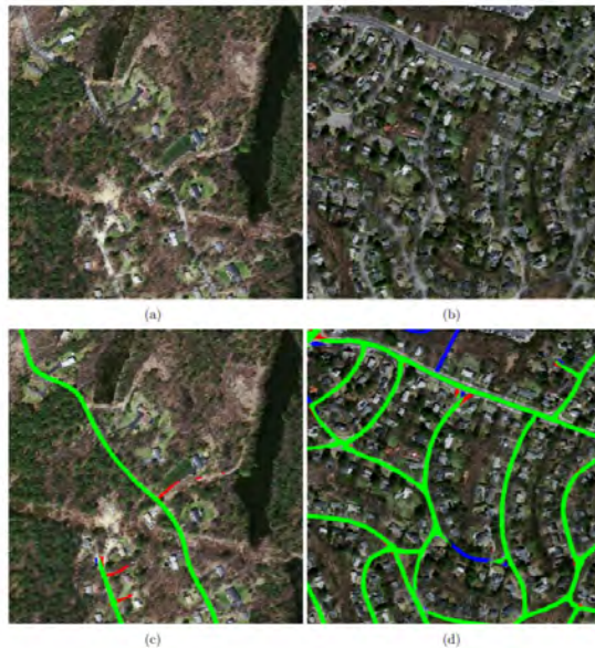
Figure 25: Massachusetts Road Dataset: (a) Rural environment input image. (b) Urban environment input image. (c) Image from (a) overlaid with truth mask depicting roads. (d) Image from (b) overlaid with truth mask depicting roads. [62]
