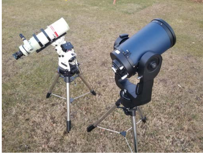
Figure 8. Takahashi 106mm with DVS240C camera and optical reducer on the left with the Meade 10-inch (no sensor attached) on the right.
