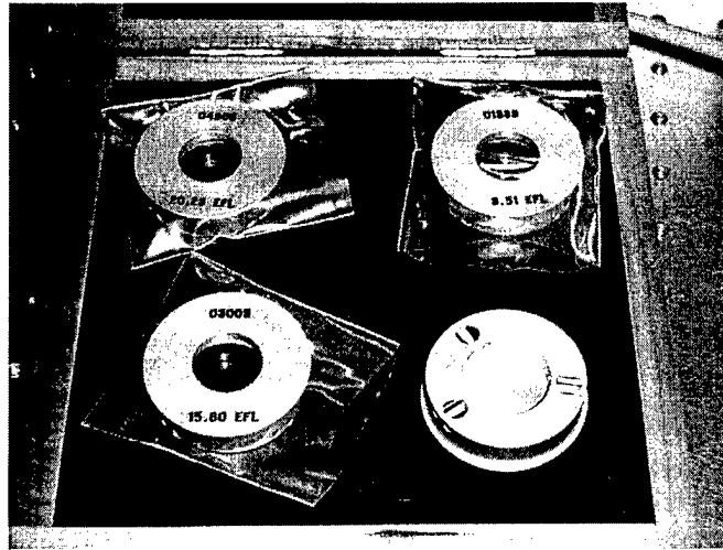
Figure 4.12 Wavescope Lenslet Arrays
