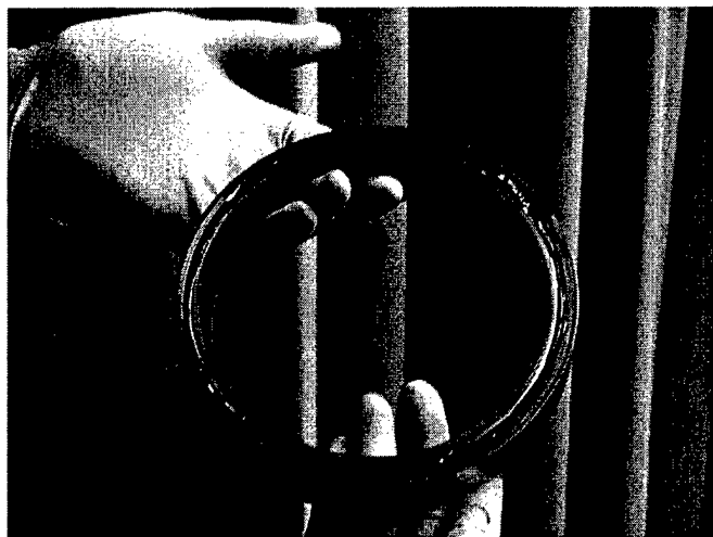
Figure 4.23 Epoxy Application to Mounting Ring
