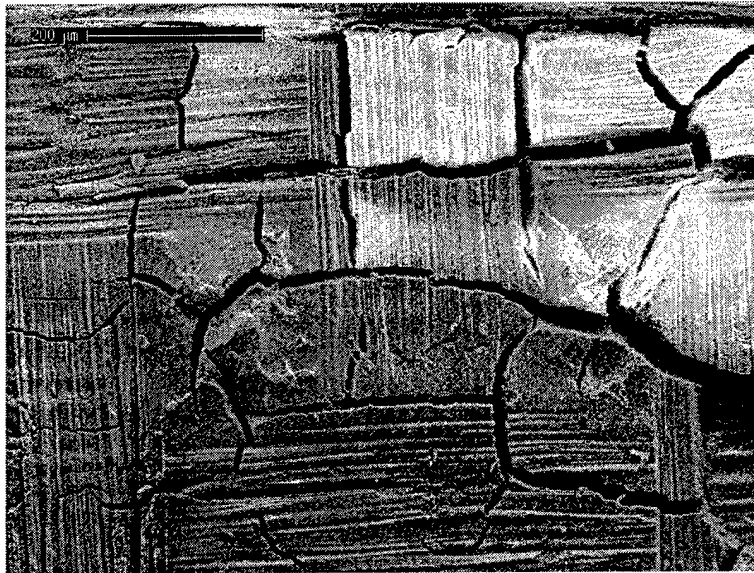
Figure 4-29 Surface of room temperature fatigue specimen after retained strength test, 140X
