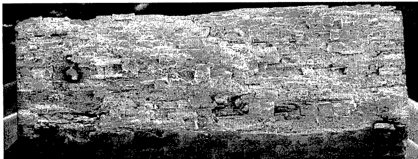
Figure 4-16 Fracture surface of GEN IV after 1200°C exposure, 20X
