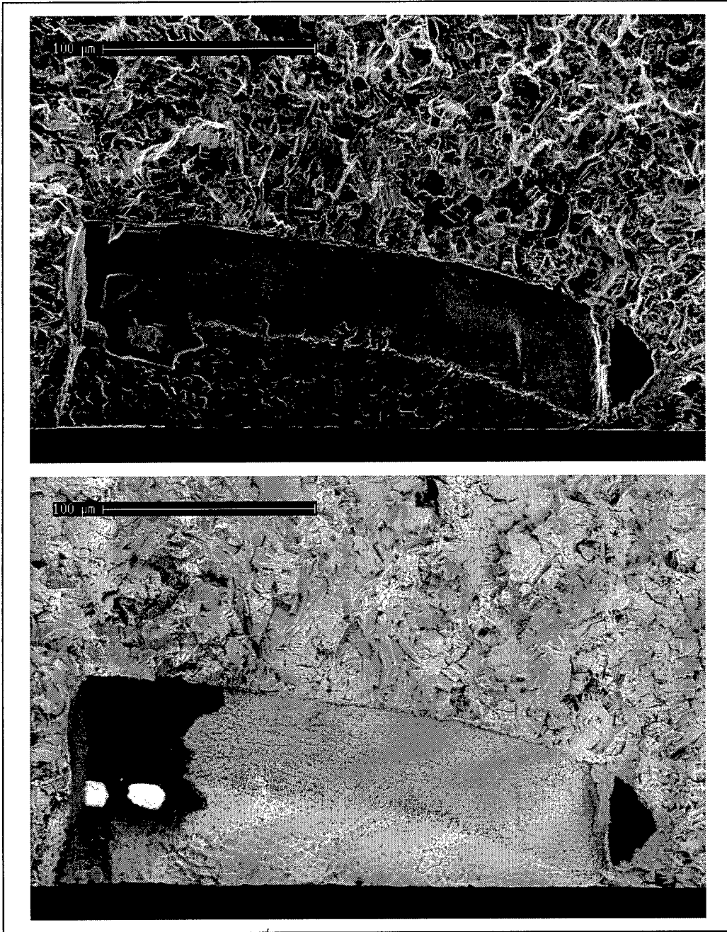
Figure 4.9: Specimen 200 (4:1 F/G) – detail view of the inclusion (the light-colored areas in the RBS image are remnants of the tungsten filament in the Trimarc 1 fiber)
