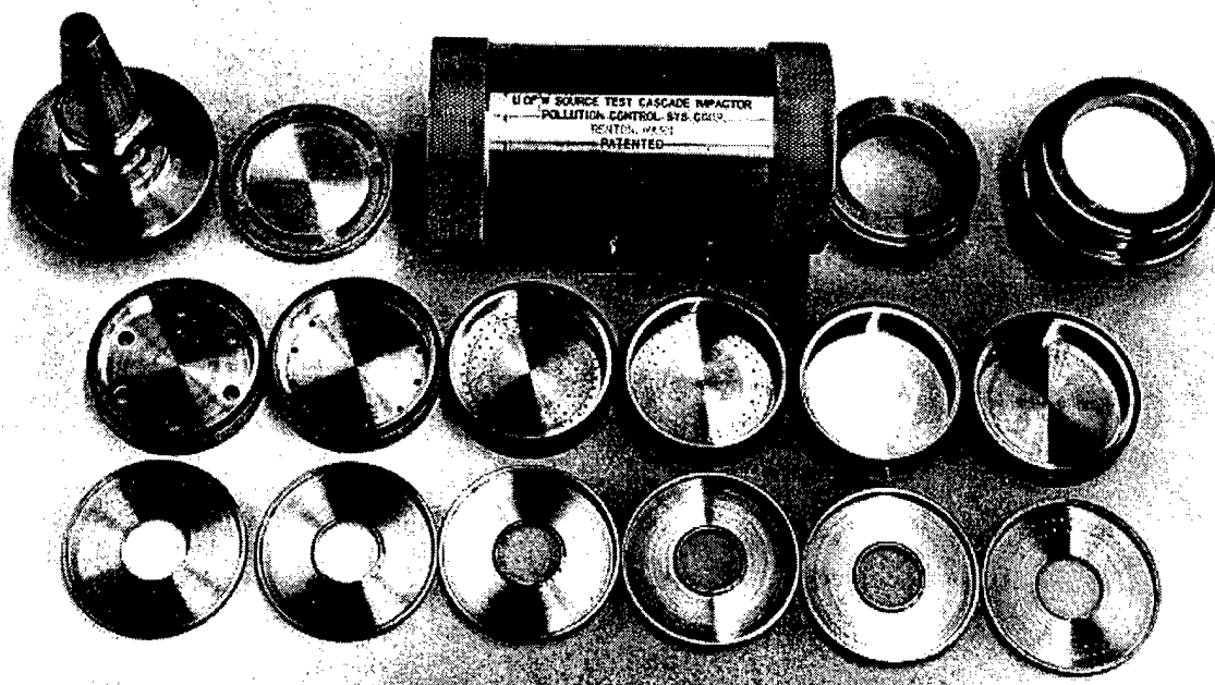
Figure 7. Cascade Impactor Assembly (PCSC, 2000)
