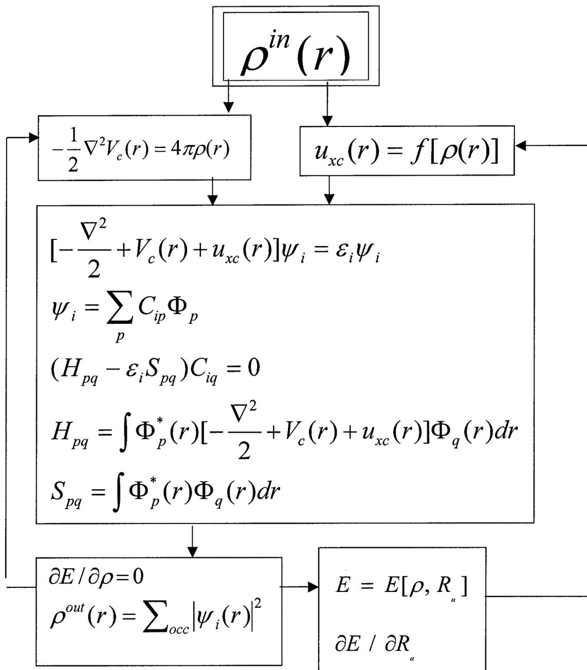
Figure 5. The flow chart of DFT-SCF calculation
