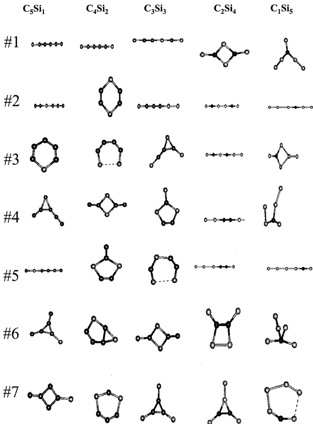
Figure 8. The structures of  $Si_mC_n$  clusters predicted by AM1 method
