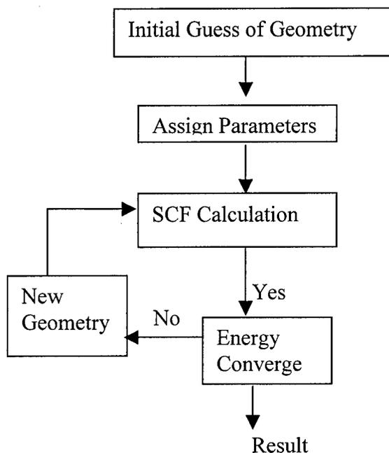
**Figure 4. The flow chart of AM1-SCF calculation**
