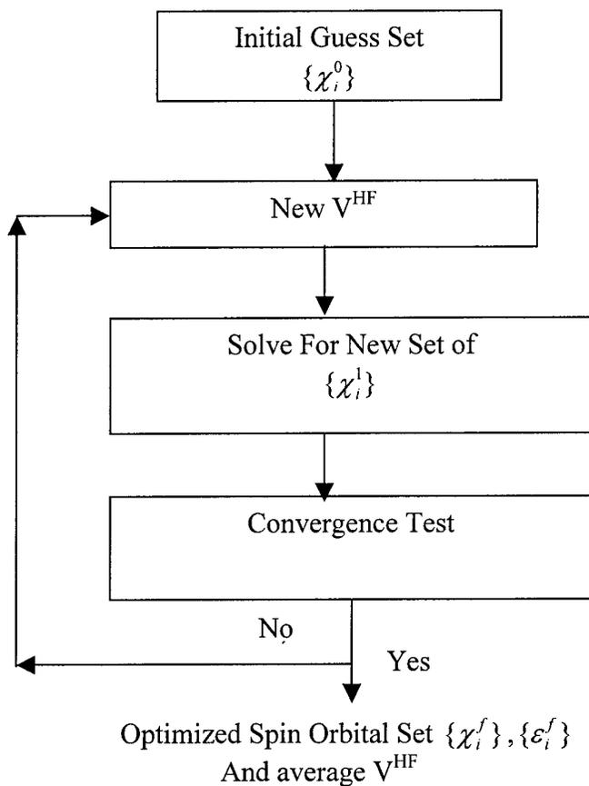
**Figure 3. The flow chart of HF-SCF calculation**
