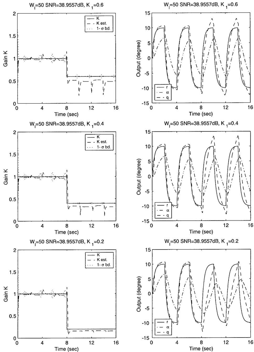
Figure 87. Moving window system ID algorithm ( $w_l = 50$ ), with adaptive smoother. Phugoid dynamics, fourth-order actuator model and parametric modeling error ( $M_\alpha = 5$  after failure) are included.  $K_{\delta_e} = -1.5$ .  $\sigma_\alpha = 0.03$  deg and  $\sigma_q = 0.1108$  deg / sec.  $K_1 = 0.6, 0.4$  and  $0.2$ .
