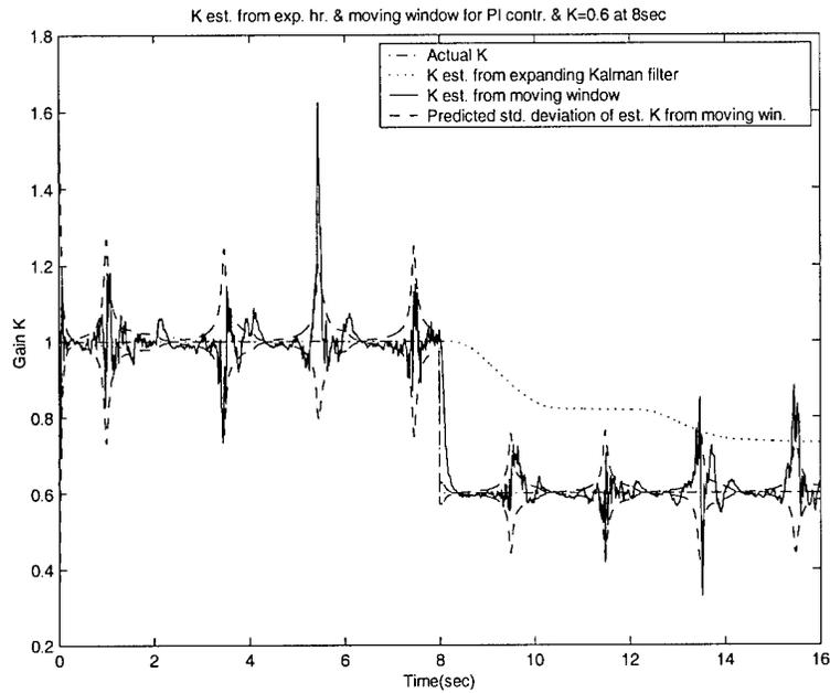
Figure 16. Comparison of expanding horizon and moving window estimation with fixed PI tracking controller.  $\sigma_\alpha = 0.03$  deg and  $\sigma_q = 0.1108$  deg/sec.  $K_1 = 0.6$ .
