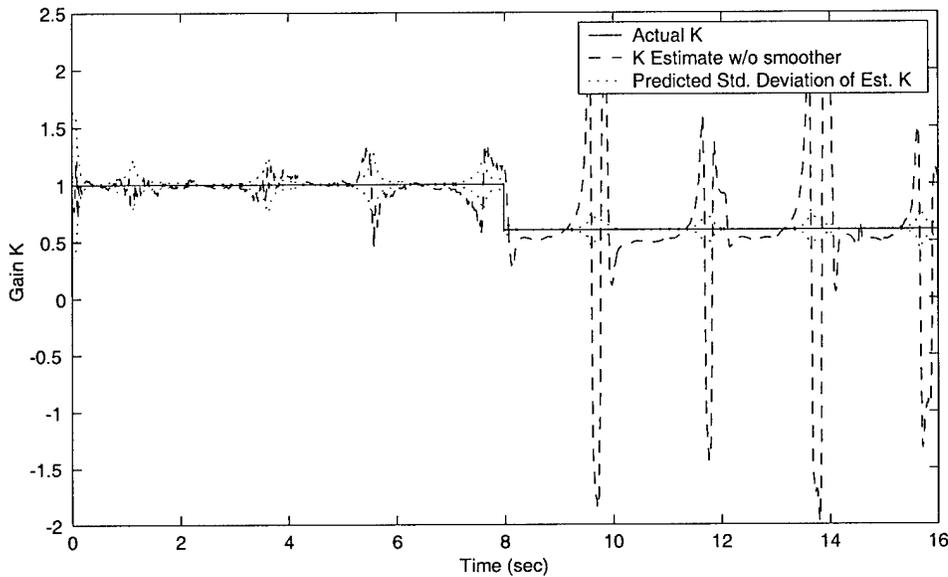
SP outs. when Phugoid dyns., 4th-order actu. & modeling err. are included w/o smoother. Failure  $K=0.6$  at 8sec  $K_{\delta_e}=-1.5$
