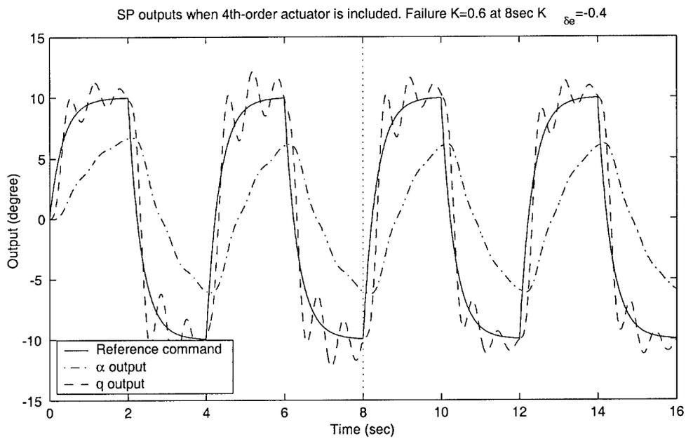
Figure 64. Smoothed  $\hat{K}$  and tracking performance when moving window system ID algorithm, adaptive smoother and fourth-order actuator are used.  $K_{\delta_e} = -0.4$ .  $\sigma_{\alpha} = 0.03$  deg and  $\sigma_q = 0.1108$  deg/sec. Failure at  $t=8$  sec. for  $K_1 = 0.6$ .
