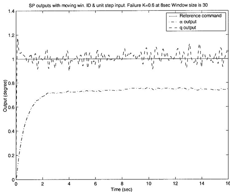
Figure 21.  $q$  and  $\alpha$  response when unit step ( $1\text{deg}/\text{sec}$  pitch rate) command is applied. Moving window system ID algorithm and fixed PI controller are used.  $\sigma_\alpha = 0.03\text{deg}$  and  $\sigma_q = 0.1108\text{deg}/\text{sec}$ .  $K_1 = 0.6$ .
