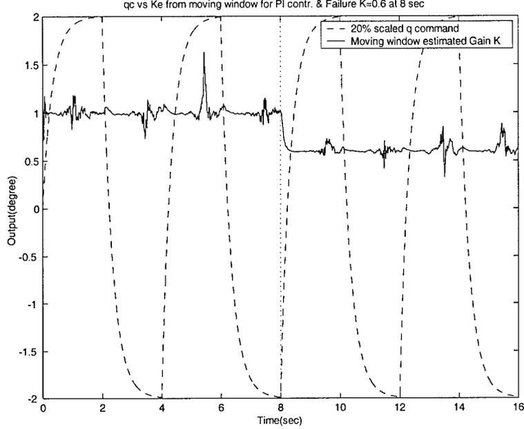
Figure 19. The reference command and the estimate  $\hat{K}$  provided by the moving window system identification algorithm.  $\sigma_\alpha = 0.03$  deg and  $\sigma_q = 0.1108$  deg / sec.  $K_1 = 0.6$ .
