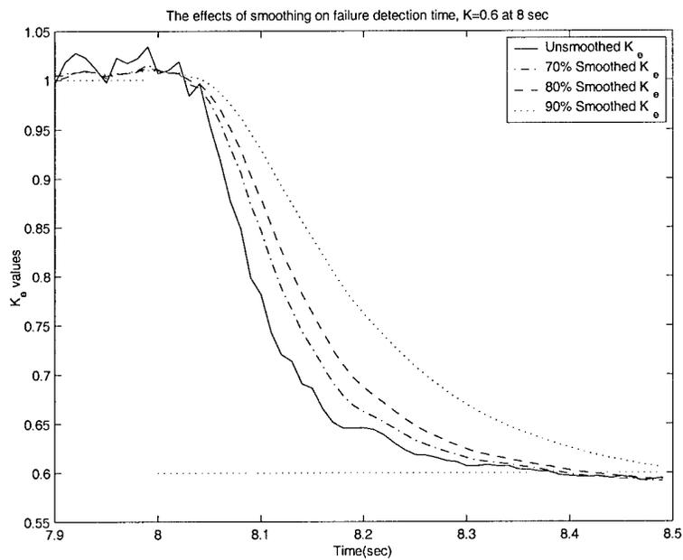
Figure 25. The effect of the fixed weights smoothing of estimated parameter on the settling time when moving window system ID is used.  $\sigma_\alpha = 0.03$  deg and  $\sigma_q = 0.1108$  deg / sec.  $K_1 = 0.6$ .
