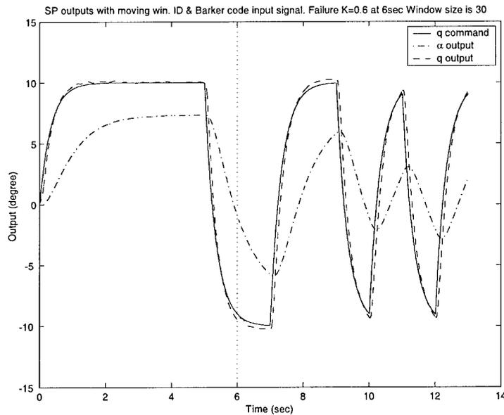
Figure 52.  $q$  and  $\alpha$  response when moving window system ID algorithm & 13-bit Barker code input signal are used.  $\sigma_\alpha = 0.03$  deg and  $\sigma_q = 0.1108$  deg/sec. Failure at  $t=6$  sec. and  $K_1 = 0.6$ .
