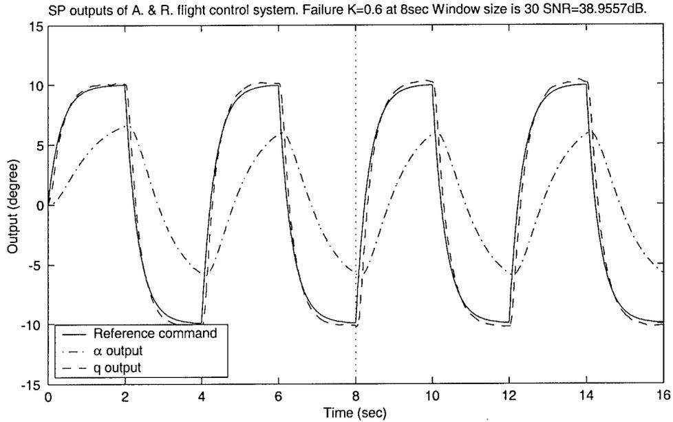
Figure 54. Smoothed  $\hat{K}$  and tracking performance when moving window system ID algorithm and adaptive smoother are used.  $SNR = 38.9557dB$  ( $\sigma_\alpha = 0.03 \text{ deg}$  and  $\sigma_q = 0.1108 \text{ deg / sec}$ ). Failure at  $t=8 \text{ sec}$ .  $K_1 = 0.6$ .
