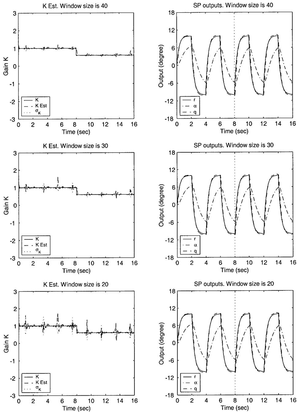
Figure 68. Parameter estimate  $\hat{K}$  and tracking performance when the moving window system ID algorithm is used without smoother.  $\sigma_\alpha = 0.03$  deg and  $\sigma_q = 0.1108$  deg/sec.  $K_1 = 0.6$ . Window lengths are 40, 30 and 20. No modeling error.
