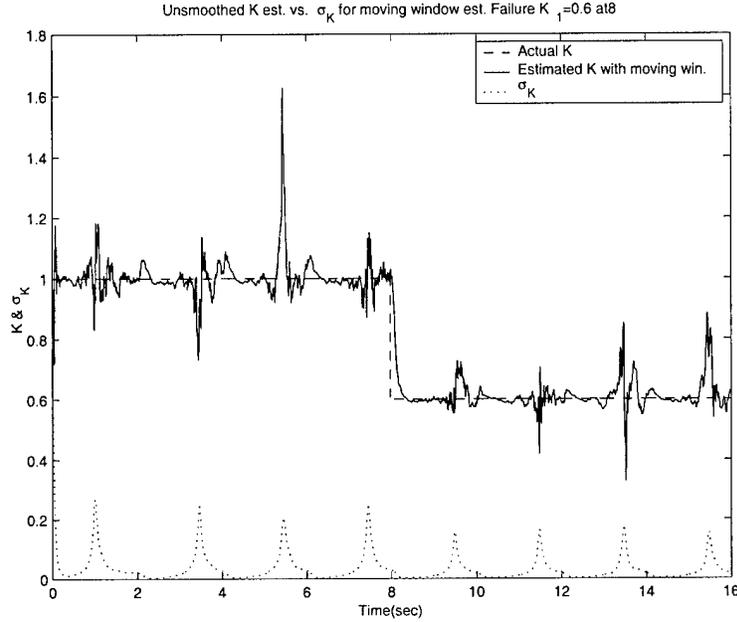
Figure 26. Loop gain estimate and predicted estimate error standard deviation when moving window system ID is used.  $\sigma_\alpha = 0.03 \text{ deg}$  and  $\sigma_q = 0.1108 \text{ deg/sec}$ .  $K_1 = 0.6$ .
