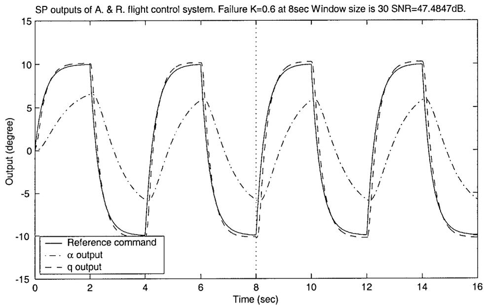
Figure 56. Smoothed  $\hat{K}$  and tracking performance when moving window system ID algorithm and adaptive smoother are used.  $SNR = 47.4847dB$  ( $\sigma_\alpha = 0.03$  deg and  $\sigma_q = 0.01108$  deg/sec). Failure at  $t=8$  sec.  $K_1 = 0.6$ .
