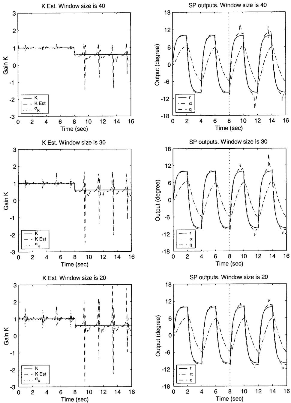
Figure 70. Parameter estimate  $\hat{K}$  and tracking performance when the moving window system ID algorithm is used without smoother.  $\sigma_\alpha = 0.03$  deg and  $\sigma_q = 0.1108$  deg/sec.  $K_1 = 0.6$ . Window lengths are 40, 30 and 20. With modeling error ( $M_\alpha = 5$ ) after failure.
