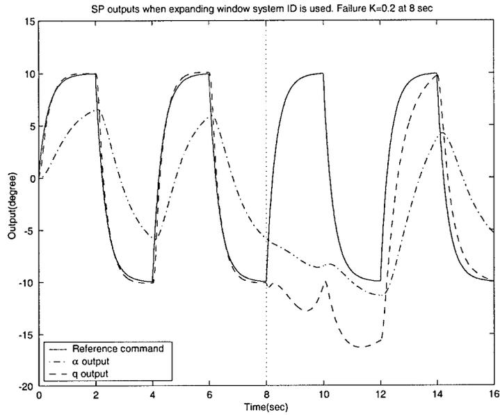
Figure 43.  $q$  and  $\alpha$  responses when expanding window system identification algorithm and reconfigurable control are used.  $\sigma_\alpha = 0.03$  deg and  $\sigma_q = 0.1108$  deg / sec .  $K_1 = 0.2$ .
