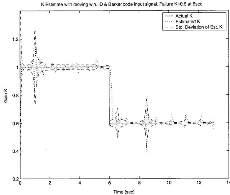
Figure 23.  $K$  estimate when moving window system ID algorithm, fixed PI Controller and 13-bit Barker input reference signal are used.  $\sigma_\alpha = 0.03$  deg and  $\sigma_q = 0.1108$  deg/sec. Failure at  $t_f = 6$  sec. and  $K_1 = 0.6$ .
