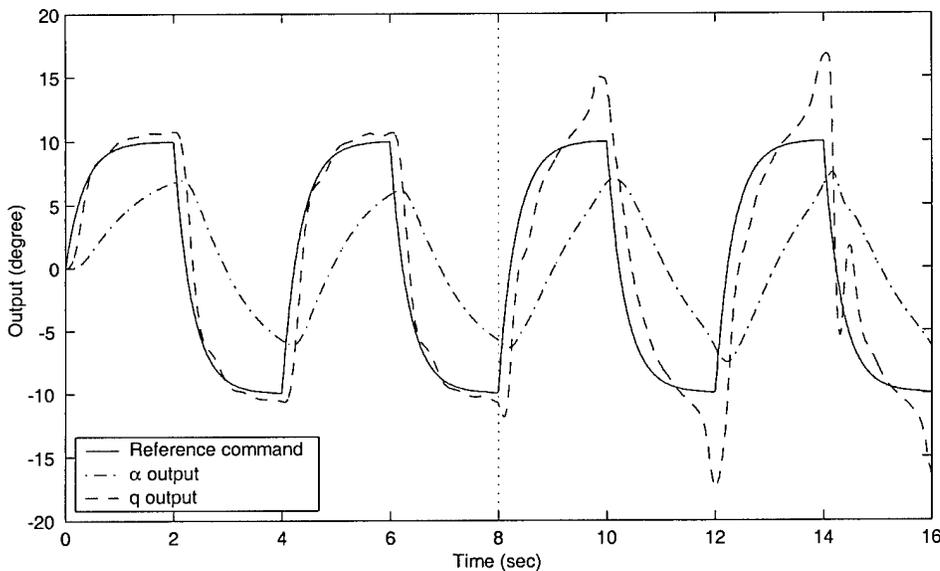
Figure 74. Parameter estimate  $\hat{K}$  and tracking performance. Moving window system ID algorithm ( $wl = 30$ ), without smoother. Phugoid dynamics, fourth-order actuator model and parametric modeling error ( $M_\alpha = 5$  after failure) are included.  $K_{\delta_e} = -1.5$ .  $\sigma_\alpha = 0.03$  deg and  $\sigma_q = 0.1108$  deg/sec.  $K_1 = 0.6$ .
