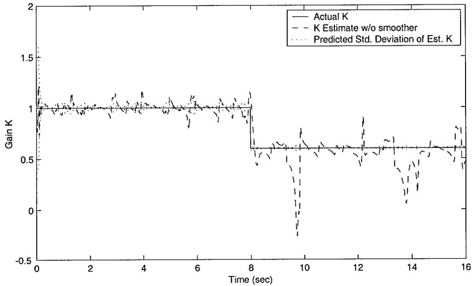
SP outs. when Phugoid dyns., 4th-order actu. & modeling err. are included w/o smoother. Failure  $K=0.6$  at 8sec  $K_{\delta_e}=-0.4$
