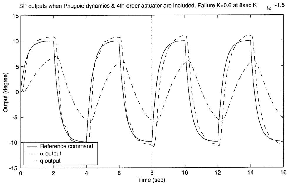
Figure 67. Smoothed  $\hat{K}$  and tracking performance when moving window system ID algorithm, adaptive smoother, Phugoid dynamics and fourth-order actuator are used.  $K_{\delta_e} = -1.5$ .  $\sigma_\alpha = 0.03$  deg and  $\sigma_q = 0.1108$  deg / sec.  $K_1 = 0.6$ .
