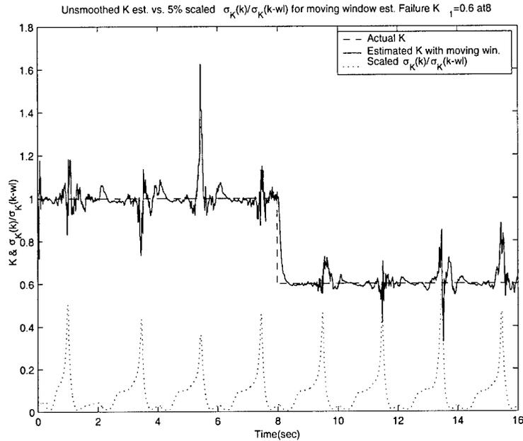
Figure 27. Loop gain estimate and  $\sigma_K(k)/\sigma_K(k-w_l)$  when moving window system ID is used.  $\sigma_\alpha = 0.03$  deg and  $\sigma_q = 0.1108$  deg/sec.  $K_1 = 0.6$ . (where  $w_l$  denotes the window length)
