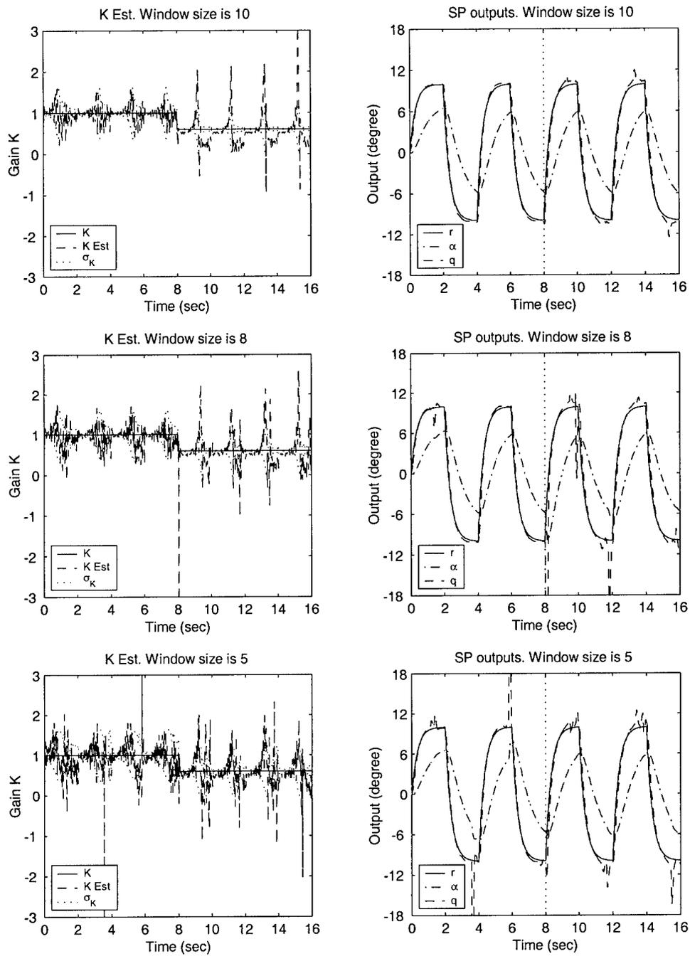
Figure 71. Parameter estimate  $\hat{K}$  and tracking performance when the moving window system ID algorithm is used without smoother.  $\sigma_\alpha = 0.03$  deg and  $\sigma_q = 0.1108$  deg/sec.  $K_1 = 0.6$ . Window lengths are 10, 8 and 5. With modeling error ( $M_\alpha = 5$ ) after failure.
