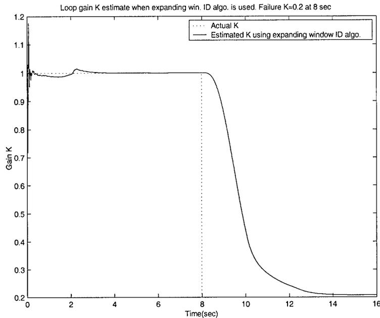
Figure 14. Loop gain estimation when  $K_1 = 0.2$ ,  $\sigma_\alpha = 0.03$  deg and  $\sigma_q = 0.1108$  deg/sec when an expanding window system ID algorithm is used.
