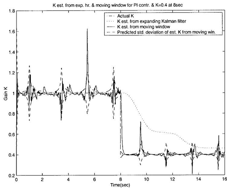
Figure 17. Comparison of expanding horizon and moving window estimation with fixed PI tracking controller.  $\sigma_\alpha = 0.03$  deg and  $\sigma_q = 0.1108$  deg/sec.  $K_1 = 0.4$ .
