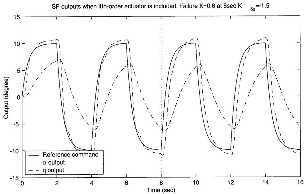
Figure 65. Smoothed  $\hat{K}$  and tracking performance when moving window system ID algorithm, adaptive smoother and fourth-order actuator are used.  $K_{\delta_e} = -1.5$ .  $\sigma_\alpha = 0.03$  deg and  $\sigma_q = 0.1108$  deg/sec.  $K_1 = 0.6$ .
