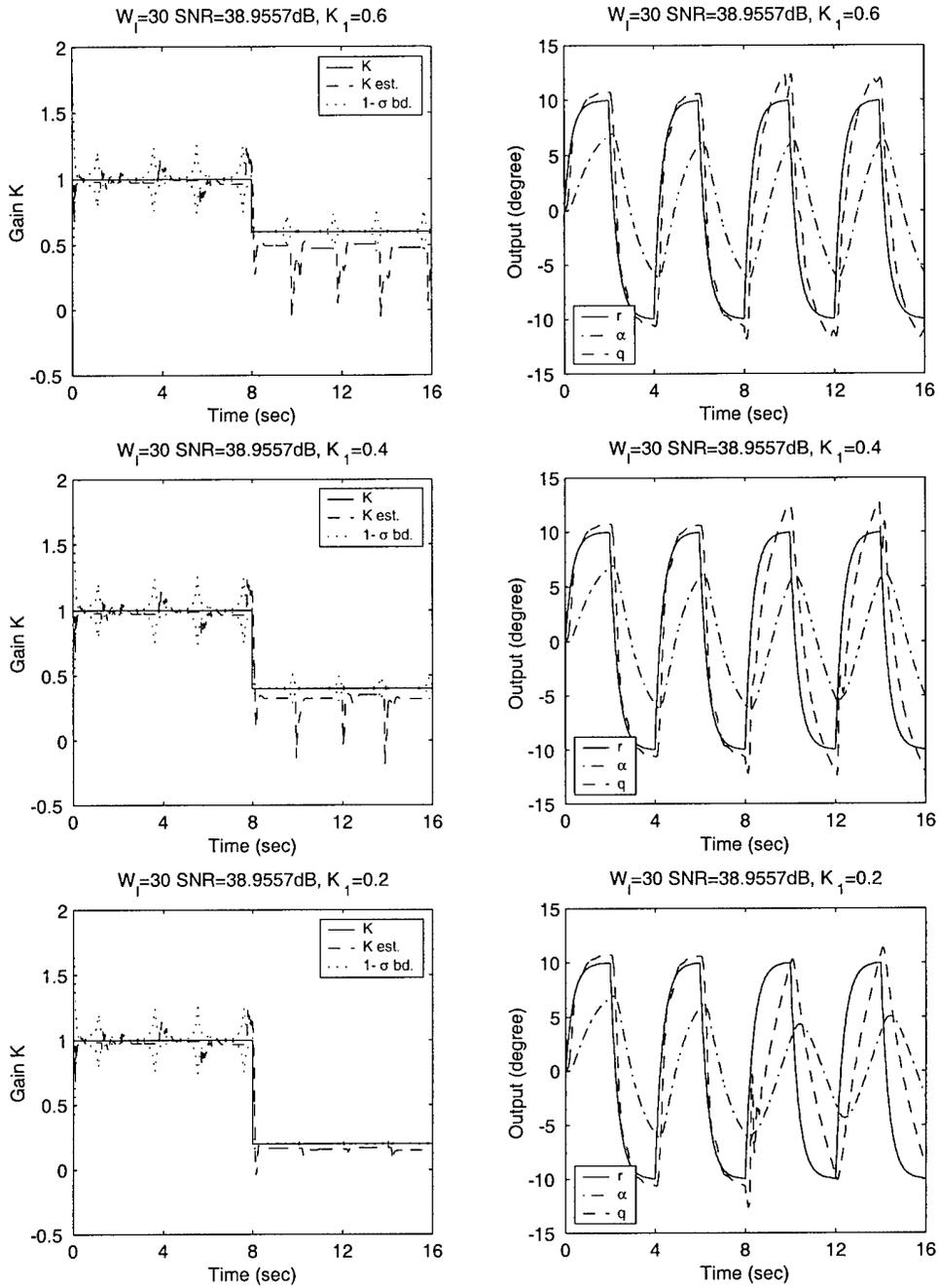
Figure 89. Moving window system ID algorithm ( $w_l = 30$ ), with adaptive smoother. Phugoid dynamics, fourth-order actuator model and parametric modeling error ( $M_\alpha = 5$  after failure) are included.  $K_{\delta_e} = -1.5$ .  $\sigma_\alpha = 0.03$  deg and  $\sigma_q = 0.1108$  deg/sec.  $K_1 = 0.6, 0.4$  and  $0.2$ .
