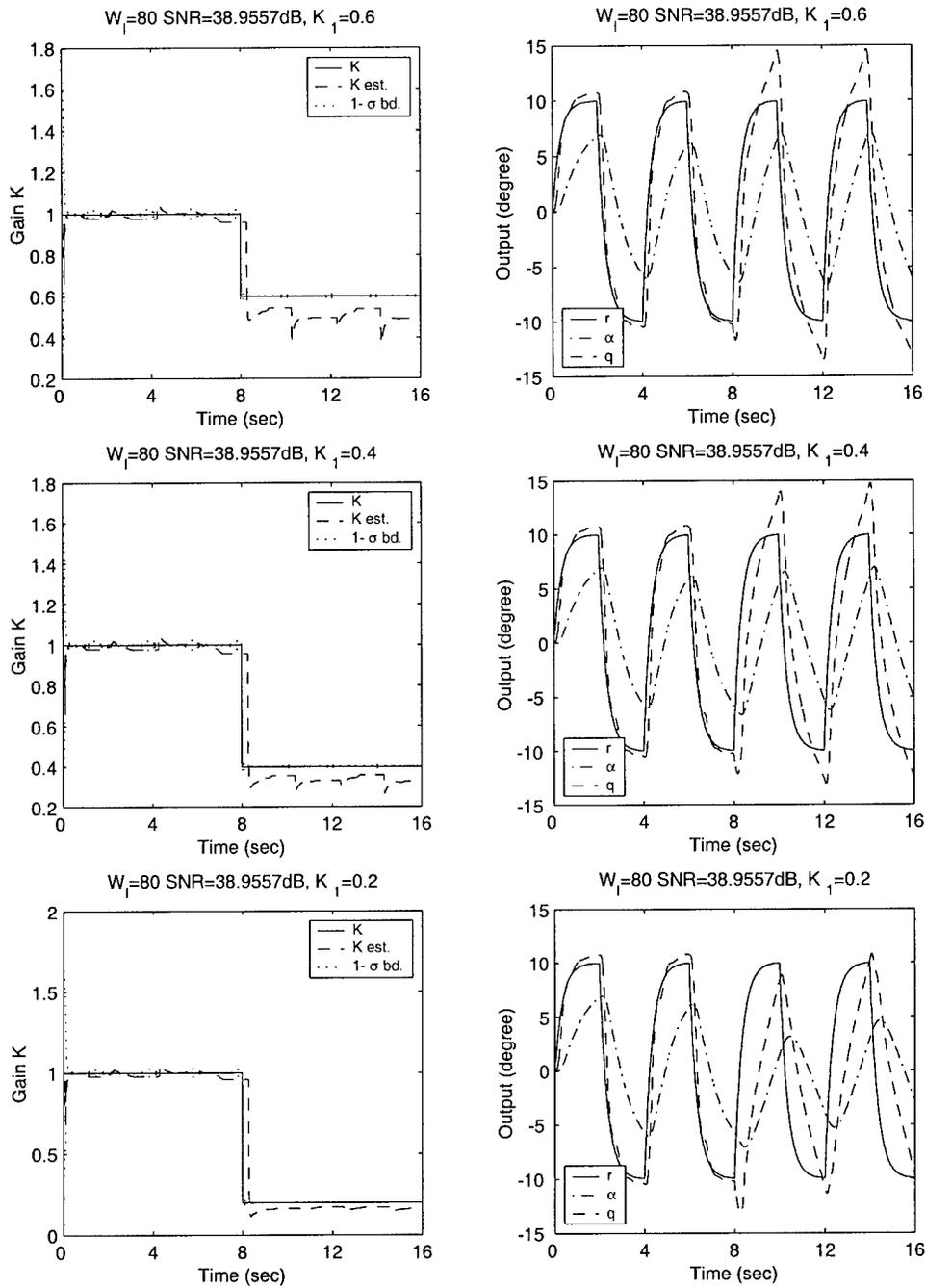
Figure 85. Moving window system ID algorithm ( $w_l = 80$ ), with adaptive smoother. Phugoid dynamics, fourth-order actuator model and parametric modeling error ( $M_\alpha = 5$  after failure) are included.  $K_{\delta_e} = -1.5$ .  $\sigma_\alpha = 0.03$  deg and  $\sigma_q = 0.1108$  deg/sec.  $K_1 = 0.6, 0.4$  and  $0.2$ .
