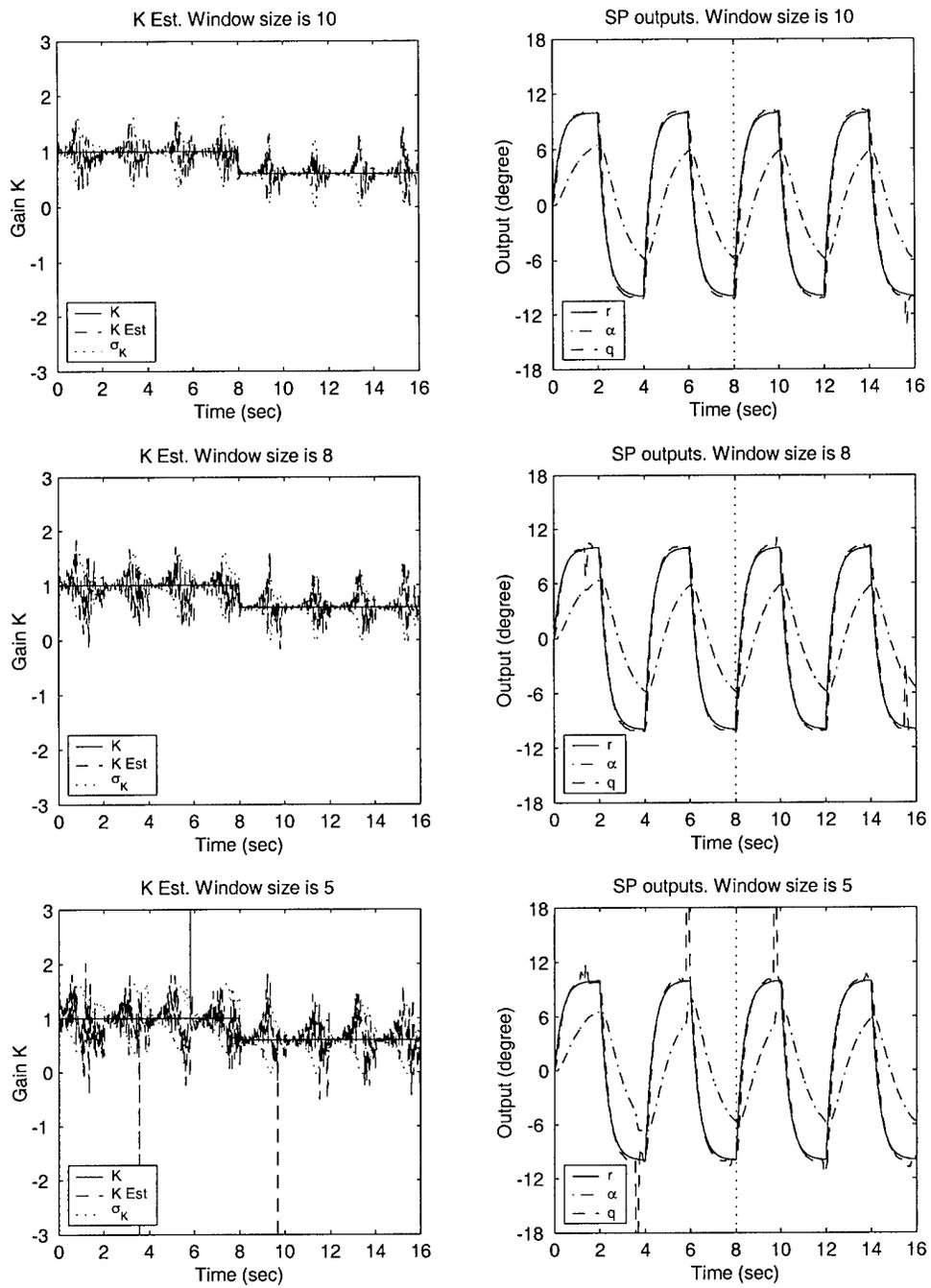
Figure 69. Parameter estimate  $\hat{K}$  and tracking performance when the moving window system ID algorithm is used without smoother.  $\sigma_\alpha = 0.03$  deg and  $\sigma_q = 0.1108$  deg/sec.  $K_1 = 0.6$ . Window lengths are 10, 8 and 5. No modeling error.
