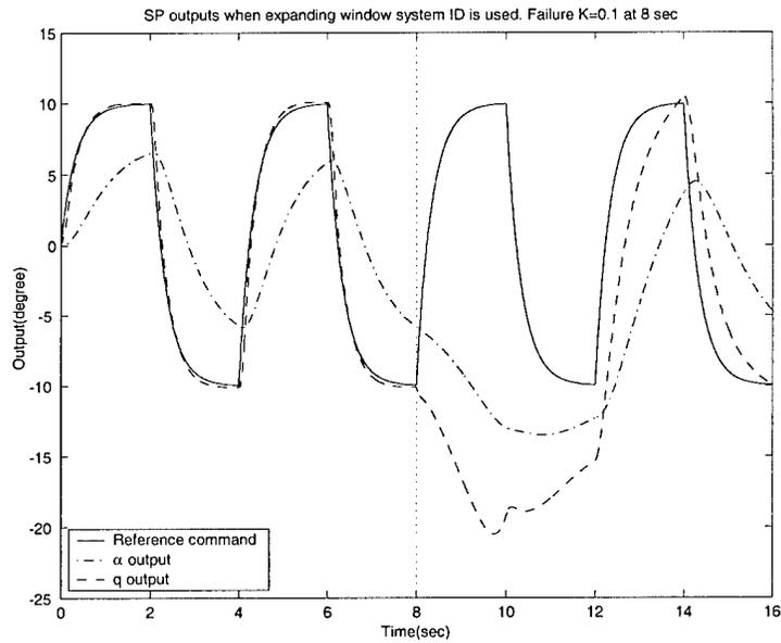
Figure 44.  $q$  and  $\alpha$  responses when expanding window system identification algorithm and reconfigurable control are used.  $\sigma_\alpha = 0.03$  deg and  $\sigma_q = 0.1108$  deg / sec .  $K_1 = 0.1$ .
