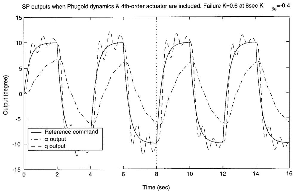
Figure 66. Smoothed  $\hat{K}$  and tracking performance when moving window system ID algorithm, adaptive smoother, Phugoid dynamics and fourth-order actuator are used.  $K_{\delta_e} = -0.4$ .  $\sigma_\alpha = 0.03$  deg and  $\sigma_q = 0.1108$  deg/sec.  $K_1 = 0.6$ .
