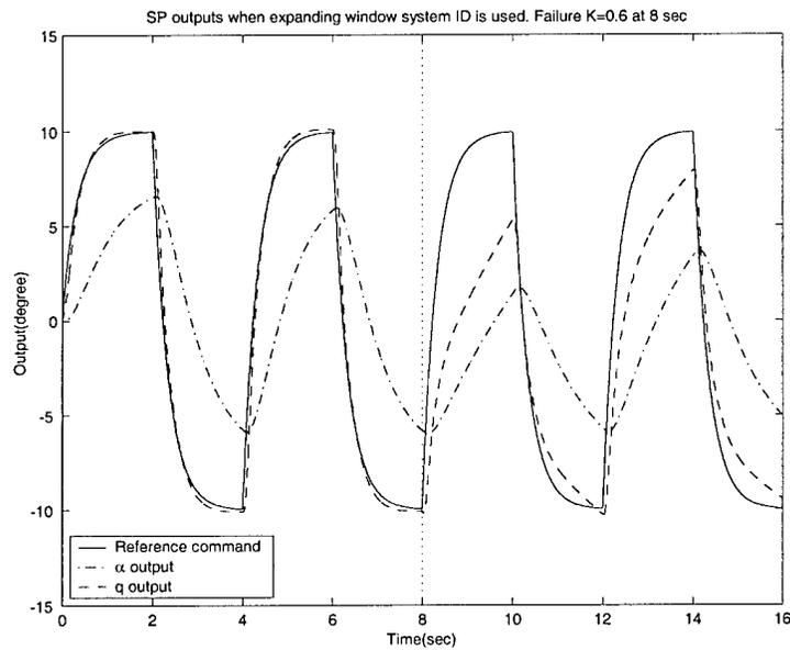
Figure 42.  $q$  and  $\alpha$  responses when expanding window system identification algorithm and reconfigurable control are used.  $\sigma_\alpha = 0.03$  deg and  $\sigma_q = 0.1108$  deg / sec .  $K_1 = 0.6$ .
