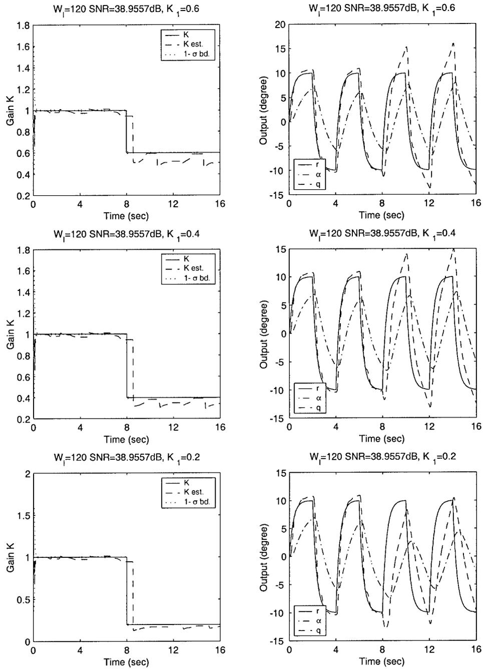
Figure 83. Moving window system ID algorithm ( $wl = 120$ ), with adaptive smoother. Phugoid dynamics, fourth-order actuator model and parametric modeling error ( $M_\alpha = 5$  after failure) are included.  $K_{\delta_e} = -1.5$ .  $\sigma_\alpha = 0.03$  deg and  $\sigma_q = 0.1108$  deg/sec.  $K_1 = 0.6, 0.4$  and  $0.2$ .
