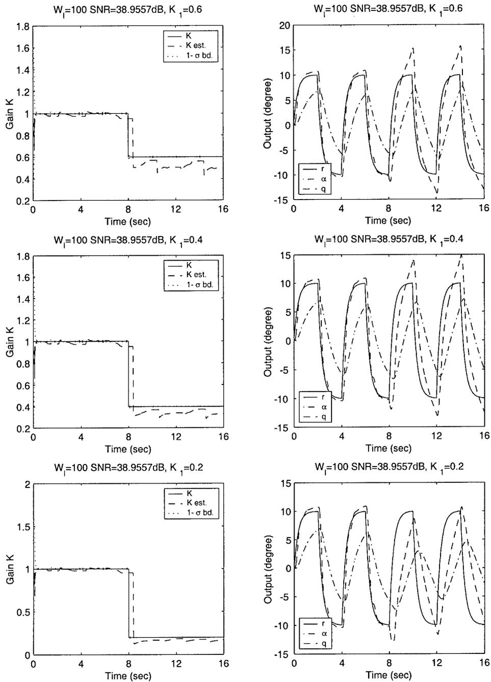
Figure 84. Moving window system ID algorithm ( $w_l = 100$ ), with adaptive smoother. Phugoid dynamics, fourth-order actuator model and parametric modeling error ( $M_\alpha = 5$  after failure) are included.  $K_{\delta_e} = -1.5$ .  $\sigma_\alpha = 0.03$  deg and  $\sigma_q = 0.1108$  deg / sec.  $K_1 = 0.6, 0.4$  and  $0.2$ .
