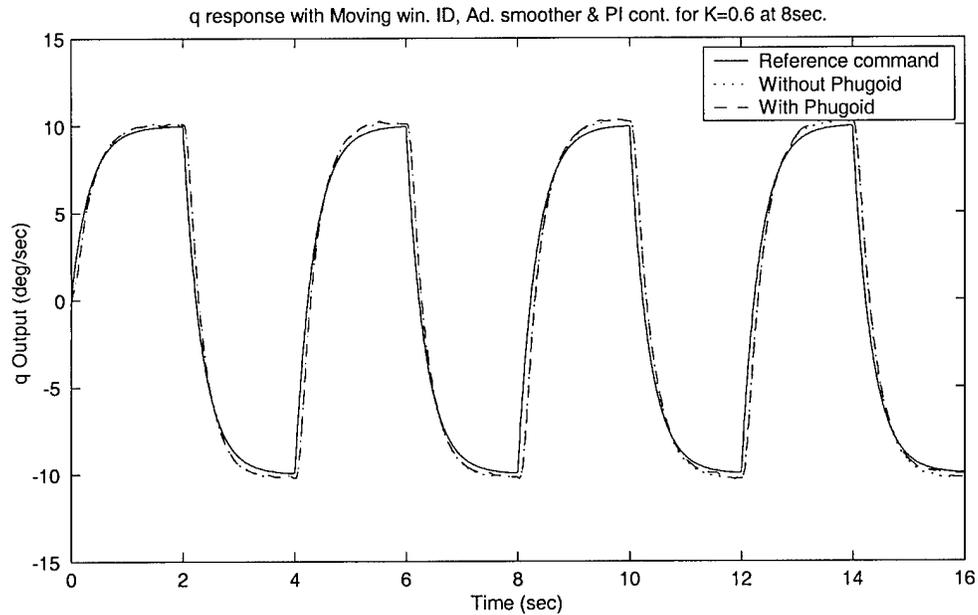
Figure 63. Phugoid dynamics are included -  $q$  response and adaptively smoothed  $\hat{K}$  when moving window system ID algorithm and adaptive smoother are used.  $\sigma_\alpha = 0.03$  deg and  $\sigma_q = 0.1108$  deg / sec.  $K_1 = 0.6$ .
