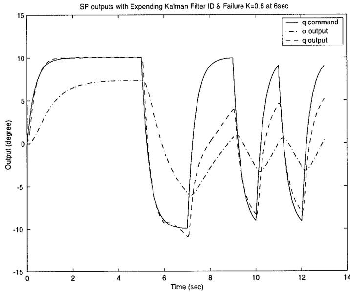
Figure 51.  $q$  and  $\alpha$  response when expanding window system identification algorithm & 13-bit Barker code input signal are used.  $\sigma_\alpha = 0.03$  deg and  $\sigma_q = 0.1108$  deg/sec. Failure at  $t=6$  sec. and  $K_1 = 0.6$ .
