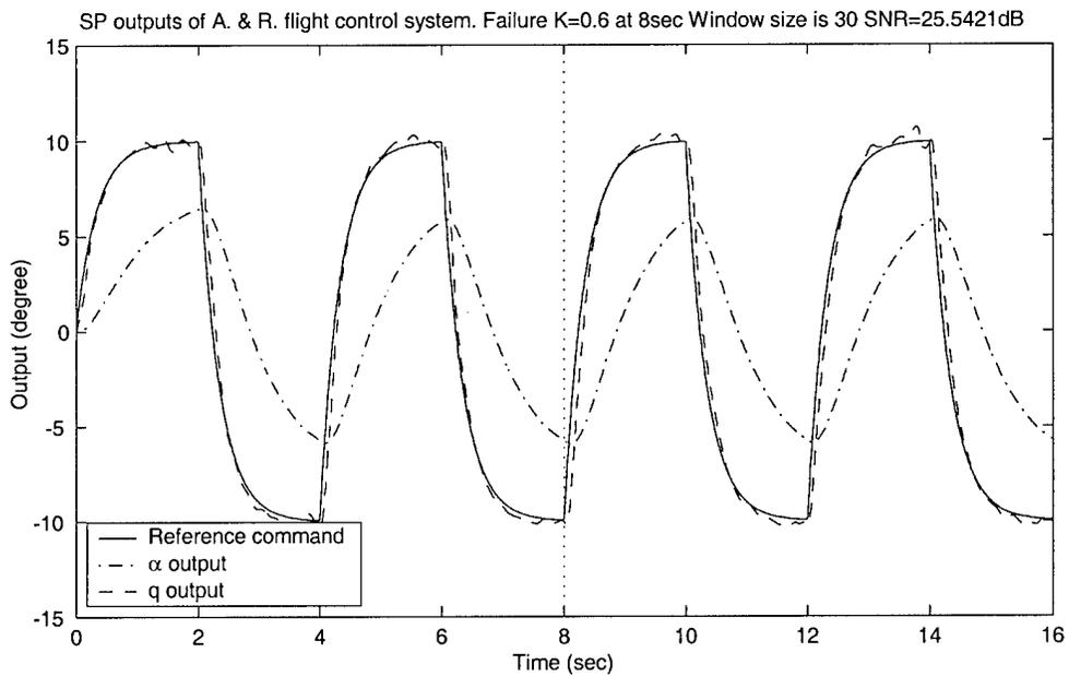
Figure 53. Smoothed  $\hat{K}$  and tracking performance when moving window system ID algorithm and adaptive smoother are used.  $SNR = 25.5421dB$  ( $\sigma_\alpha = 0.03 \text{ deg}$  and  $\sigma_q = 0.55534 \text{ deg/sec}$ ). Failure at  $t=8 \text{ sec}$ .  $K_1 = 0.6$ .
