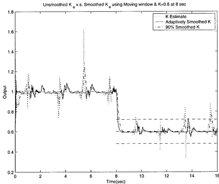
Figure 30. Loop gain estimate  $\hat{K}$  and smoothed  $\hat{K}_s$  when moving window system identification, fixed weights smoother and adaptive smoother are used.  $\sigma_\alpha = 0.03$  deg and  $\sigma_q = 0.1108$  deg/sec.  $K_1 = 0.6$ .
