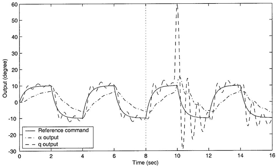
Figure 72. Parameter estimate  $\hat{K}$  and tracking performance. Moving window system ID algorithm ( $wl = 30$ ), without smoother. Phugoid dynamics, fourth-order actuator model and parametric modeling error ( $M_\alpha = 5$  after failure) are included.  $K_{\delta_e} = -0.4$ .  $\sigma_\alpha = 0.03$  deg and  $\sigma_q = 0.1108$  deg/sec.  $K_1 = 0.6$ .
