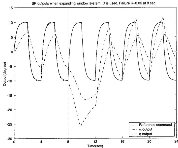
Figure 45.  $q$  and  $\alpha$  responses when expanding window system identification algorithm and reconfigurable control are used.  $\sigma_\alpha = 0.03 \text{ deg}$  and  $\sigma_q = 0.1108 \text{ deg/sec}$ .  $K_1 = 0.06$ .
