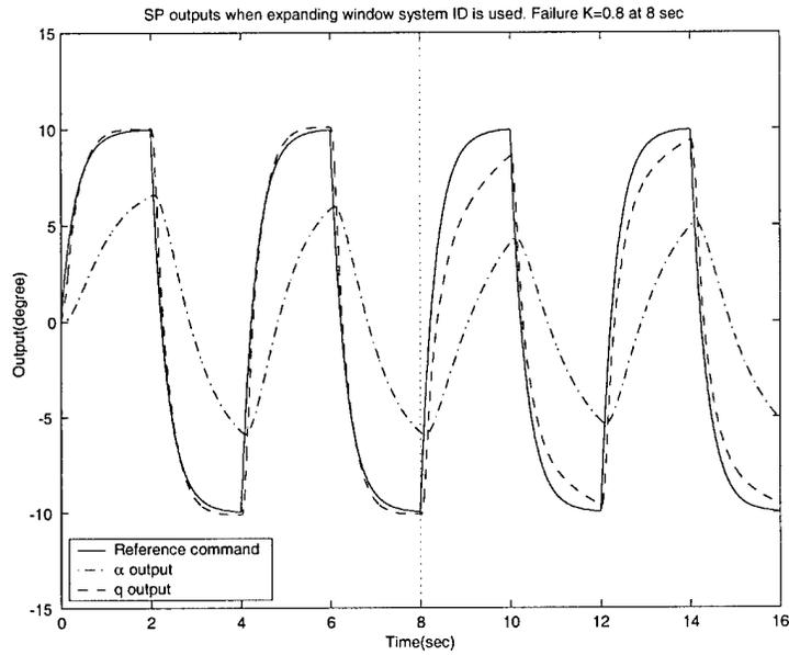
Figure 41.  $q$  and  $\alpha$  responses when expanding window system identification algorithm and reconfigurable control are used.  $\sigma_\alpha = 0.03$  deg and  $\sigma_q = 0.1108$  deg / sec .  $K_1 = 0.8$ .
