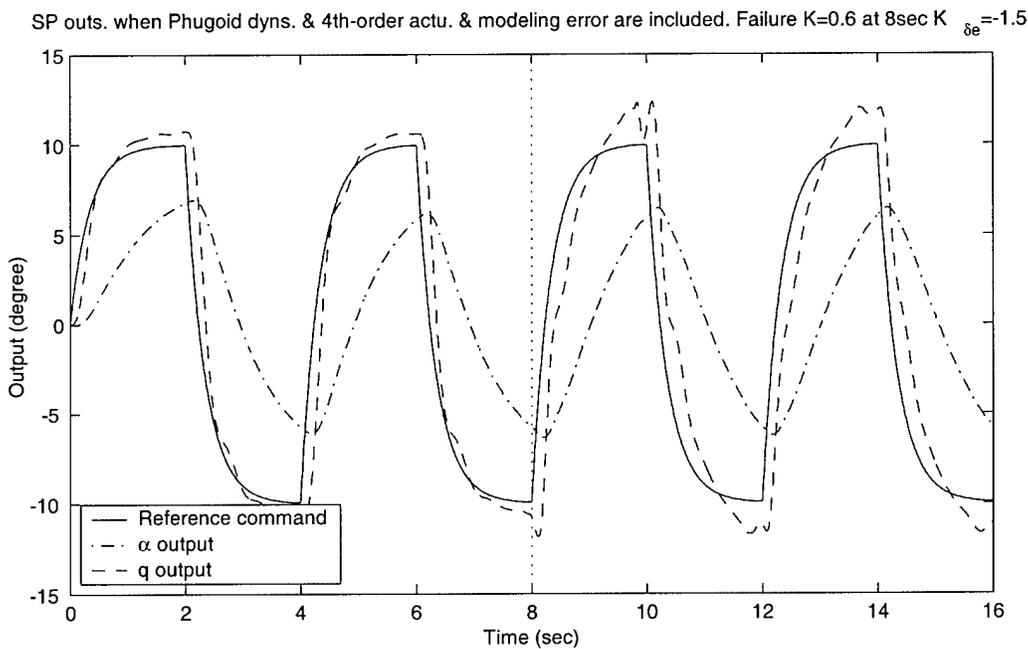
Figure 75. Smoothed  $\hat{K}$  and tracking performance. Moving window system ID algorithm ( $wl = 30$ ), with adaptive smoother. Phugoid dynamics, fourth-order actuator model and parametric modeling error ( $M_\alpha = 5$  after failure) are included.  $K_{\delta_e} = -1.5$ .  $\sigma_\alpha = 0.03$  deg and  $\sigma_q = 0.1108$  deg/sec.  $K_1 = 0.6$ .
