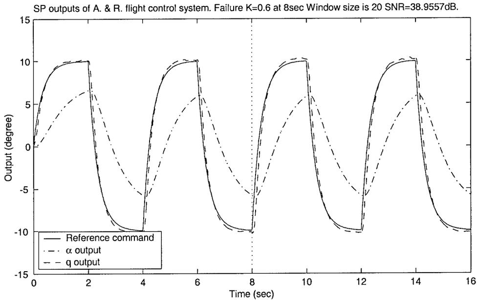
Figure 60. Smoothed  $\hat{K}$  and tracking performance when moving window system ID algorithm and adaptive smoother are used. Window size is 20,  $\sigma_\alpha = 0.03$  deg and  $\sigma_q = 0.1108$  deg / sec. Failure at  $t=8$  sec.  $K_1 = 0.6$ .
