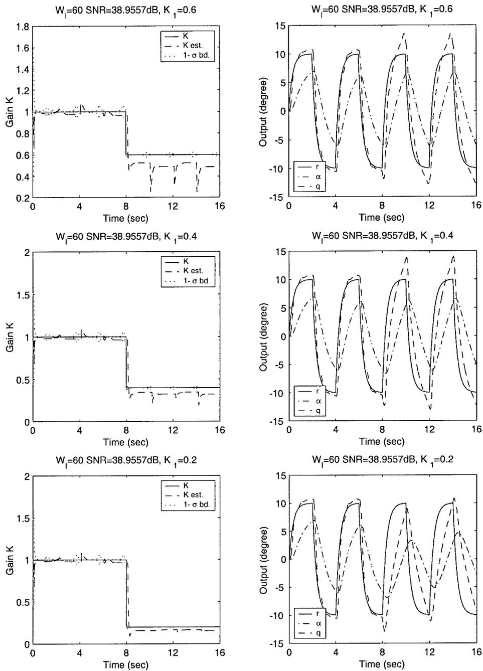
Figure 86. Moving window system ID algorithm ( $w_l = 60$ ), with adaptive smoother. Phugoid dynamics, fourth-order actuator model and parametric modeling error ( $M_\alpha = 5$  after failure) are included.  $K_{\delta_e} = -1.5$ .  $\sigma_\alpha = 0.03$  deg and  $\sigma_q = 0.1108$  deg/sec.  $K_1 = 0.6, 0.4$  and  $0.2$ .
