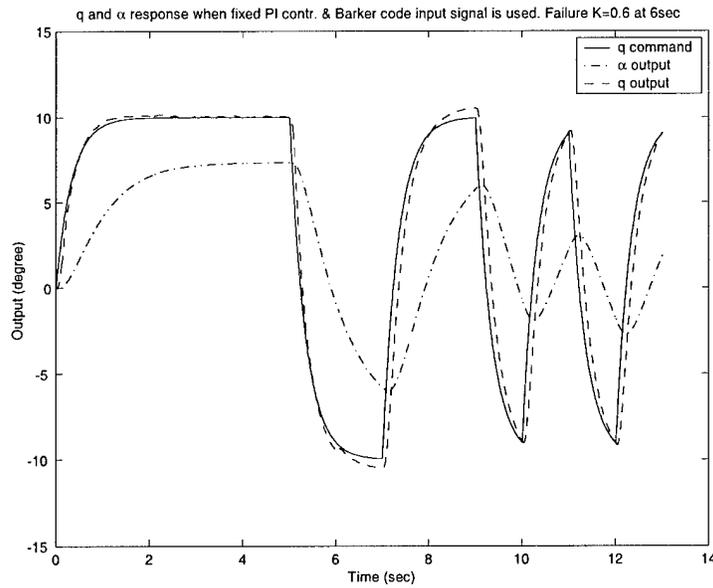
Figure 50.  $q$  and  $\alpha$  response when fixed PI controller & 13-bit Barker code input signal are used.  $\sigma_\alpha = 0.03$  deg and  $\sigma_q = 0.1108$  deg / sec. Failure at  $t=6$  sec. and  $K_1 = 0.6$ .
