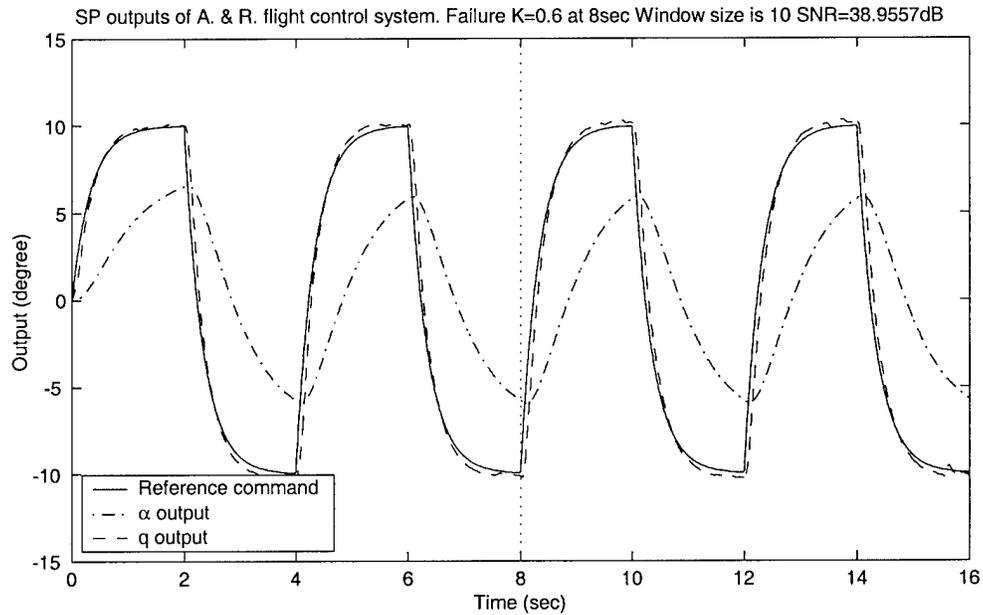
Figure 61. Smoothed  $\hat{K}$  and tracking performance when moving window system ID algorithm and adaptive smoother are used. Window size is 10,  $\sigma_\alpha = 0.03$  deg and  $\sigma_q = 0.1108$  deg / sec. Failure at  $t=8$  sec.  $K_1 = 0.6$ .
