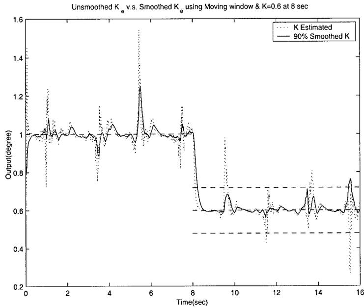
Figure 24. Nonsmoothed and 90% fixed weights smoothed loop gain estimate  $\hat{K}$  when moving window system ID algorithm is used.  $\sigma_\alpha = 0.03$  deg and  $\sigma_q = 0.1108$  deg / sec.  $K_1 = 0.6$ .
