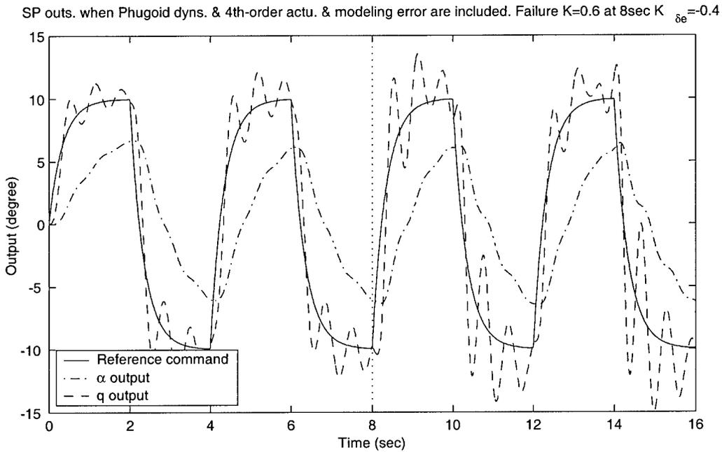
Figure 73. Smoothed  $\hat{K}$  and tracking performance. Moving window system ID algorithm ( $wl = 30$ ), with adaptive smoother. Phugoid dynamics, fourth-order actuator model and parametric modeling error ( $M_\alpha = 5$  after failure) are included.  $K_{\delta_e} = -0.4$ .  $\sigma_\alpha = 0.03$  deg and  $\sigma_q = 0.1108$  deg/sec.  $K_1 = 0.6$ .
