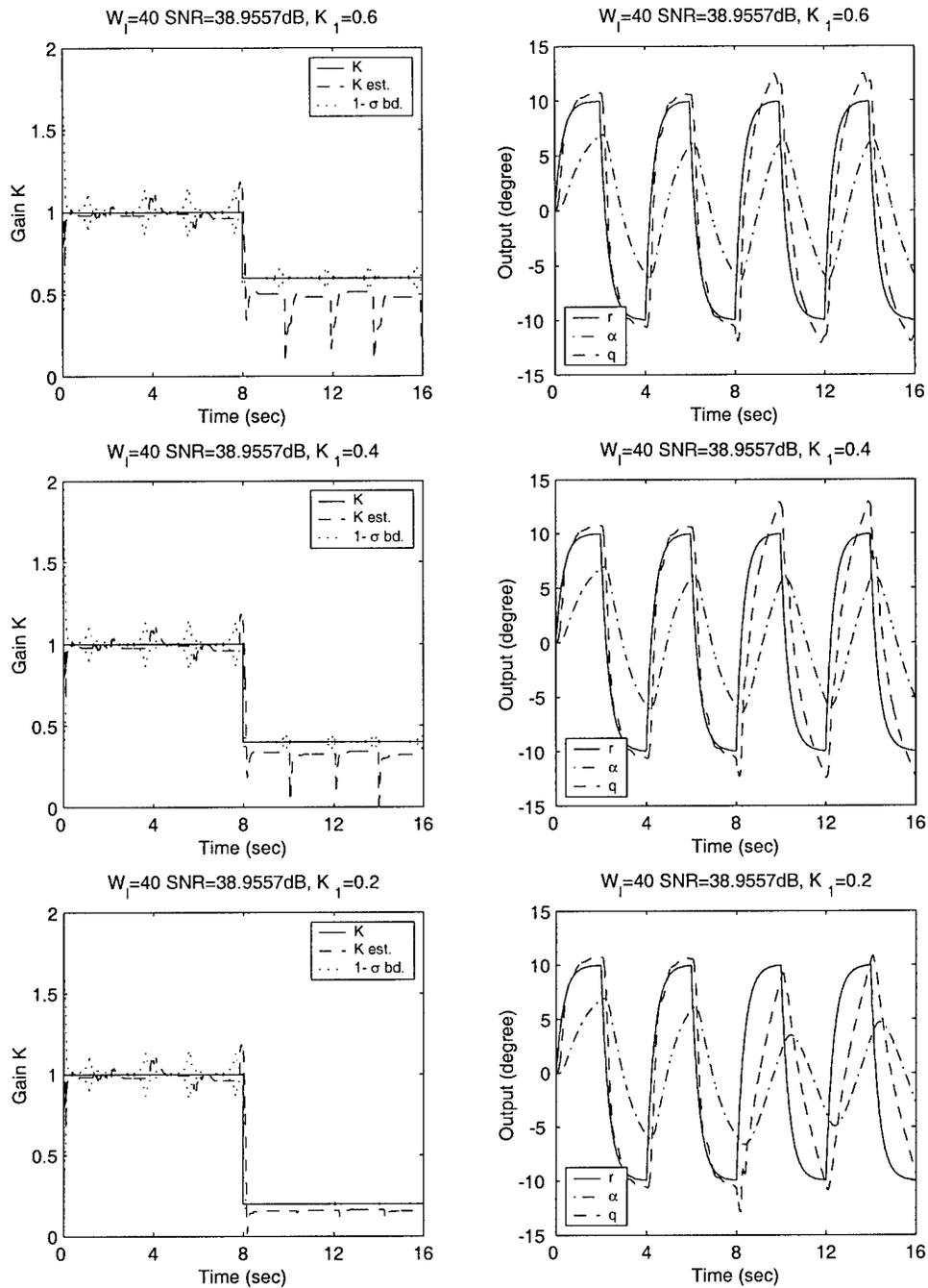
Figure 88. Moving window system ID algorithm ( $w_l = 40$ ), with adaptive smoother. Phugoid dynamics, fourth-order actuator model and parametric modeling error ( $M_\alpha = 5$  after failure) are included.  $K_{\delta_e} = -1.5$ .  $\sigma_\alpha = 0.03$  deg and  $\sigma_q = 0.1108$  deg / sec.  $K_1 = 0.6, 0.4$  and  $0.2$ .
