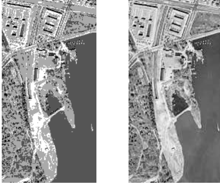
Figure 4-12 Comparison of 2-bit image with 8-bit image
