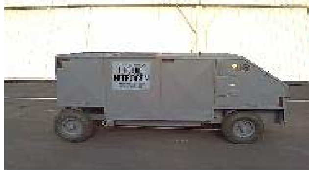
Figure 4. Nitrogen Servicing Unit
