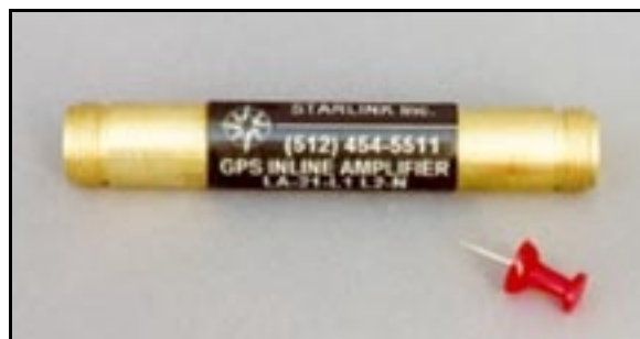
Figure 73. Inline GPS Signal Amplifier
