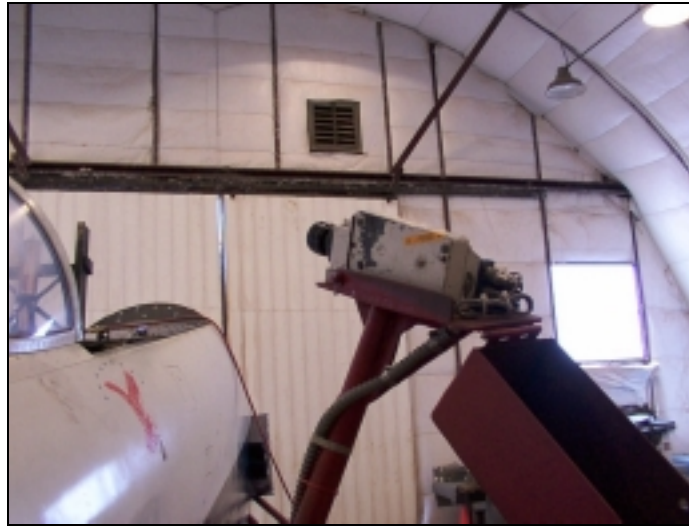
Figure 29. 16mm High-speed Sled Camera
