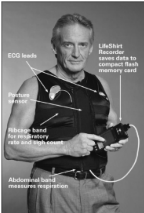
Figure B-3. LifeShirt® sensor vest and wired data recorder [61]
