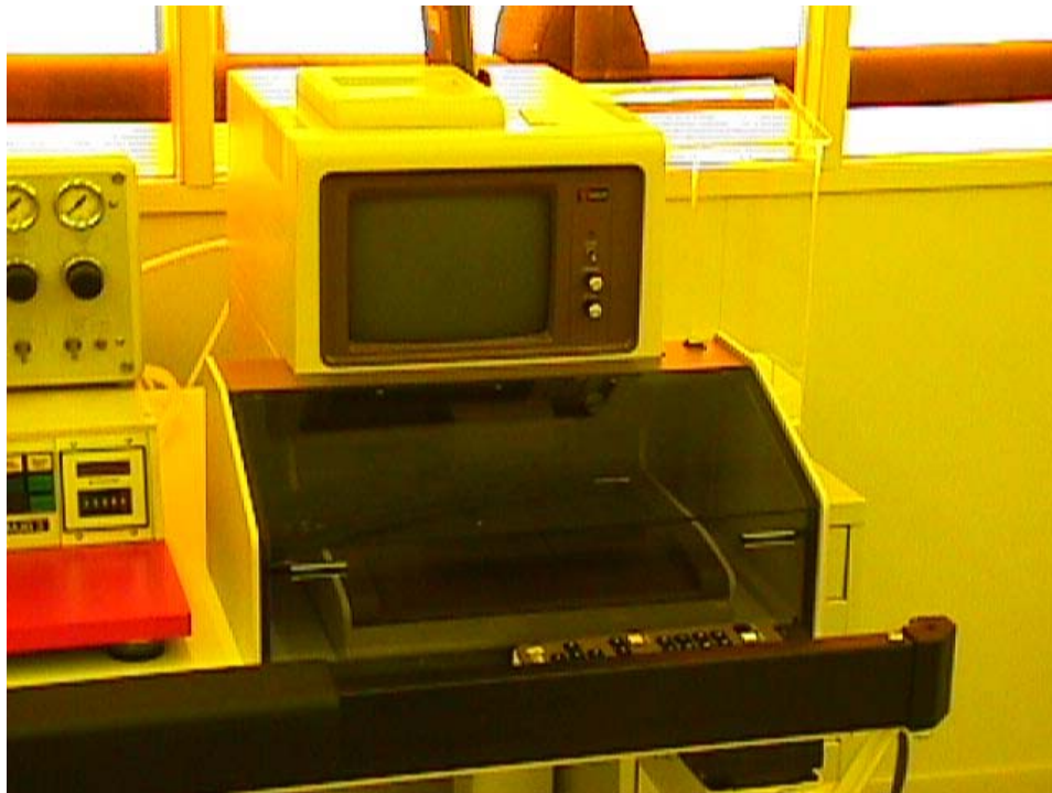
Figure 46 Tencor Alpha Step 200 Profilometer located in the AFIT cleanroom.
