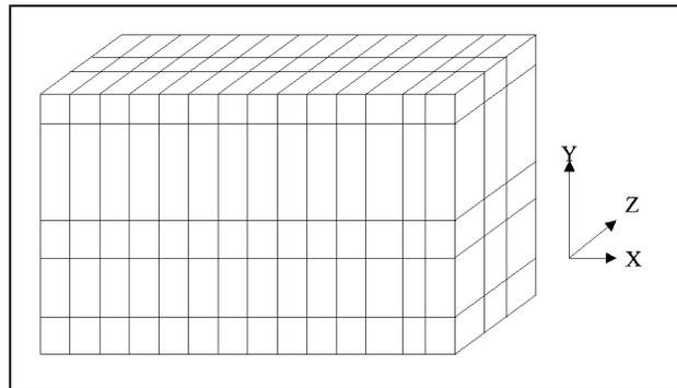
**Figure 2.9: Finite difference grid used in MODFLOW (Garrett, 1999)**
