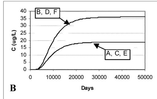
**Figure 4.8: Concentration breakthroughs in the 6<sup>th</sup> layer for changing system anisotropy (a) monitoring well 1 and (b) monitoring well 2**
