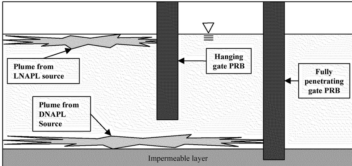
**Figure 2.3: Fully penetrating and hanging gate PRB configurations**
