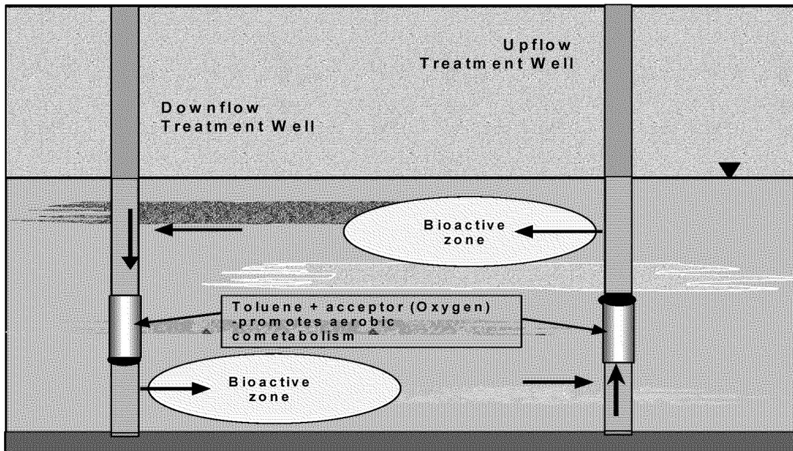
Figure 2.5: Schematic of HFTW system with bioactive zones
