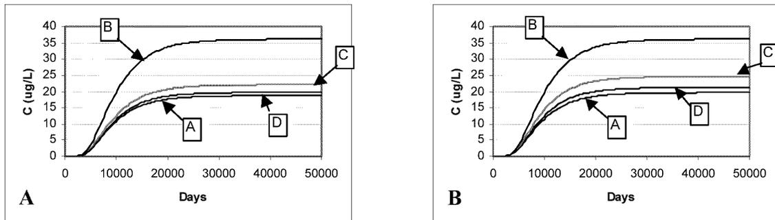
**Figure 4.13: Concentration breakthroughs in the 8<sup>th</sup> layer for changing pump rates (a) monitoring well 1 and (b) monitoring well 2**
