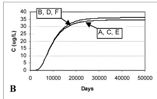
**Figure 4.9: Concentration breakthroughs in the 7<sup>th</sup> layer for changing system anisotropy (a) monitoring well 1 and (b) monitoring well 2**
