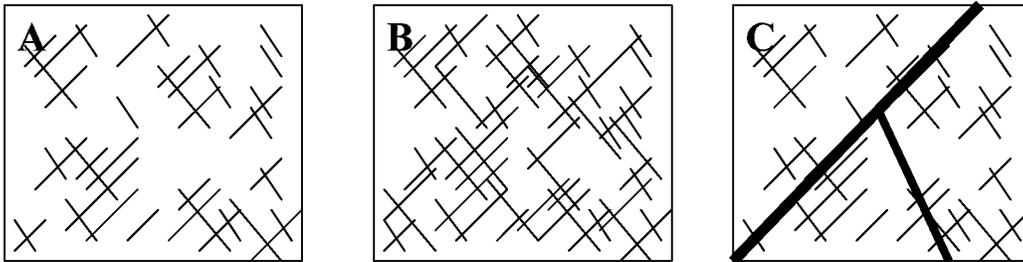
**Figure 2.10: Porosity differences in fractured media. (a) Unconnected fractures with minimal flow, (b) connected clusters that would support fractured flow, and (c) large fractures dominating the matrix inducing channel flow (From Domenico and Schwartz, 1998)**
