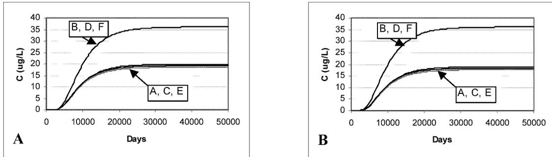
**Figure 4.2: Concentration breakthroughs in the 6<sup>th</sup> layer for varying 7<sup>th</sup> layer conductivity (a) monitoring well 1 and (b) monitoring well 2**
