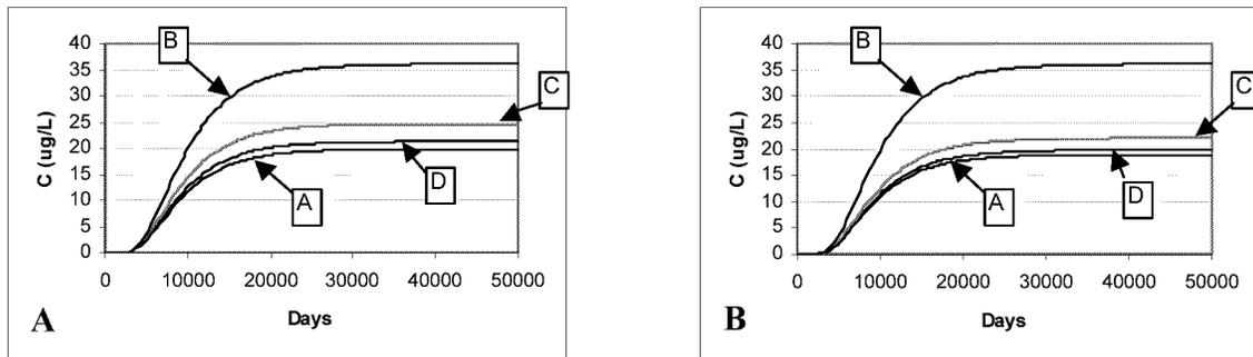
**Figure 4.11: Concentration breakthroughs in the 6<sup>th</sup> layer for changing pump rates (a) monitoring well 1 and (b) monitoring well 2**
