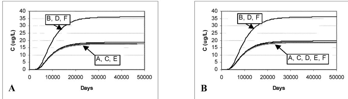
**Figure 4.4: Concentration breakthroughs in the 8<sup>th</sup> layer for varying 7<sup>th</sup> layer conductivity (a) monitoring well 1 and (b) monitoring well 2**
