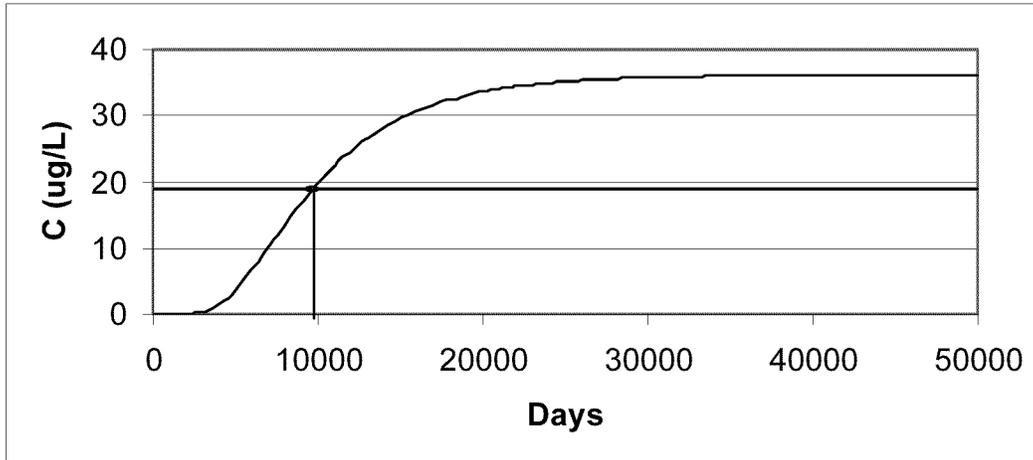
**Figure 4.1: Breakthrough curve at layer 6 of monitoring well 1 for contaminant transport by regional gradient only (HFTWs not pumping). Transport time to the well is estimated as the time to attain 50% of the steady-state concentration at the well.**
