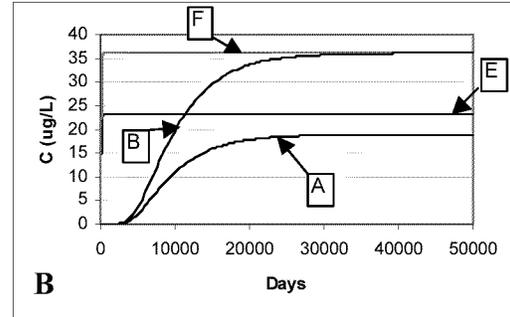
**Figure 4.5: Concentration breakthroughs in the 6<sup>th</sup> layer for varying gneiss conductivity (a) monitoring well 1 and (b) monitoring well 2**
