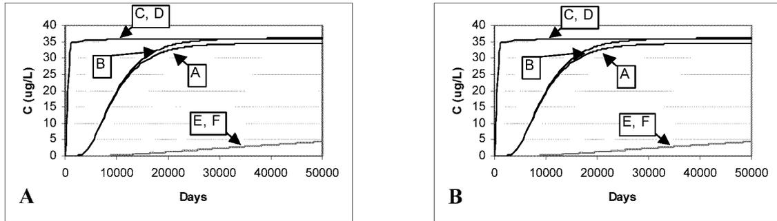
**Figure 4.3: Concentration breakthroughs in the 7<sup>th</sup> layer for varying 7<sup>th</sup> layer conductivity (a) monitoring well 1 and (b) monitoring well 2**
