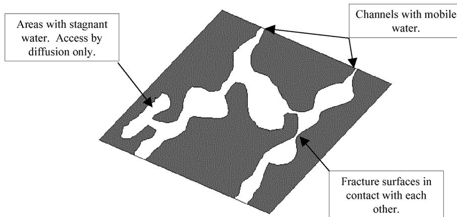
**Figure 2.13: Channel network conceptual model (Selroos *et al.*, 2001)**
