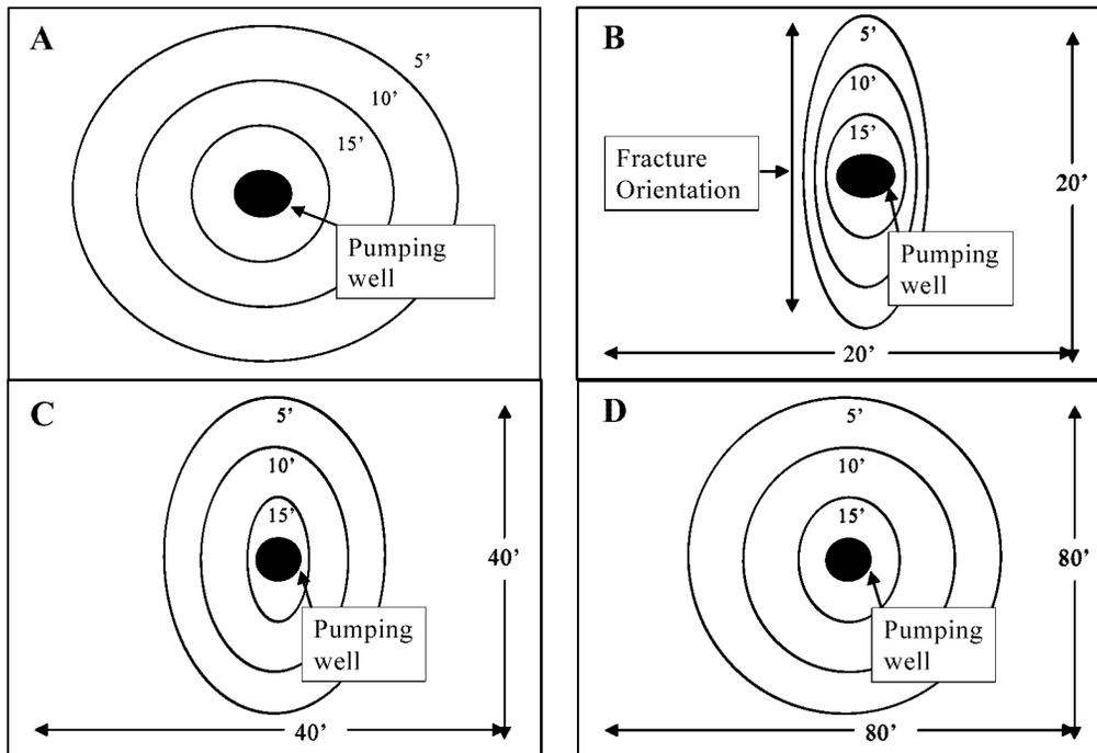
**Figure 2.12: Drawdown curves differ for porous media versus fractured media, but begin to converge as measurements are taken farther from the pumping well: (a) drawdown expected from homogenous porous media, (b) drawdown due to fractal flow at small radial distance, (c) and (d) as the radial distance from the pumping well increases, the drawdown begins to resemble that of porous media.**
