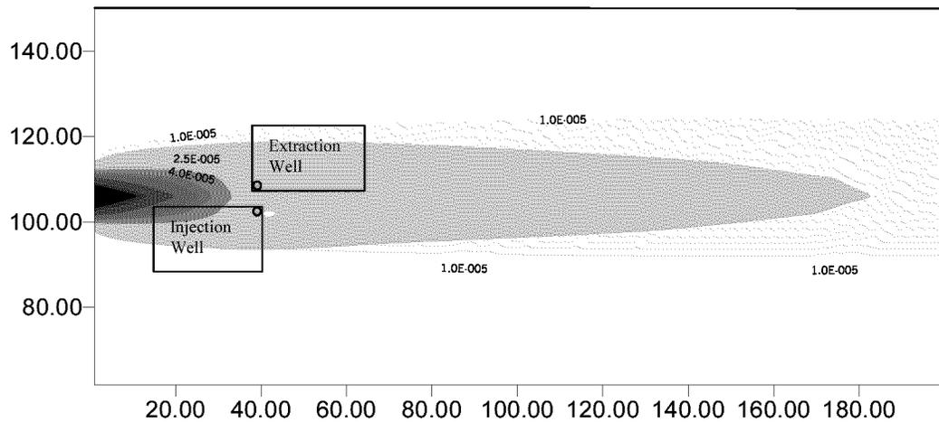
**Figure 4.14: Concentration contours ( $\text{mg}/\text{m}^3$ ) in layer 6 at 50,000 days. Note that the contaminant plume bypasses the capture zone of the HFTW system, and is transported downgradient**
