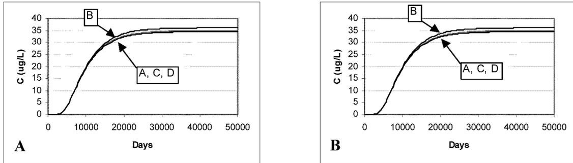
**Figure 4.12: Concentration breakthroughs in the 7<sup>th</sup> layer for changing pump rates (a) monitoring well 1 and (b) monitoring well 2**
