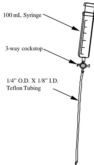
**Figure 4. Extraction Assembly**
