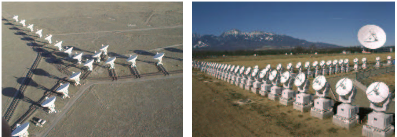
Figure 3.2 The Very Large Array (left) near Socorro, New Mexico has its 27 antennas mounted on rails for limited repositioning capability to 72 different antenna stations. The Nobeyama Solar Radio Observatory (right) in Nobeyama, Japan has its 84 antennas permanently spaced for optimum observations of the solar disk.
