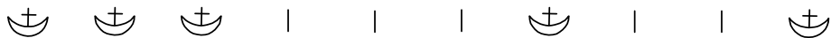
Figure 3.10 This five antenna array suggested by Bracewell only has redundancy in the unit spacing.
