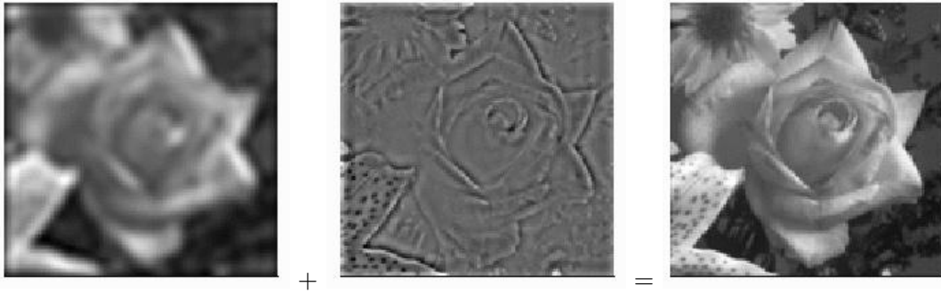
Figure 3.9 The overall image quality is a composite of the regional intensities offered by low spatial frequencies and the edge-defining properties of the high spatial frequencies.
