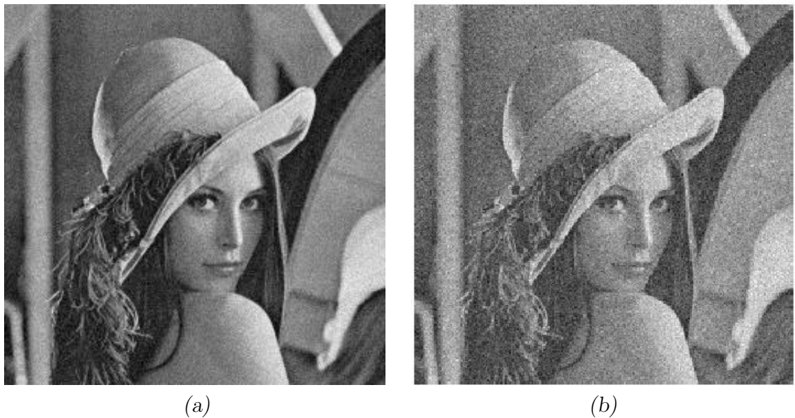
Figure 4.2. Examples of PSNR values for the test images. (a) Lenna image with 28 dB PSNR. (b) Lenna image with 22 dB PSNR.
