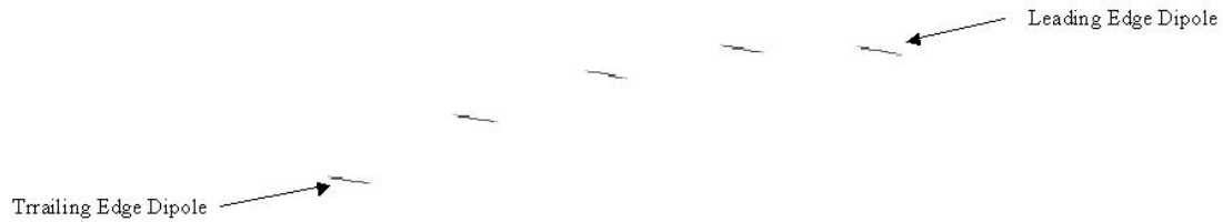
Figure 1.2 One chordwise array of dipoles
