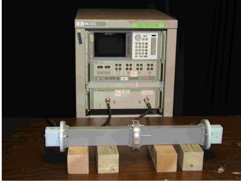
Figure 4-1. Experimental setup showing a WR284 waveguide connected to an HP8510C Vector Network Analyzer with coaxial cables. The reduced-aperture sample holder is mounted between the waveguide feeds with precision alignment pins.
