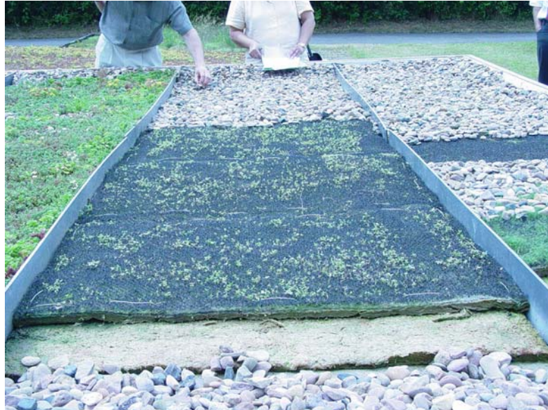
Figure 2.6 Soil-less plants. Xeroflor's seed-impregnated mats. Plastic mesh covers seed impregnated mats; pebbles cover others; pre-grown mats grow without soil as well.
