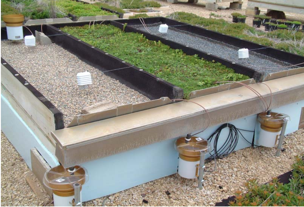
Figure 4.38 Divided Test Platform. A divided model-scale platform used to quantify differences in storm water runoff between roof types. (VanWoert et al., 2003)
