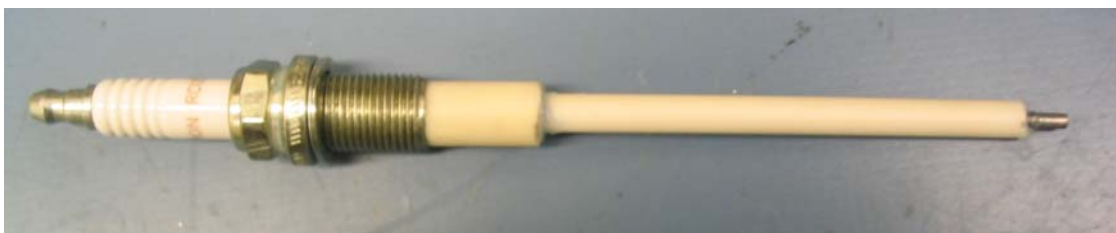
Figure 6. Long Probe with 10.16 cm insulated extension
