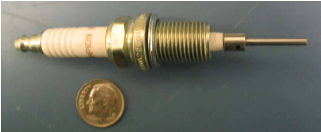
Figure 5. Medium Probe with 2.54 cm center electrode
