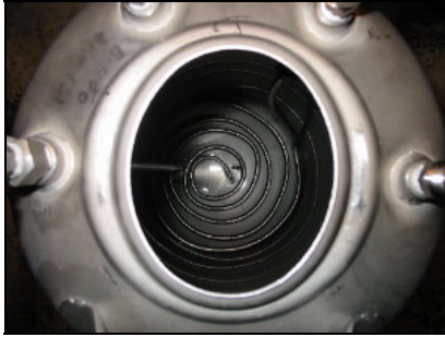
Fig. 3.17 Sparging coil in fuel tank
