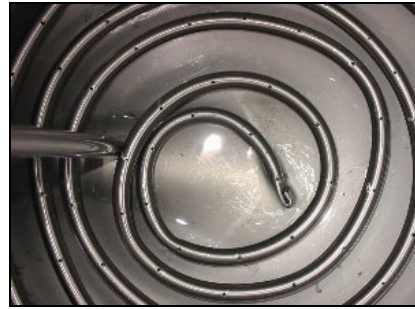
Fig. 3.18 Sparging coil close-up
