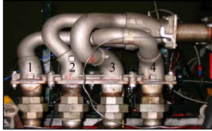
Fig. 3.11 Manifold that feeds fuel-air mixture into four thrust tube heads
