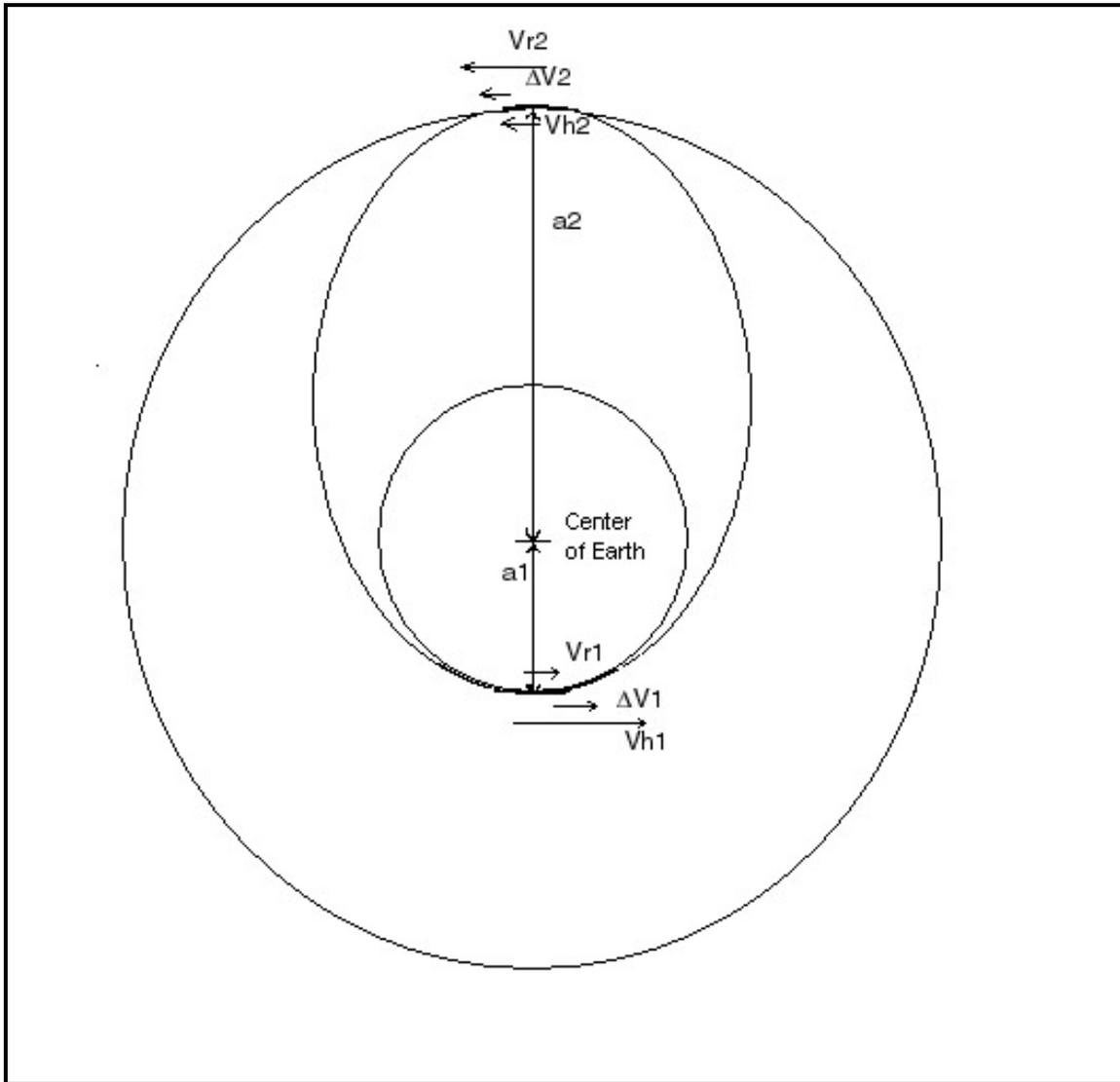
Figure 4: Hohmann Transfer between two orbits (Wiesel, 1989:74)
