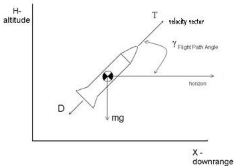
**Figure 3: Diagram of Forces Acting on the Vehicle**
