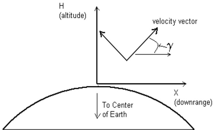
**Figure 2: Reference frame with flight path angle**
