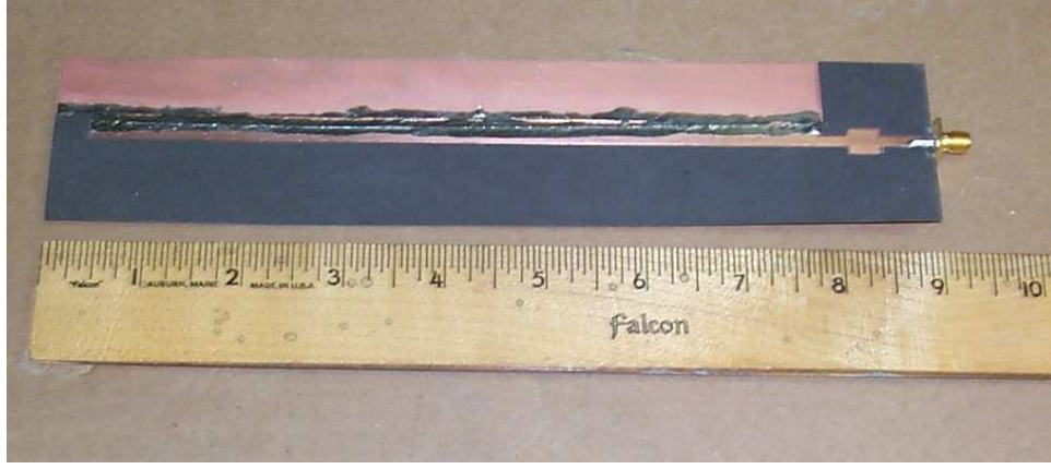
Figure 5.16: THW antenna fabricated without vias.
