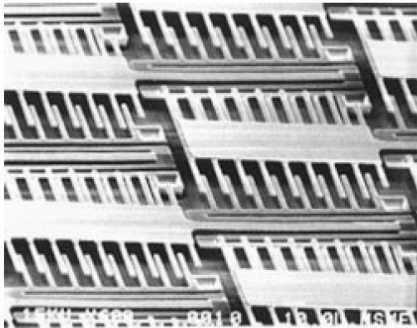
Figure 8. SEM of pixels using optical gratings controlled by thermally generating stress in SiN cantilever arms [34].
