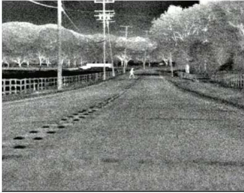
Figure 9. IR image taken with thin-film ferroelectric pixel array camera with f/1 optics [36].
