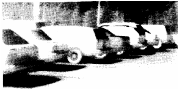
Figure 10. IR image obtained using monolithic silicon 240 x 336 FPA operating at room temperature with camera f/1 optics and 30 Hz frame rate [37].
