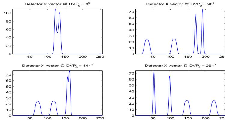
Figure 4.18: This figure shows the  $x$  vector sum of the detector image for the small overlapping bar test hyperspectral data cube. The vector again shows the spatial separation of the dispersed bars.
