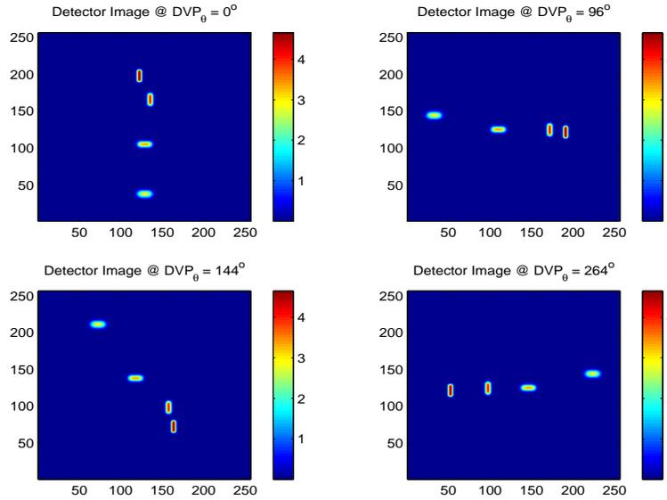
Figure 4.17: This figure shows the detector at four rotation angles resulting from the CTIS model sensing the  $20 \times 20$  pixel bar test hyperspectral data cube. Again the spectrally dispersed bars are spatially separated with the smaller scene image.
