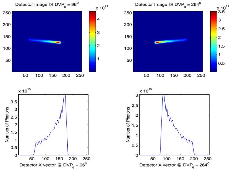
Figure 4.37: This figure shows the CTIS detector image and  $x$  vector sum of the second evolving fireball. This fireball transitions from  $1600^\circ\text{K}$  to  $1300^\circ\text{K}$  at  $DVP_\theta = 168^\circ$ .
