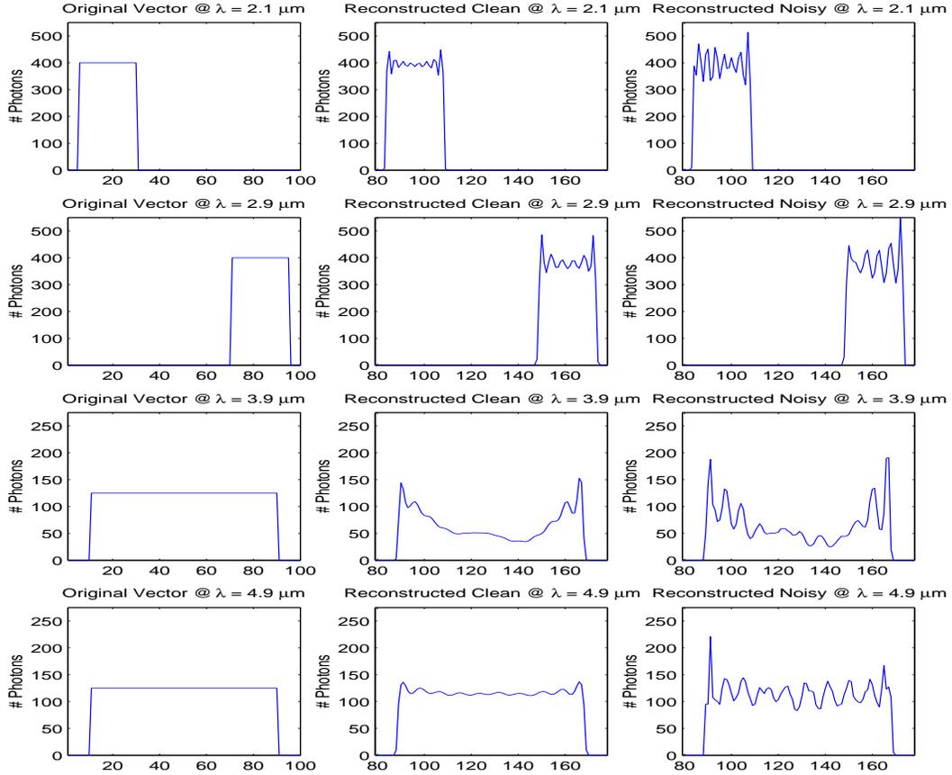
Figure 5.18: This figure shows the reproduction of the original overlapping bar test data cube by the 1D reconstruction algorithm. Again the reconstruction of  $x$  vector sum degrades with the addition of noise to the detector image.
