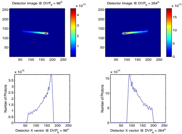
Figure 4.36: This figure shows the CTIS detector image and  $x$  vector sum of the first evolving fireball. This fireball transitions from  $1600^\circ\text{K}$  to  $1500^\circ\text{K}$  at  $DVP_\theta = 168^\circ$ .
