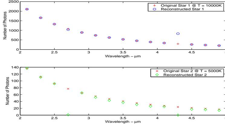
Figure 5.7: This figure shows the original and reconstructed  $x$  vector containing a horizontal sum of the number of photons in the input hyperspectral data cube. The results are obtained using 1000 iterations of the vector atmospheric reconstruction algorithm.
