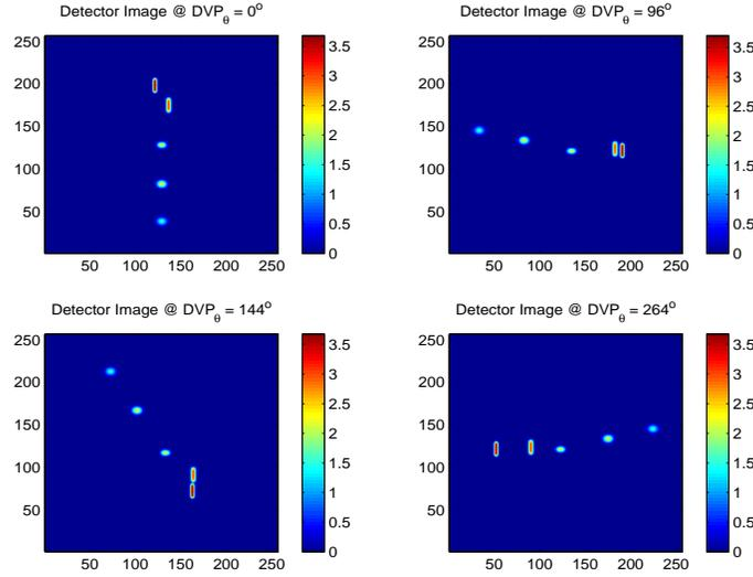
Figure 4.10: This figure shows the detector at four rotation angles resulting from the CTIS model sensing the  $20 \times 20$  pixel bar test hyperspectral data cube. The major difference (apart from bar size) compared to Figure 4.8 is that the spectrally dispersed bars are spatially separated. Note also how the expected bar-shape changes. This is a function of the PSF of the optics in that PSF width increases with wavelength.
