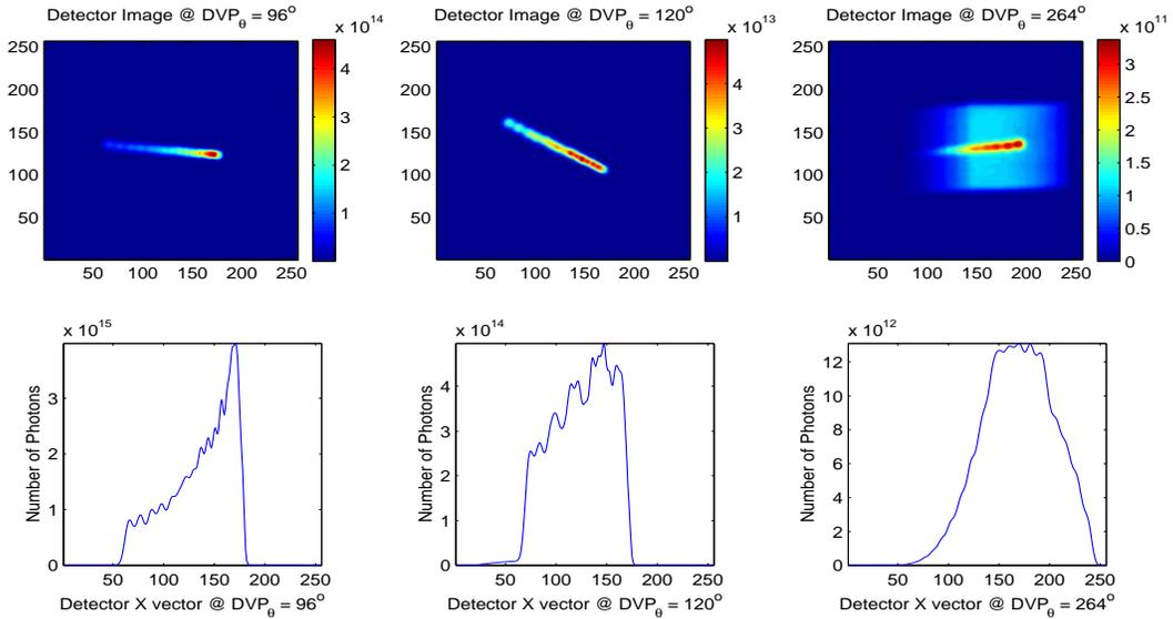
Figure 4.39: This figure shows the CTIS detector image and  $x$  vector sum of the fourth evolving fireball. This fireball transitions from  $1600^\circ\text{K}$  to  $1000^\circ\text{K}$  at  $DVP_\theta = 120^\circ$  and  $1000^\circ\text{K}$  to  $400^\circ\text{K}$  at  $DVP_\theta = 240^\circ$ .
