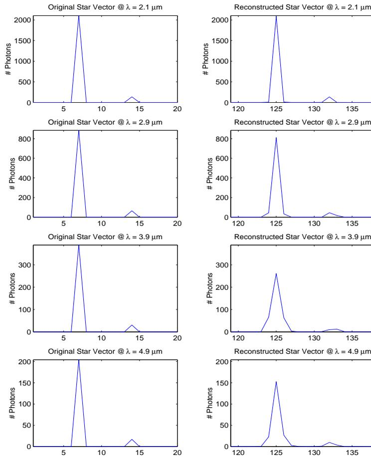
Figure 5.5: This figure shows the original and reconstructed  $x$  vector containing a horizontal sum of the number of photons in the input hyperspectral data cube. The results are obtained using the 1000 iterations of the vector reconstruction algorithm.
