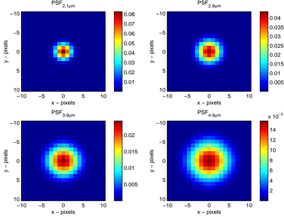
Figure 3.6: This figure shows the different unshifted spectral  $PSF_\lambda$  for  $\lambda = 2, 2.9, 3.9$  and  $4.9\mu m$ . Each unshifted spectral  $PSF_\lambda$  sums to one over the  $21 \times 21$  matrix.
