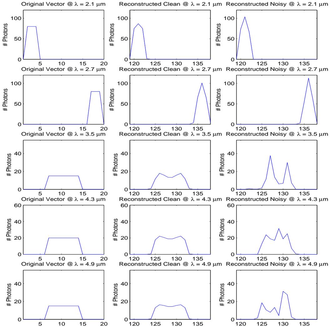
Figure 5.13: This figure shows the reproduction of the original small bar test data cube by the 1D reconstruction algorithm. The reconstruction of  $x$  vector sum suffers more degradation than the previous test case with the addition of noise to the detector image.
