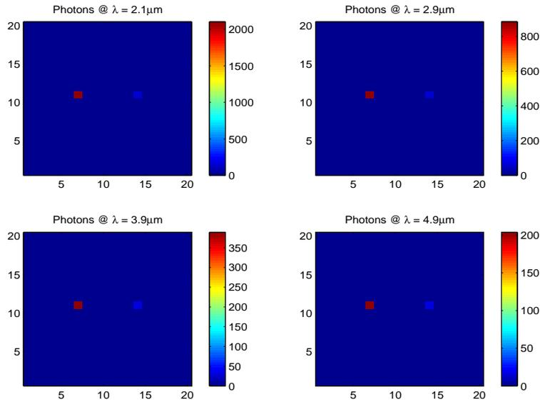
Figure 4.1: This figure shows four wavelength bins of the binary star hyperspectral data cube. The cube has spatial extent of  $20 \times 20$  pixels with the stars being separated by six pixels. The number of photons in each bin is indicated by the color bar.
