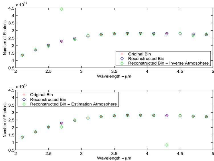
Figure 5.29: This figure shows the sum of photons in each wavelength bin for the  $1000^\circ\text{K}$  fireball in the reconstructed data compared with the original data cube. The sum of photons for the reconstruction of atmospherically attenuated detector data is also shown for both atmospheric reconstruction methods.
