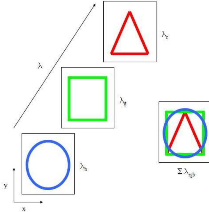
Figure 1.1: This figure shows three monochromatic images (red, green and blue) within a multi-spectral data cube. The data cube is composed of two spatial dimensions,  $x$  and  $y$ , and one spectral dimension,  $\lambda$ . The sum of the images along the spectral dimension of the data cube results in a broadband image of the red, green and blue wavelengths.
