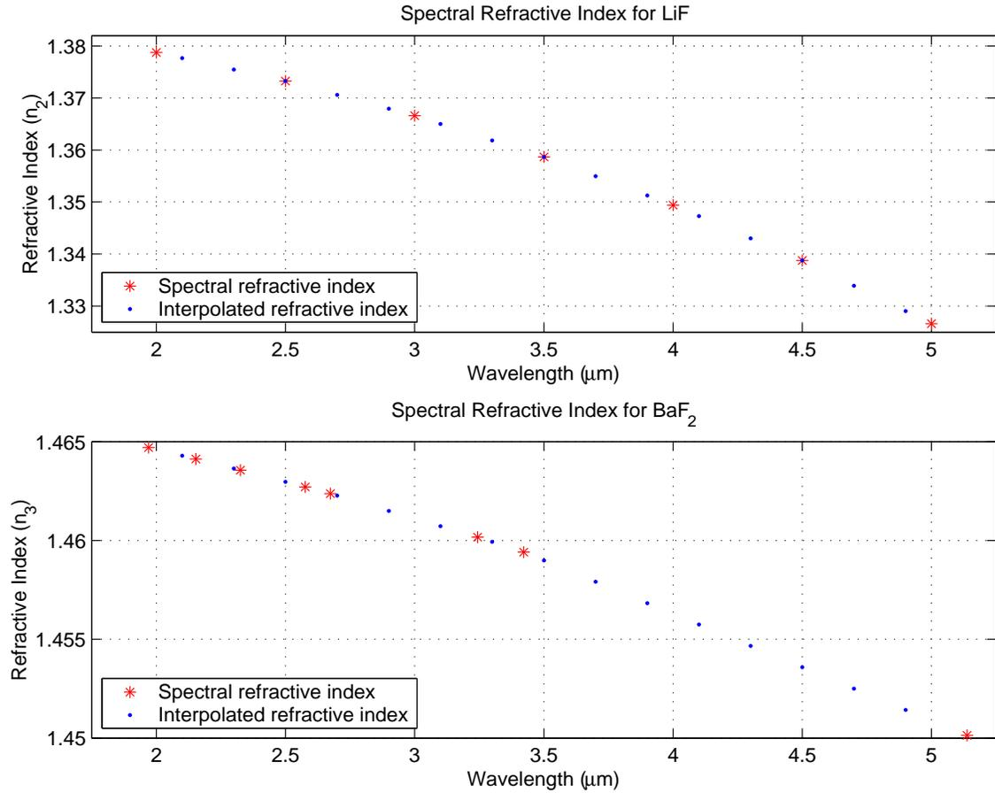
Figure 3.1: This figure shows the linear interpolation of the spectral refractive indices for both LiF and BaF<sub>2</sub> at the center of each wavelength bin.
