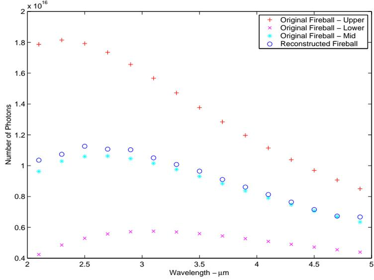
Figure 5.45: This figure shows the sum of photons in each wavelength bin for the third evolving fireball. The reconstruction algorithm averages the three components of the original input data cube.
