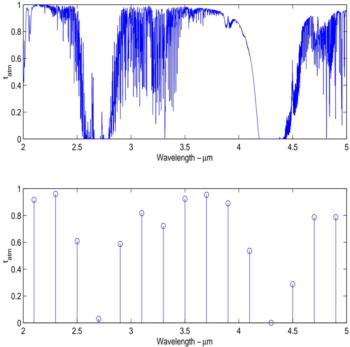
Figure 3.10: This figure shows the wavelength dependent atmospheric transmission coefficient,  $t_{atm}(\lambda)$ , with the pseudo-continuous data in the upper subplot taken from [14]. This data is then sampled by averaging over each wavelength bin as shown in the lower subplot.
