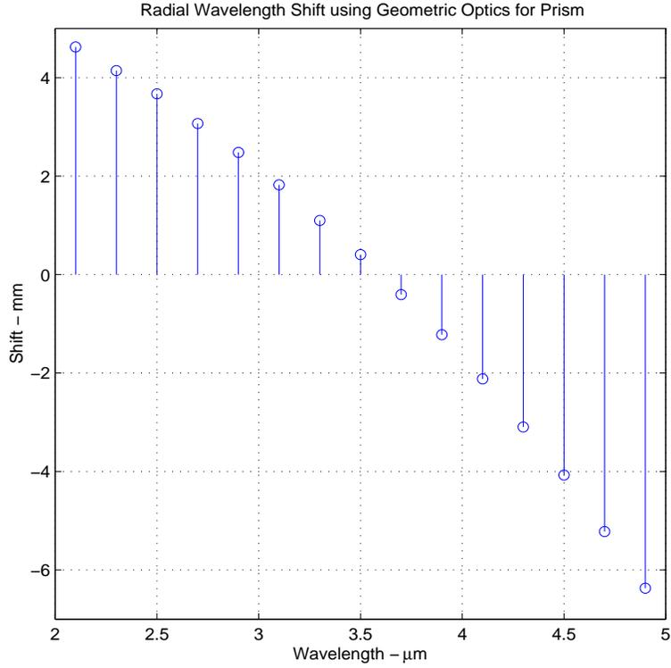
Figure 3.3: This figure shows the radial spectral shifts ( $r_\lambda$ ) at the detector resulting from the Direct Vision Prism and Focusing Lens for 15 spectral bins. Note that  $\lambda = 3.6\mu\text{m}$  is the undeviated wavelength and that the separation between consecutive shifts increases as wavelength increases.
