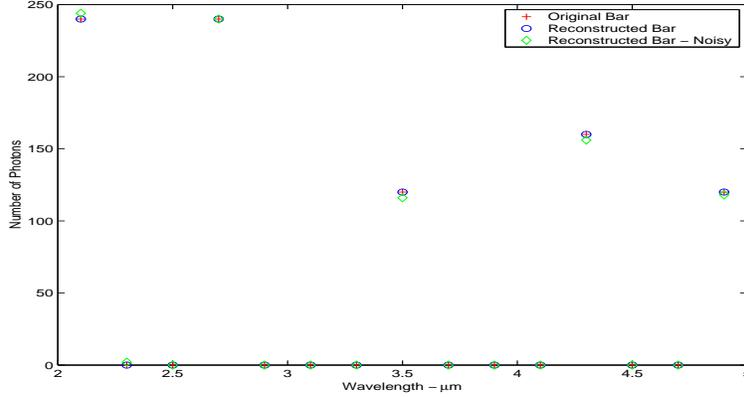
Figure 5.14: This figure shows the sum of photons in each wavelength bin for the smaller bar test in the reconstructed data compared with the original data cube. The sum of photons for the reconstruction of noisy detector data is also shown. The smaller input data cube leads to improved reconstruction performance in terms of reproducing the number of photons in the original scene.
