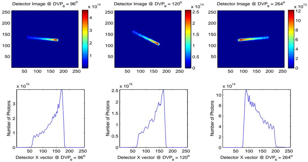
Figure 4.38: This figure shows the CTIS detector image and  $x$  vector sum of the third evolving fireball. This fireball transitions from  $1600^\circ\text{K}$  to  $1400^\circ\text{K}$  at  $DVP_\theta = 120^\circ$  and  $1400^\circ\text{K}$  to  $1200^\circ\text{K}$  at  $DVP_\theta = 240^\circ$ .
