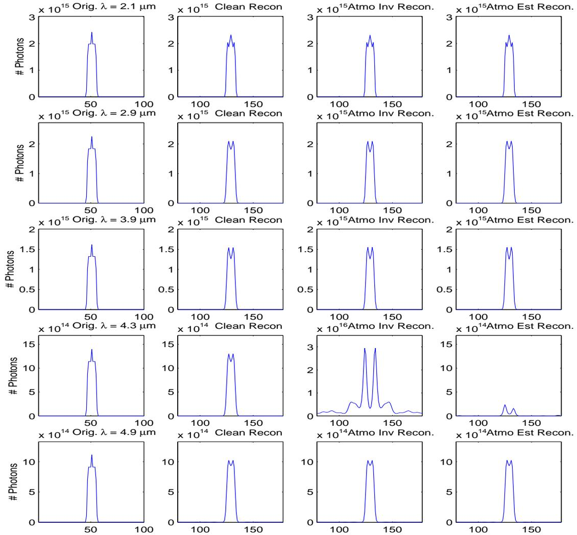
Figure 5.30: This figure shows the reproduction of the original 1600°K fireball data cube by the vector reconstruction algorithm. The reconstruction of atmospherically attenuated input data is also shown with reconstruction failure in the  $\lambda = 4.3\mu\text{m}$  bin for both atmospheric reconstruction methods.
