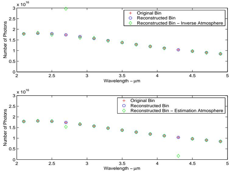
Figure 5.31: This figure shows the sum of photons in each wavelength bin for the  $1600^{\circ}\text{K}$  fireball in the reconstructed data compared with the original data cube. The sum of photons for the reconstruction of atmospherically attenuated detector data is also shown.
