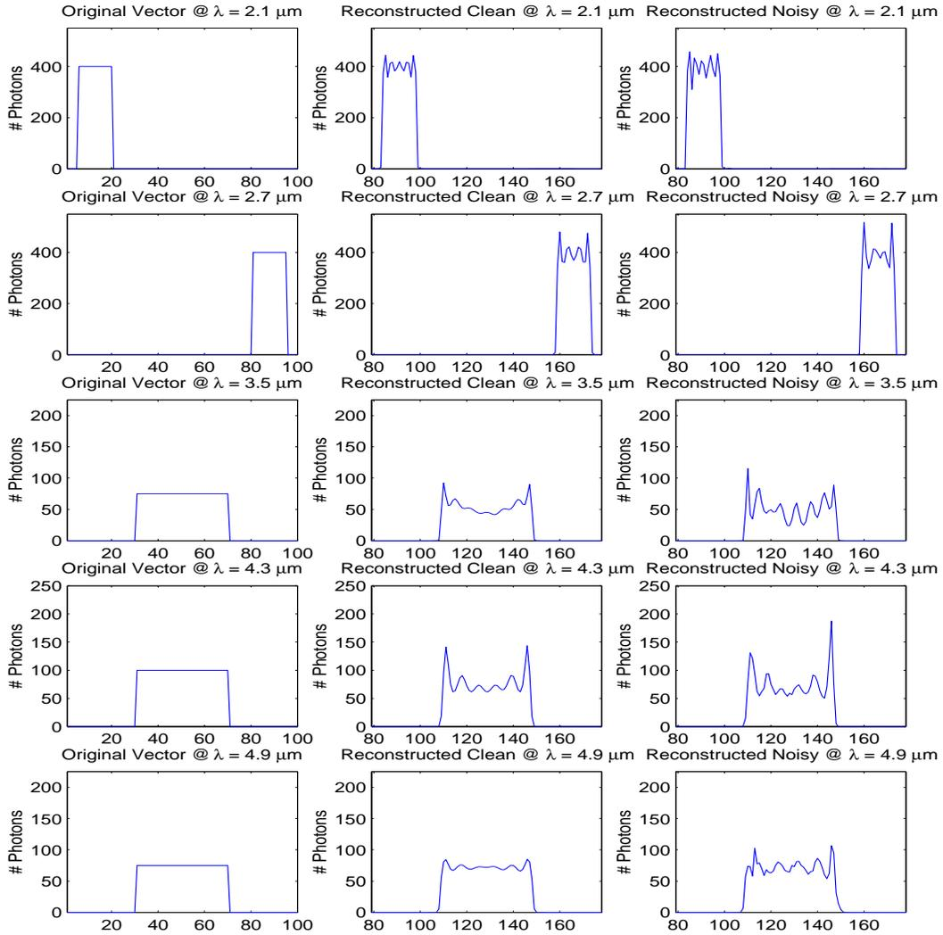
Figure 5.11: This figure shows the reproduction of the original bar test data cube by the 1D reconstruction algorithm. The reconstruction of  $x$  vector sum degrades with the addition of noise to the detector image, though the general spatial features are still apparent.
