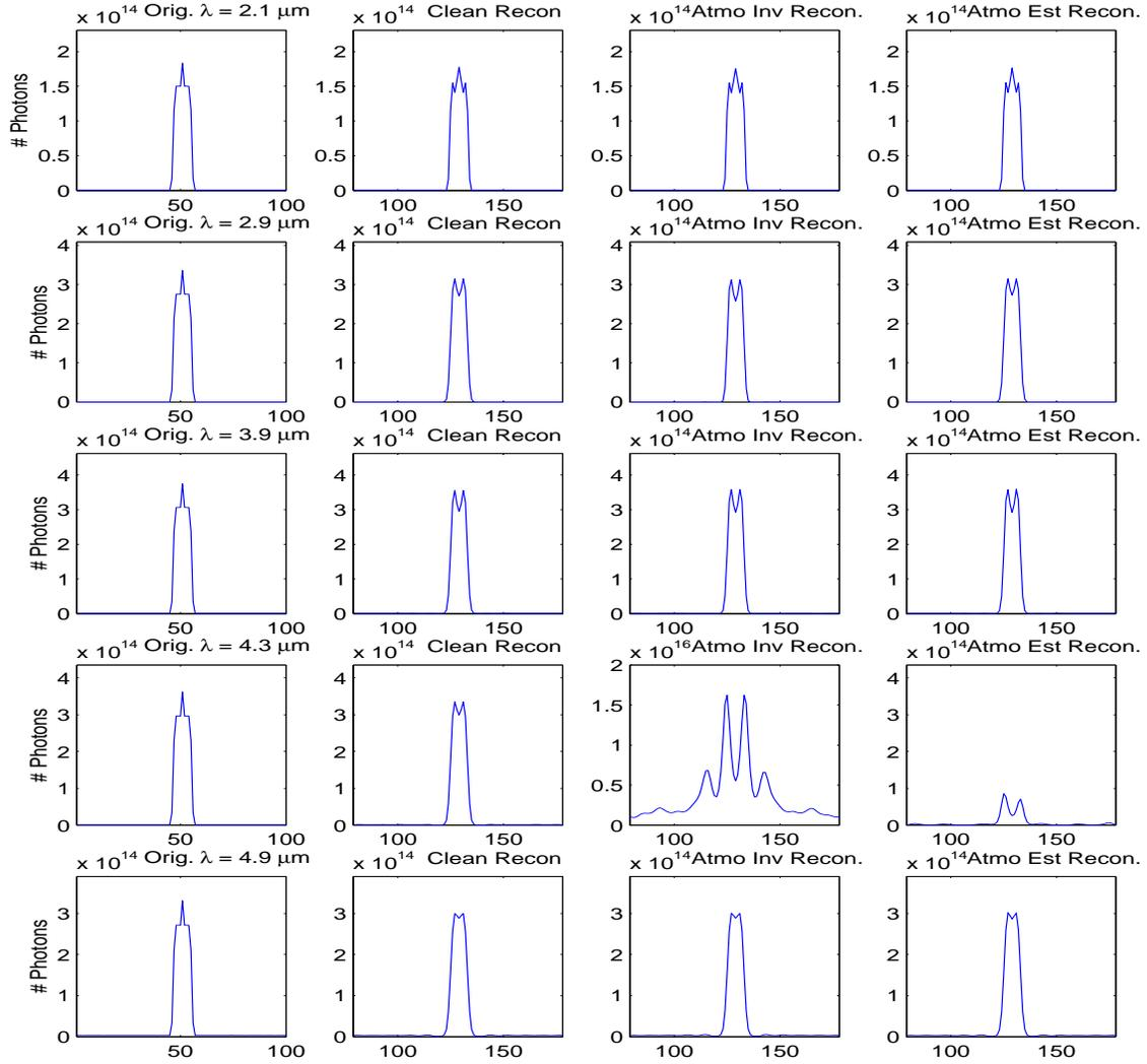
Figure 5.28: This figure shows the reproduction of the original 1000°K fireball data cube by the vector reconstruction algorithm. The reconstruction of atmospherically attenuated input data is also shown with reconstruction failure in the  $\lambda = 4.3 \mu\text{m}$  bin more severe in the direct atmospheric inverse method.
