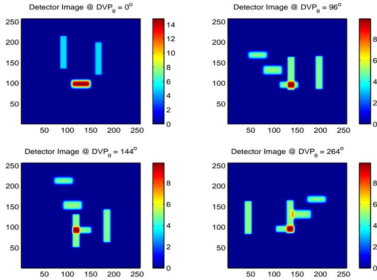
Figure 4.8: This figure shows the detector image at four rotation angles resulting from the CTIS model sensing the  $100 \times 100$  pixel bar test hyperspectral data cube. The CTIS model spatially disperses the sources as a function of wavelength and DVP rotation angle.
