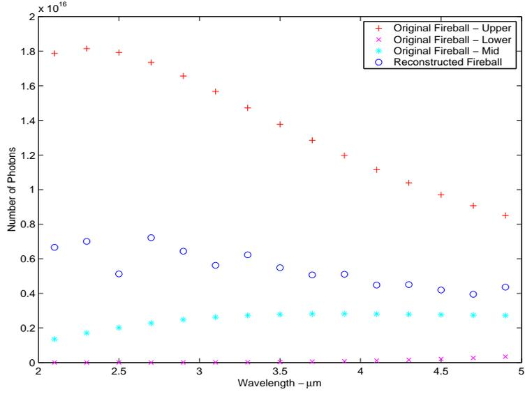
Figure 5.47: This figure shows the sum of photons in each wavelength bin for the fourth evolving fireball. The reconstruction algorithm averages the three components of the original input data cube with a greater error than in the previous test case.
