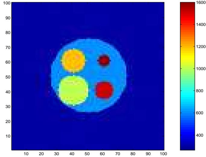
Figure 4.33: This figure shows a temperature map of a  $600^{\circ}\text{K}$  fireball containing hot-spots at a temperature of  $1000^{\circ}\text{K}$ ,  $1200^{\circ}\text{K}$ ,  $1500^{\circ}\text{K}$  and  $1600^{\circ}\text{K}$ . The random background scene has a mean temperature of  $300^{\circ}\text{K}$ .
