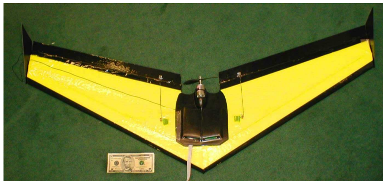
Figure 1.1: A inexpensively constructed UAV used by Carnegie Mellon University for teaching students control theory, artificial intelligence, and robotics.
