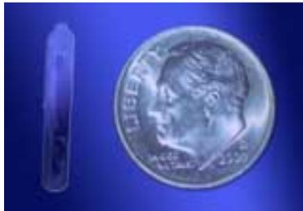
**Figure 1: An Implantable RFID Tag (VeriChip Corporation, 2004)**
