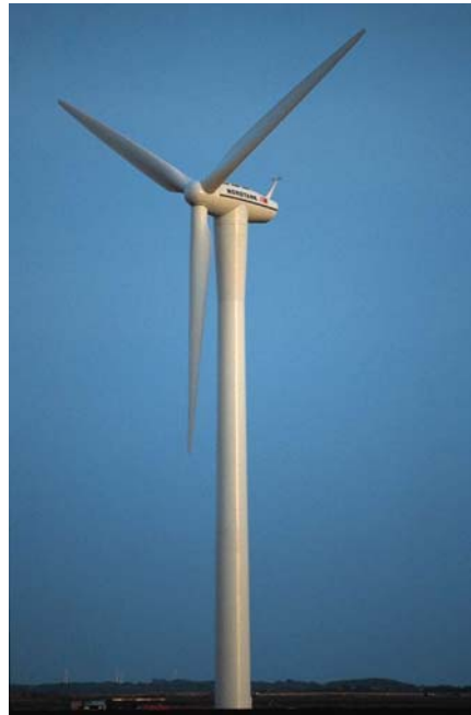
Figure 7. A Horizontal-Axis Three-Bladed Turbine
