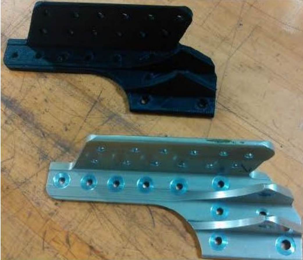
Figure 2. 10 Additive Printed Part [46].
