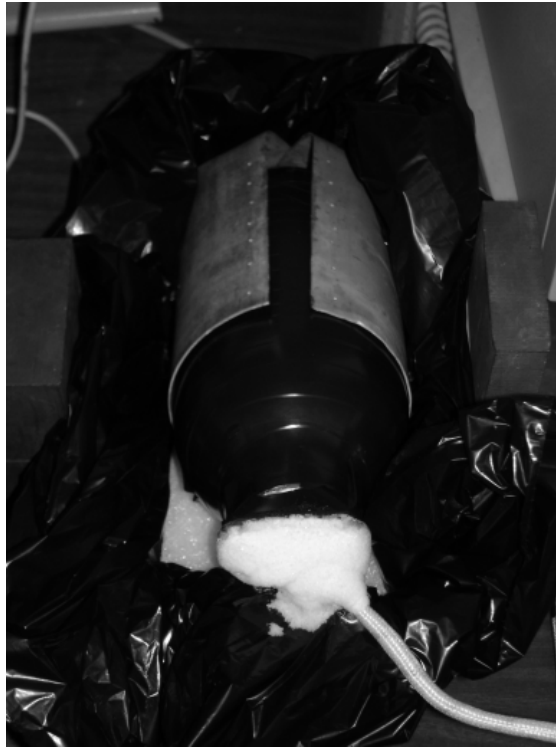
Figure 38. 6" Dewar system for in situ measurements at 80 K within the BP.
