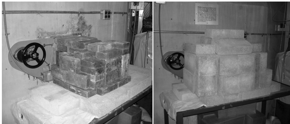
Figure 41. Shielding of the beam port with lead bricks (LEFT) and concrete blocks (RIGHT) to attenuate neutron-induced gamma radiation.
