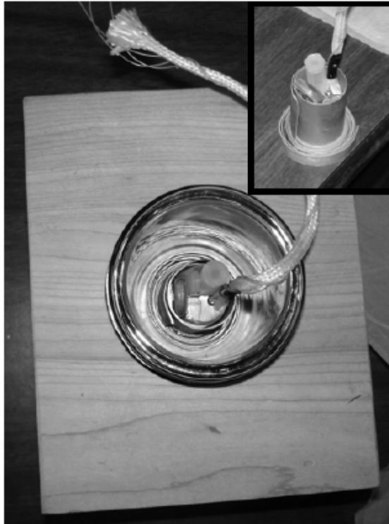
Figure 36. Dewar shown in wooden cradle designed to fit within the 7" section of the beam port. Inset shows Cadmium shielded thermal block.
