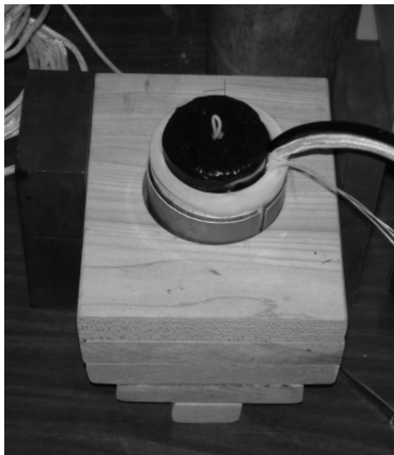
Figure 37. Wooden cradle used for both in situ beam port measurements and benchtop characterizations at 80 K in darkness.
