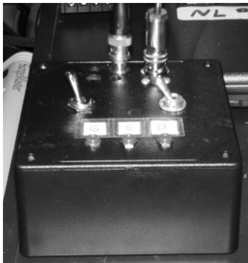
Figure 34. Measurement-type control switch.
