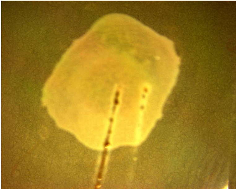
Figure 20. 0.50 and 0.35 W Laser Burn Lines through Spore Sample
