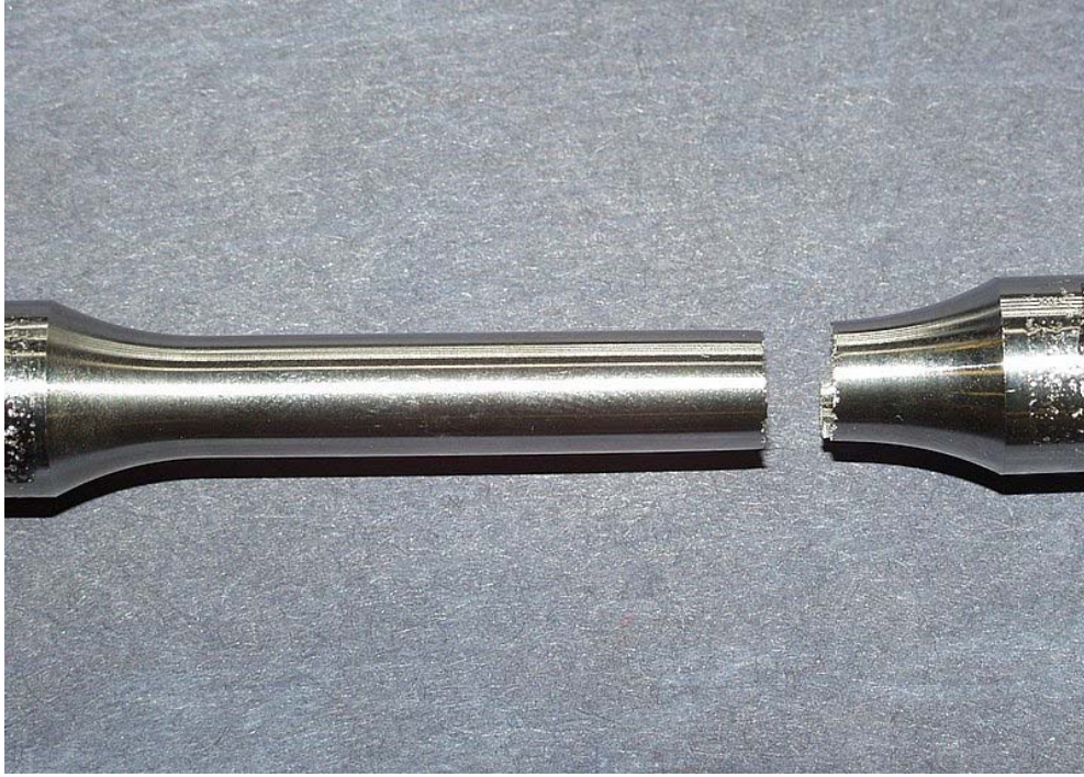
Figure 3-59. Tensile Test Failure
