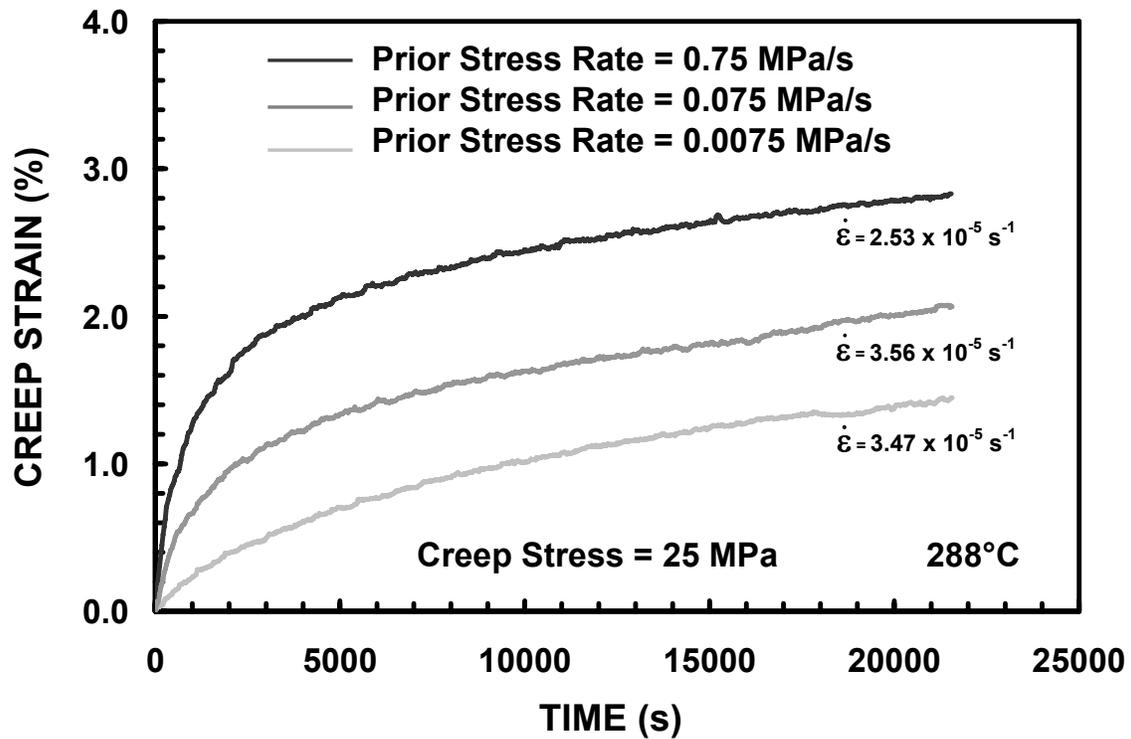
Fig. 15. Creep strain vs. time at 25 MPa and 288°C. Effect of prior stress rate on creep strain is apparent
