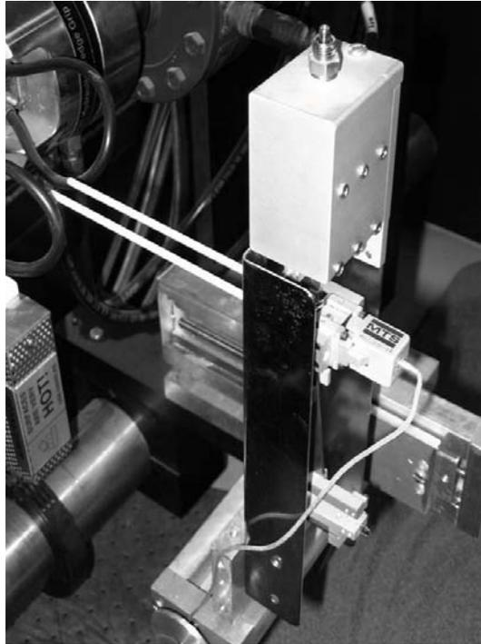
Figure 6. High temperature extensometer assembly
