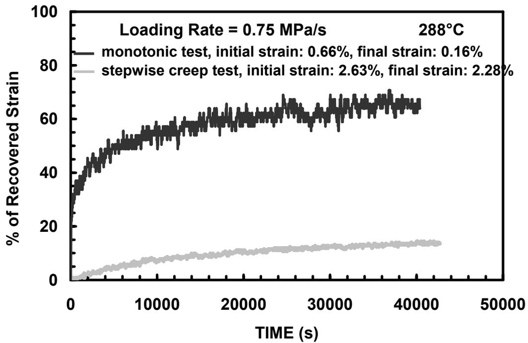
Figure 32. Recovery following monotonic loading and unloading test and recovery following stepwise creep test with prior stress rate of 0.75 MPa/s at 288°C. Recovery is calculated as the percent of the strain at the beginning of recovery.
