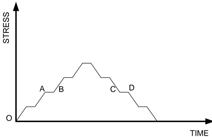
Figure 7. Schematic of stepwise creep test
