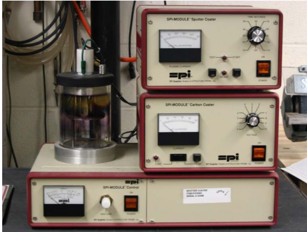
Figure 21. SPI MODULE Sputter Coater
