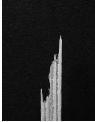
Figure 32. Tensile Fracture Surface of N610/Alumina at 1100°C (Side)
