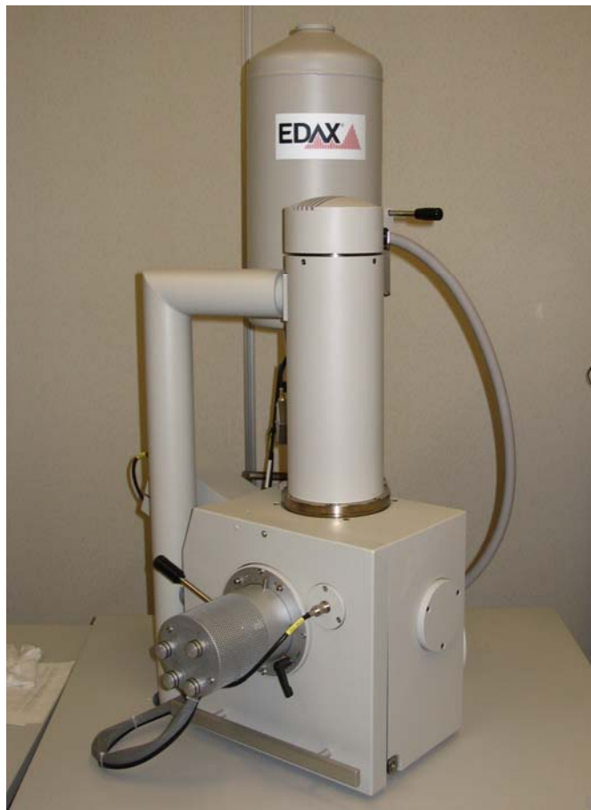
Figure 20. FEI Quanta 200 HV Scanning Electron Microscope
