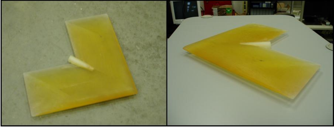
Figure 10: \frac{1}{2} -Scaled Chevron UCAV Model
