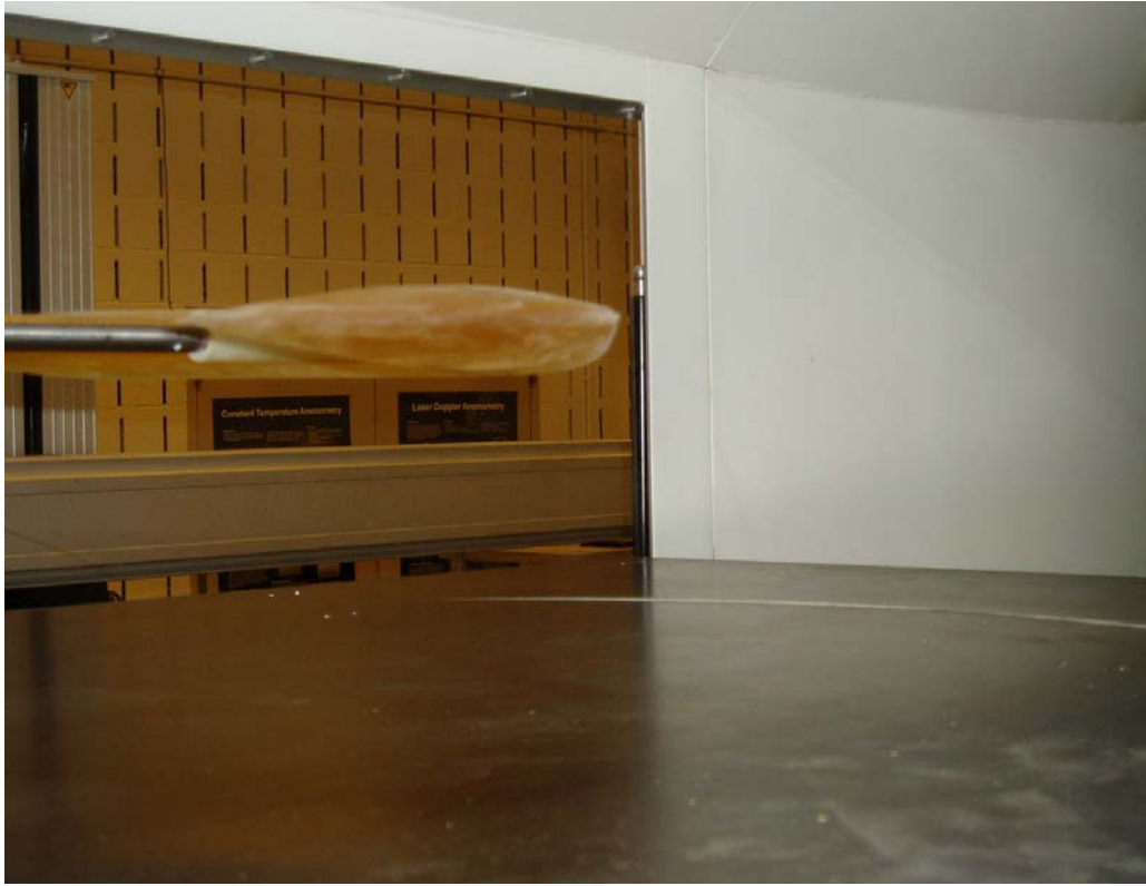
Figure 46: Model & Ground Plane at h/b = 0.3
