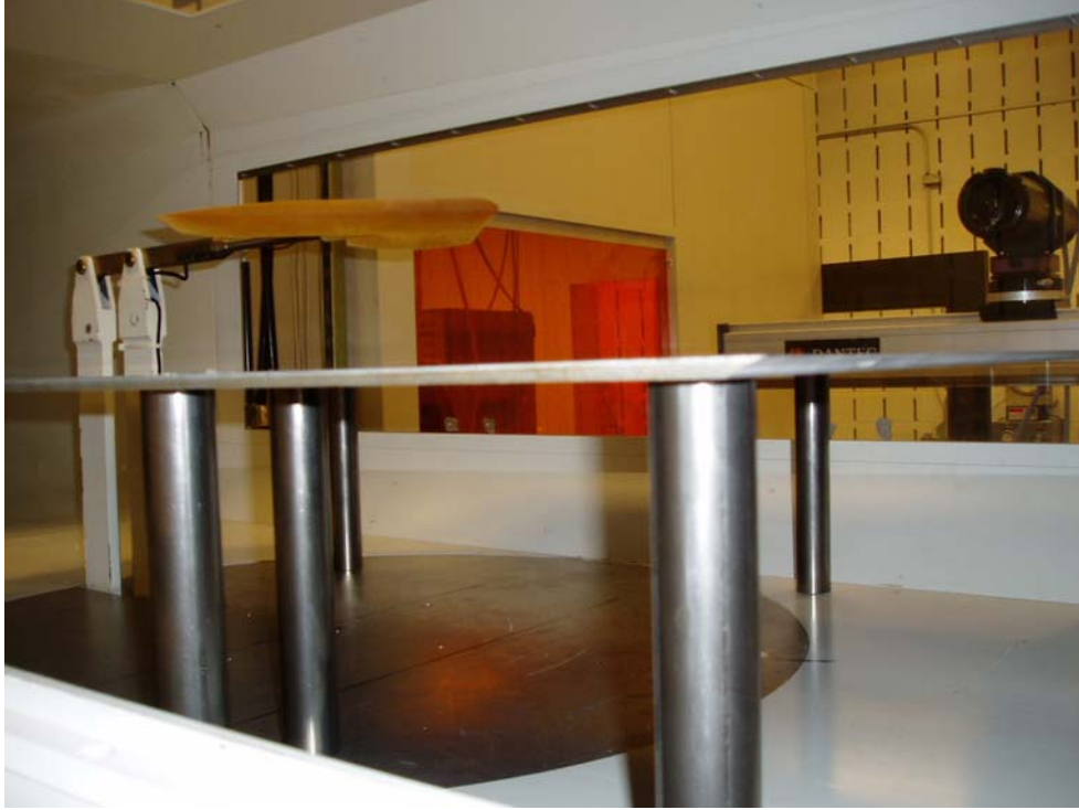
Figure 17: Ground Plane and Model in Test Section
