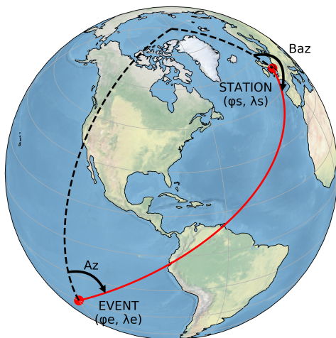
Figure 30. This diagram demonstrates the azimuth ( Az ) and backazimuth ( Baz ) angles for the given Event-Station pair. The latitude and longitude coordinates for the station, in radians, are given by (\phi_s, \lambda_s) , while the event coordinates are given by (\phi_e, \lambda_e) .
